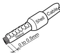
Figure 5.15 Using a bar terminal
