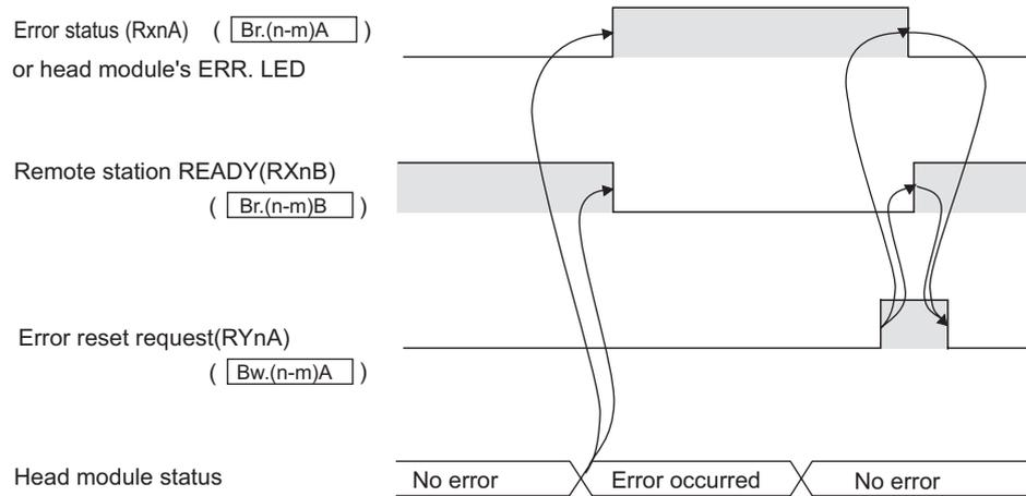
**Figure 3.7 When an error has occurred in the head module**
