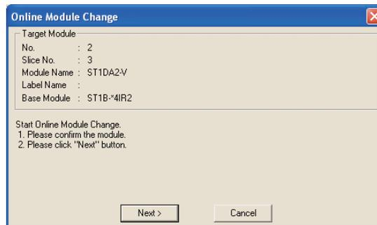
**Figure 4.21 Confirming the slice module to be replaced**
