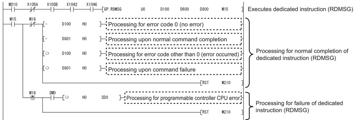
Figure 7.9 Program for setting command parameters (common to head module and slice modules) (continued)
