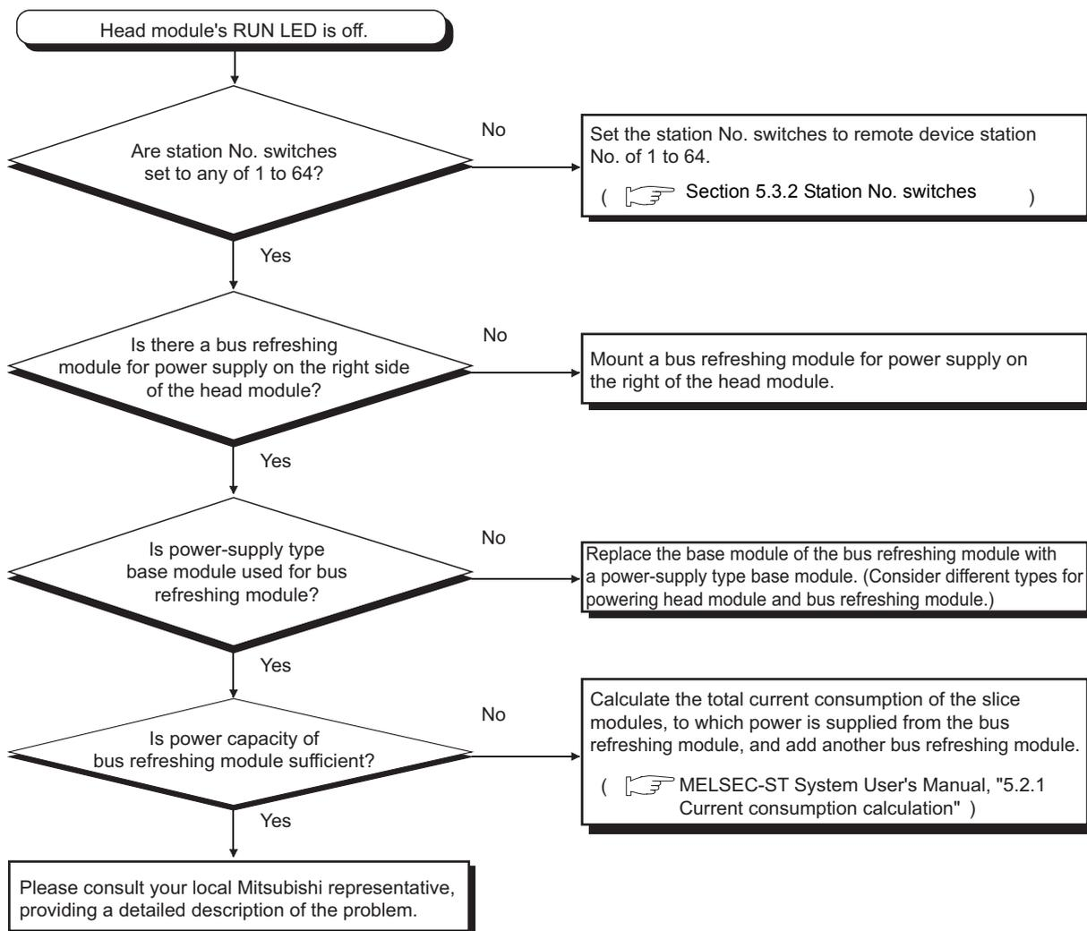
Figure 9.3 When the RUN LED is off
