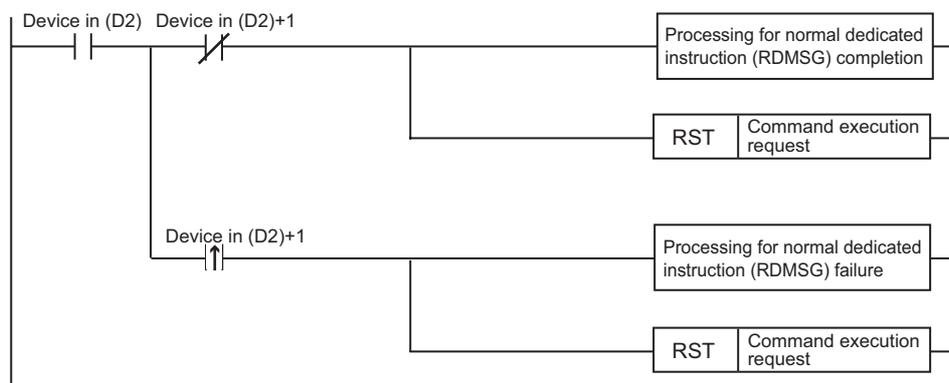
**Figure 8.6 Reading Cr Command result area**
