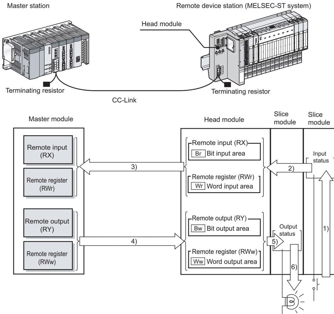
Figure 3.1 Communication between master station and MELSEC-ST system
