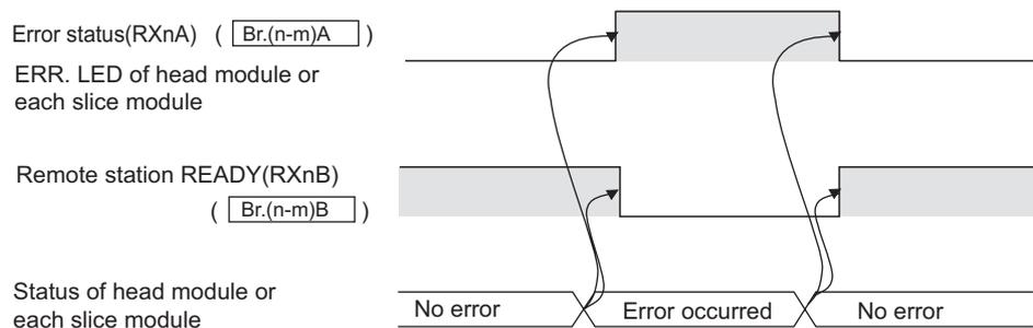
**Figure 3.6 Operation when an error occurs**
