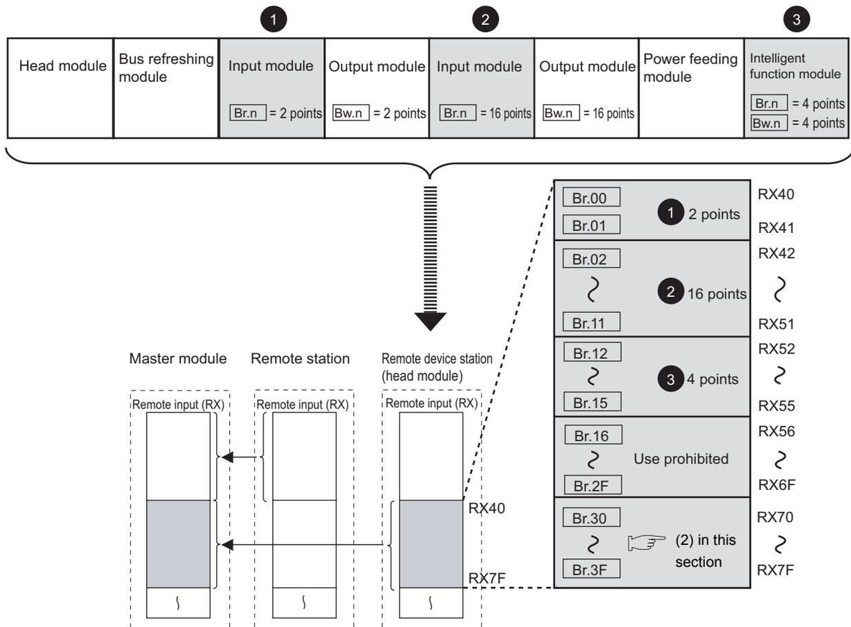
Figure 3.4 Input area assignment example
