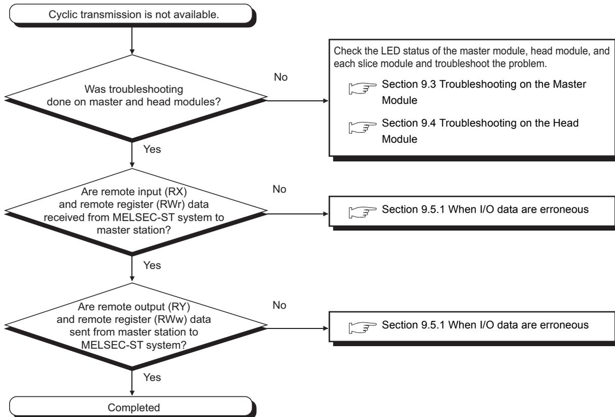
Figure 9.8 When cyclic transmission is not available
