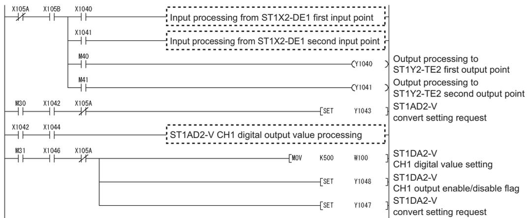
Figure 7.12 Program for controlling each slice module
