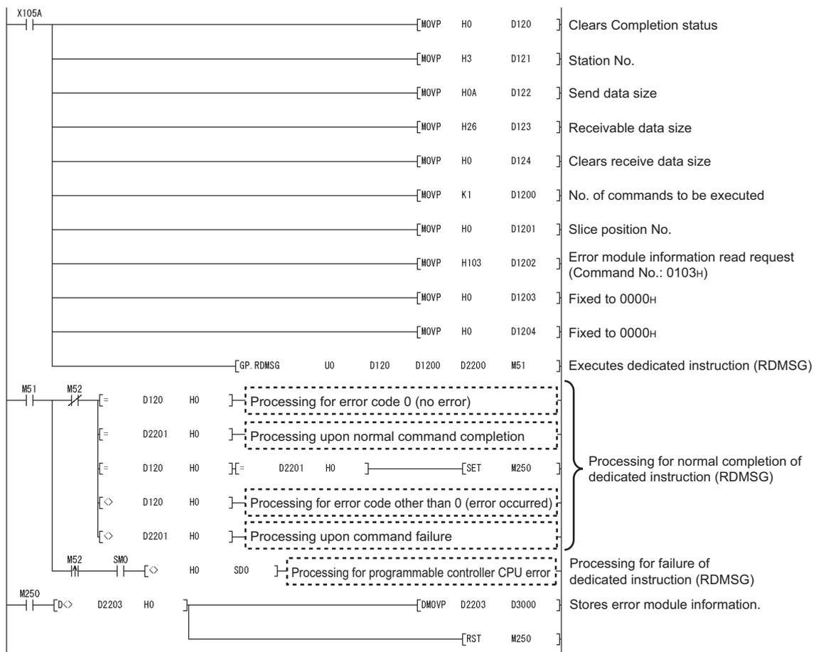
Figure 7.13 Program for reading error module information
