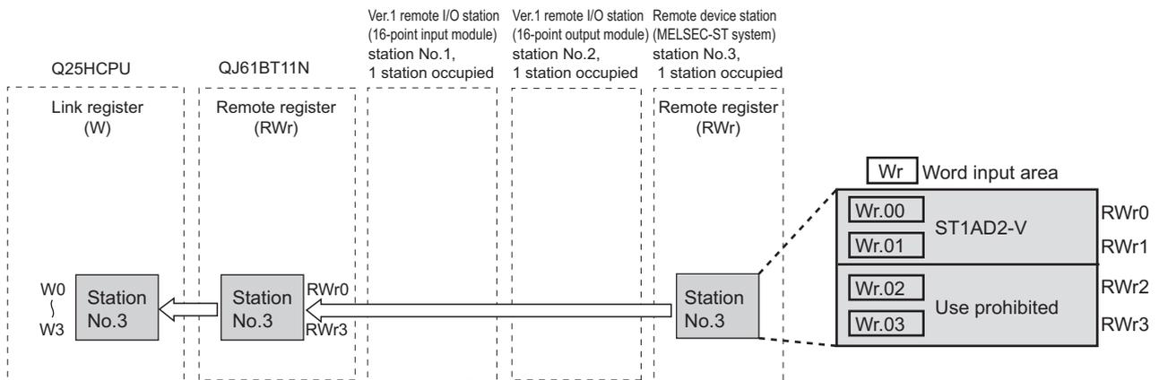
Figure 7.6 Remote register (RWr) assignment
