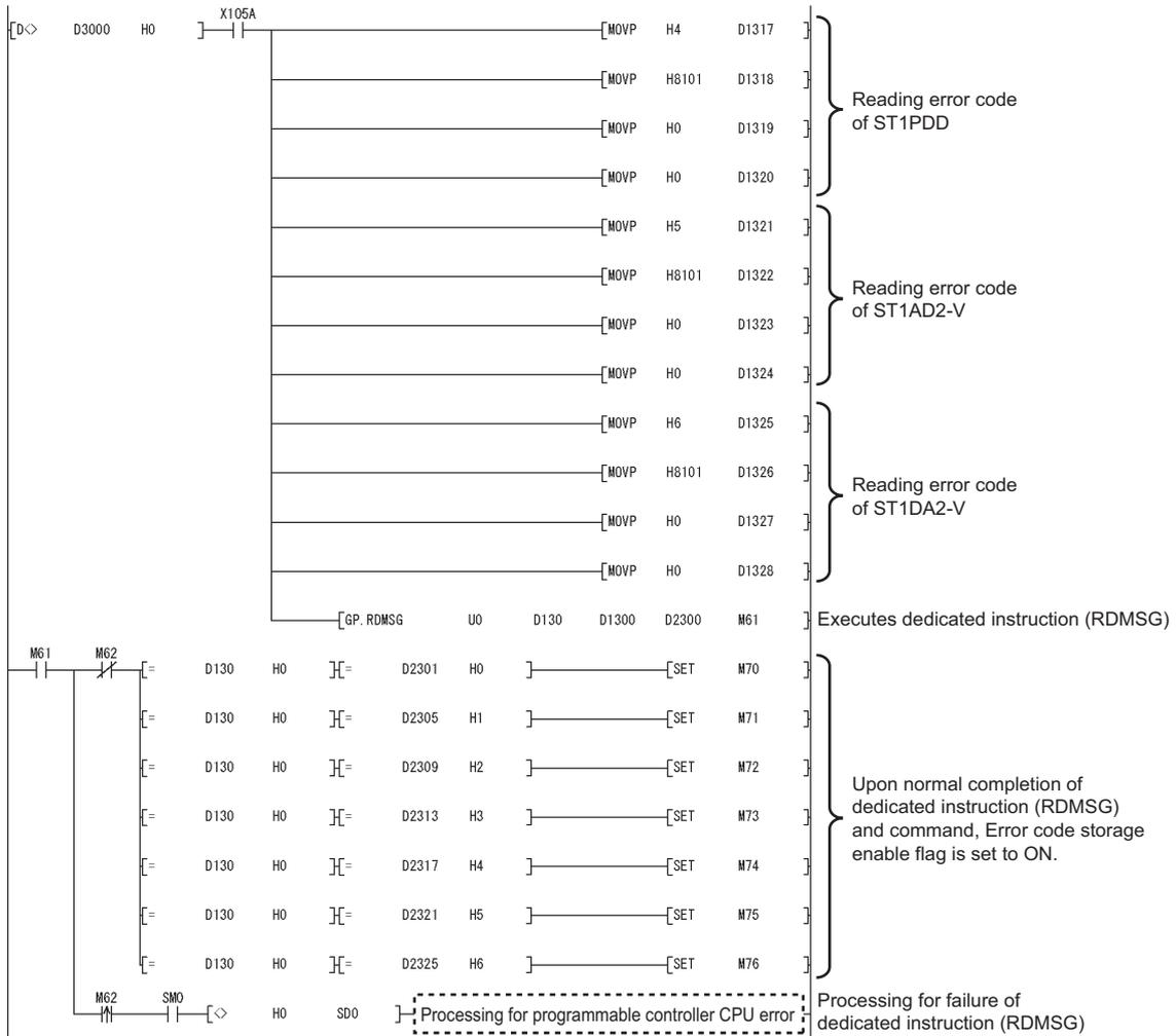
Figure 7.14 Program for reading error codes (continued)
