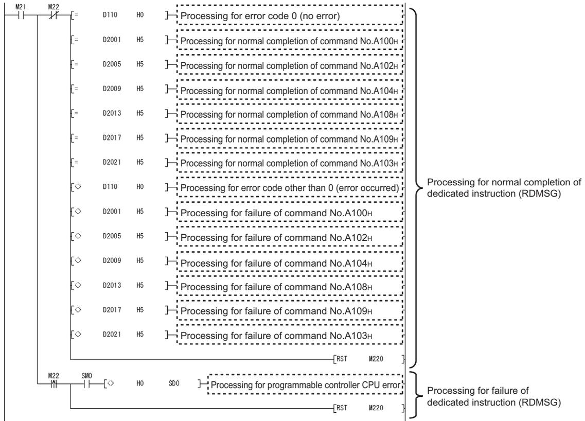
Figure 7.10 Program for setting command parameters (ST1AD2-V) (continued)
