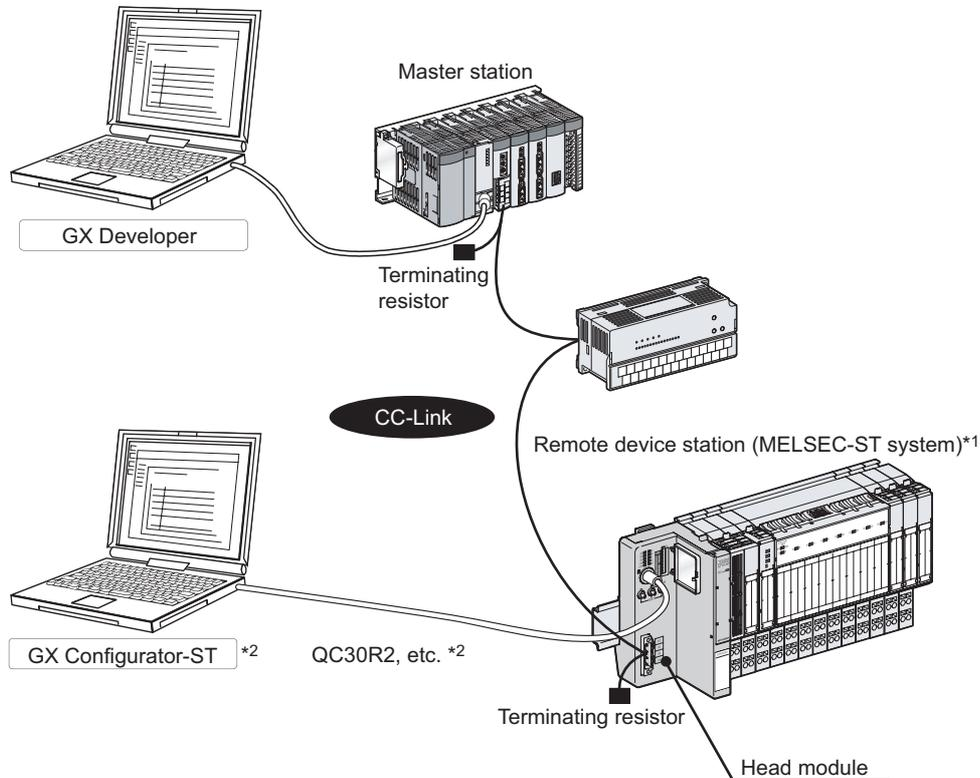
**Figure 2.1 System configuration**
