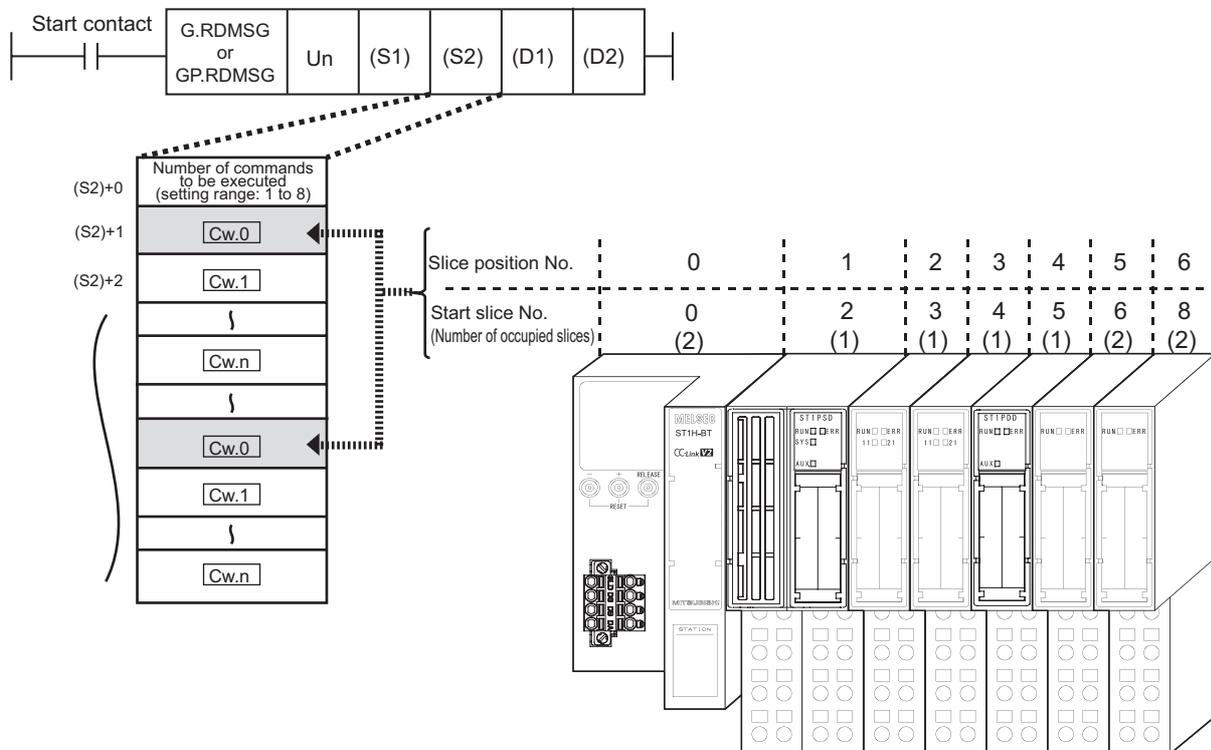
Figure 8.4 Difference between slice position No. and start slice No.
