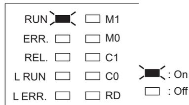
Figure 5.12 LEDs indicating normal completion
