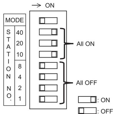
Figure 5.10 Station No. setting for self-diagnostics (Station No.70)
