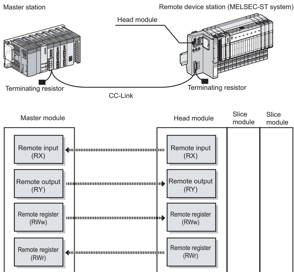
Figure 1.2 Connecting MELSEC-ST system to CC-Link
