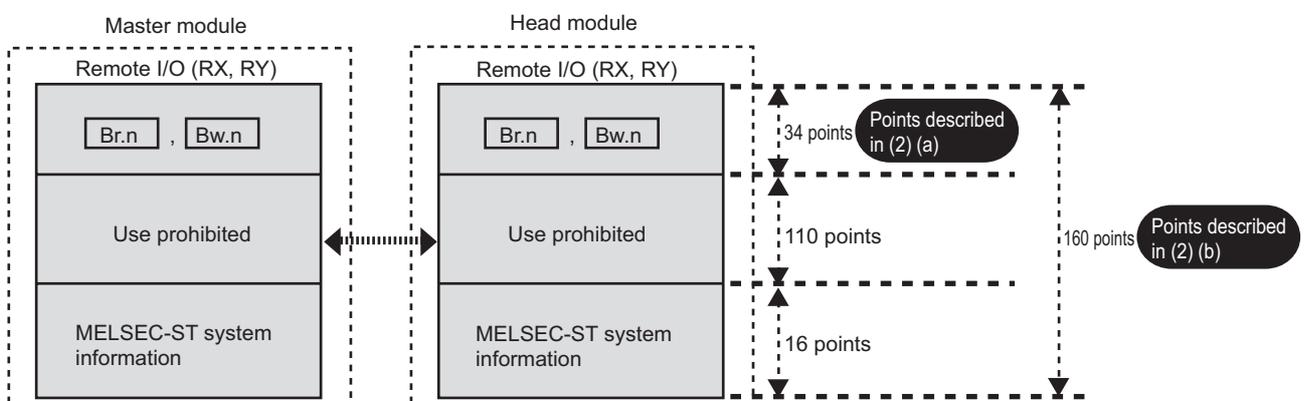
Figure 4.2 Cyclic transmission data sizes (Remote input/output (RX, RY))
