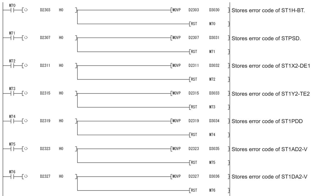
Figure 7.14 Program for reading error codes (continued)
