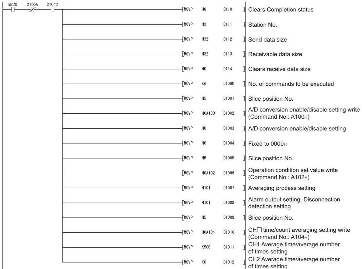
Figure 7.10 Program for setting command parameters (ST1AD2-V)
