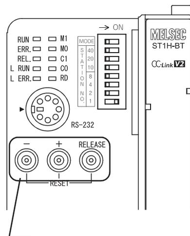
Figure 5.9 Resetting the head module
