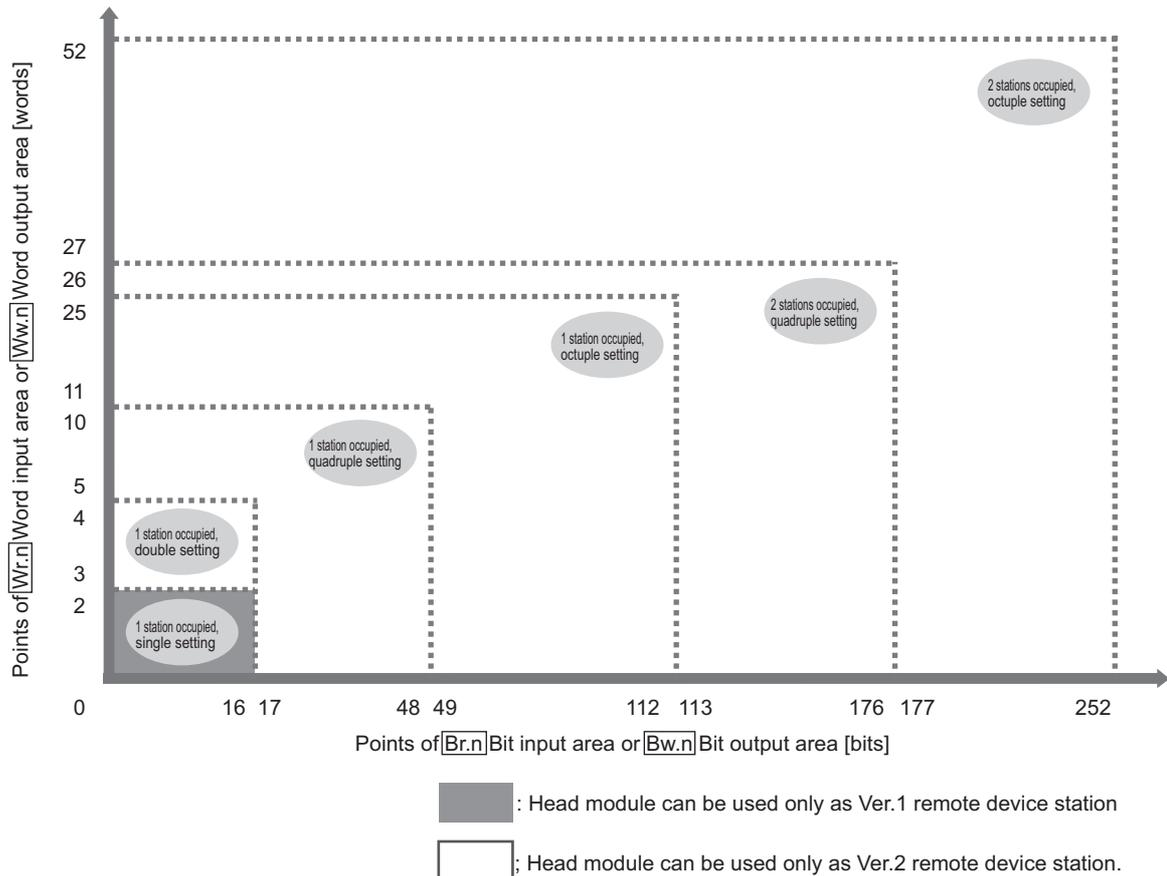
Figure 4.6 No. of occupied stations and extended cyclic settings in Priority min. stations mode
