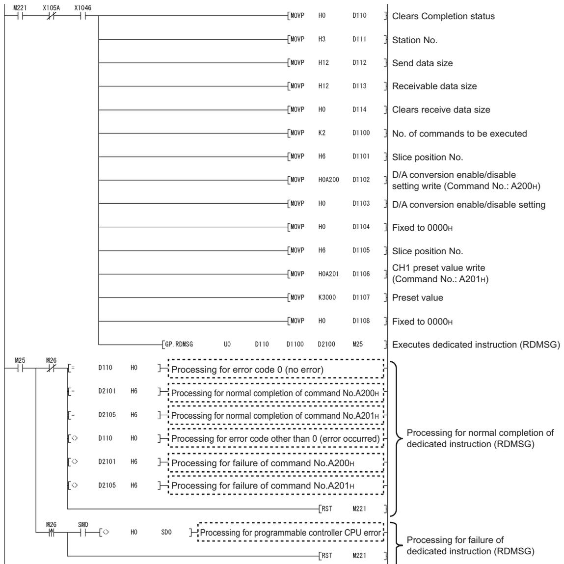
Figure 7.11 Program for setting command parameters (ST1DA2-V)
