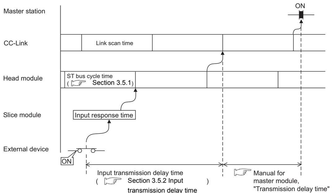
Figure 3.12 Processing of MELSEC-ST system → Master station
