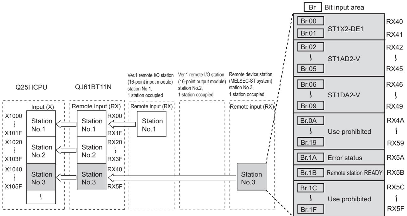
Figure 7.4 Remote input (RX) assignment
