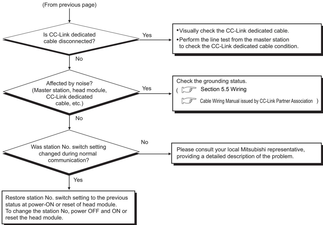
Figure 9.7 When the ERR. LED is flashing (continued)
