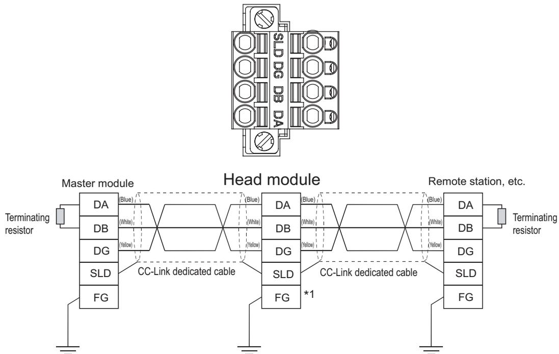
**Figure 5.18 CC-Link dedicated cable connection method**
