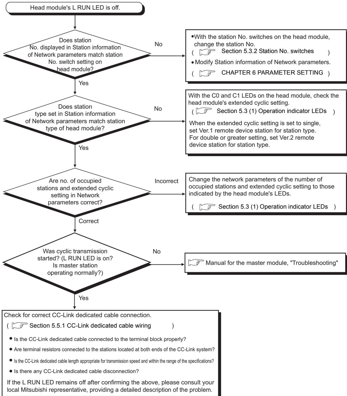
Figure 9.6 When the L RUN LED is off
