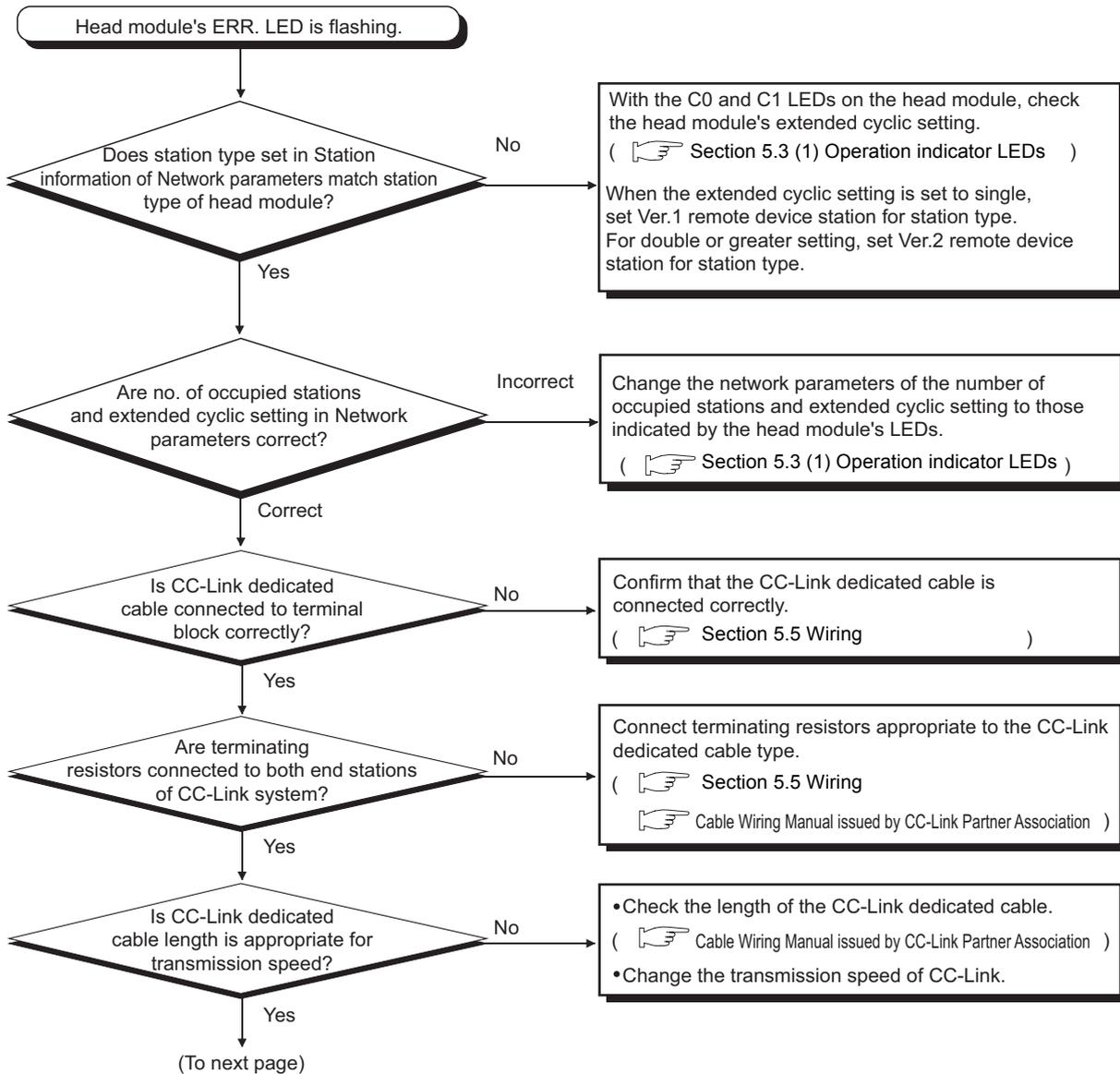
Figure 9.7 When the ERR. LED is flashing
