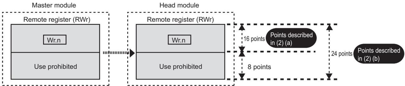
Figure 4.3 Cyclic transmission data sizes (Remote register (RWr))
