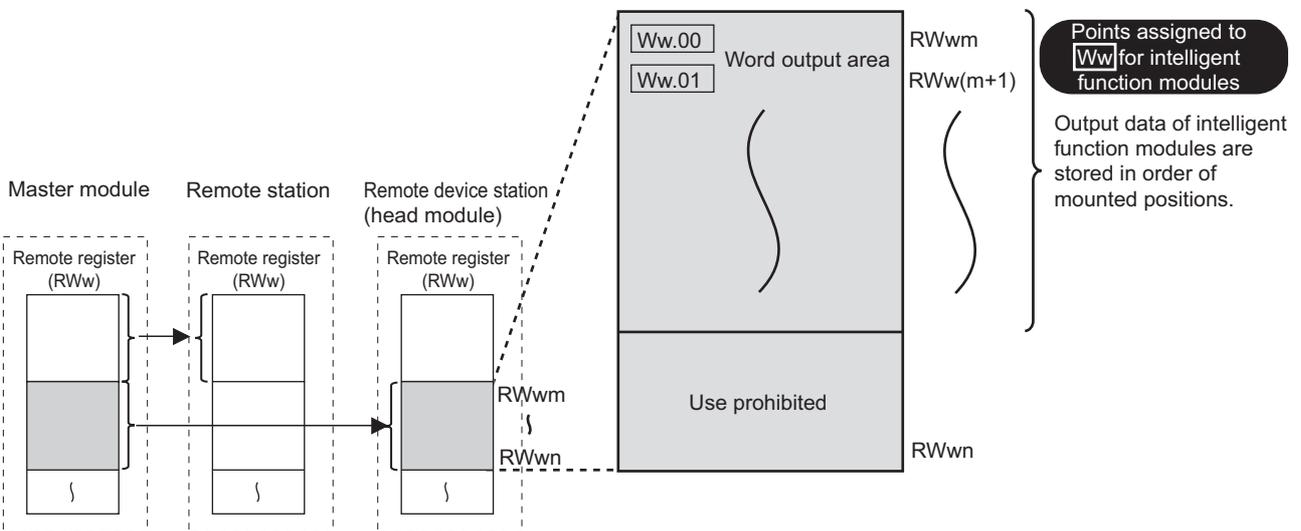
Figure 3.9 Configuration of remote register (RW<sub>w</sub>)
