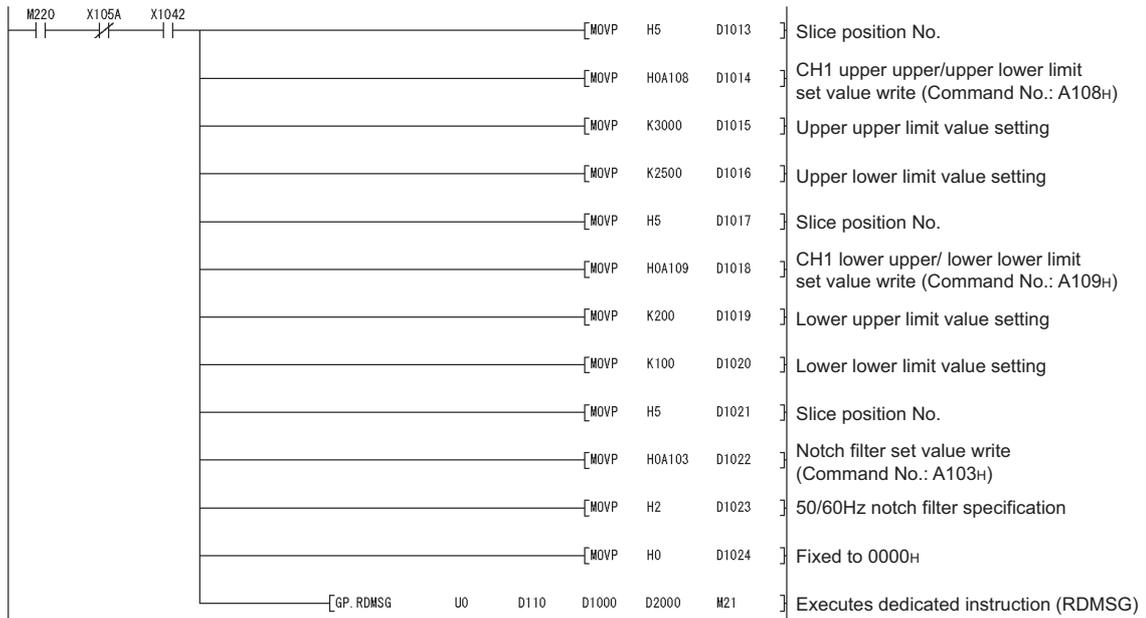
Figure 7.10 Program for setting command parameters (ST1AD2-V) (continued)
