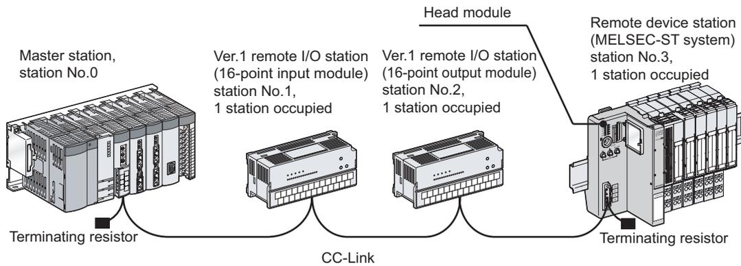
Figure 7.1 System configuration example
