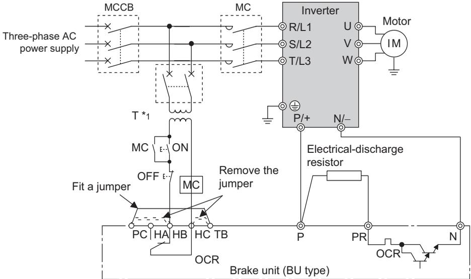
\*1. When the power supply is 400V class, install a step-down transformer.
