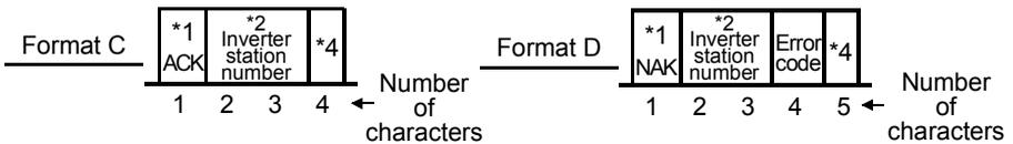
3) Reply data from inverter to computer during data read
