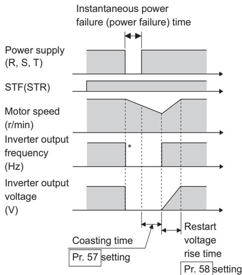
\* The output shut off timing differs according to the load condition.
