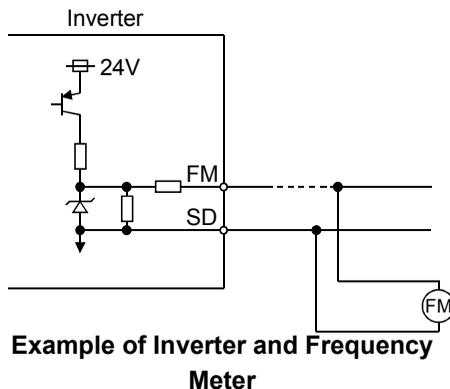
\*1. 0.5V or less when a DC ammeter of 300Ω or less internal resistance is connected to measure the output voltage.
