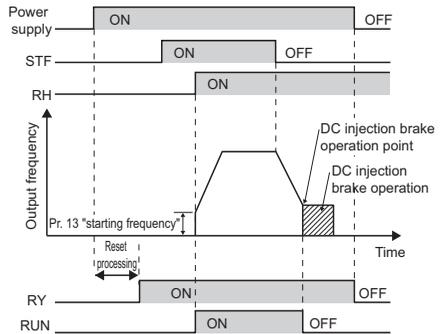
3) Checking the inverter operating status by the start signal input to the inverter and inverter running signal.
