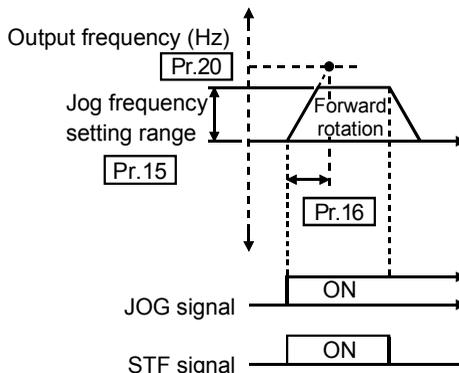
● Set the frequency and acceleration/deceleration time for jog operation.
