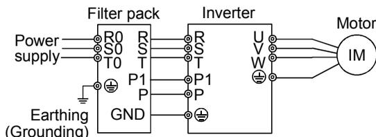
(For the type without filter pack, earth (ground) the motor with the inverter at one point on the inverter side.)
