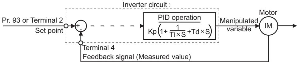
Kp: Proportion constant    Ti: Integral time    S: Operator    Td: Differential time
