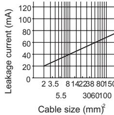
Leakage current example of three-phase induction motor during commercial power supply operation (200V 60Hz)
