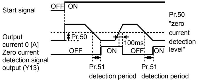
To prevent this, the output current "zero" signal can be output from the inverter to close the mechanical brake when the output current has fallen to "0[A]".
