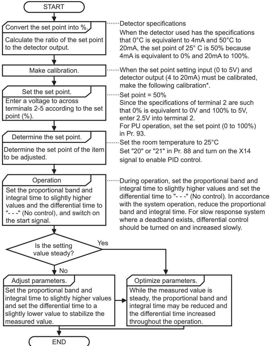
\*When calibration → Use Pr. 38 and calibration parameters C2 to C4 (terminal 2) and Pr. 39 and calibration parameters C5 to C7 (terminal 4) to calibrate the detector output and set point setting input. Make calibration in the PU mode when the inverter is at a stop.
