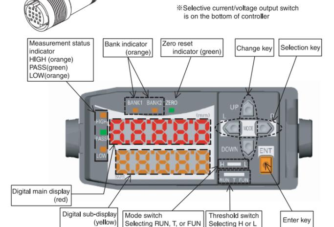
The current/voltage output selector for the analog output is on the bottom of the Controller.
