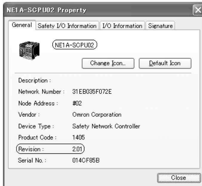
The device name and revision are given in the Property Dialog Box. The NE1A-series Controllers supported by Network Configurator are listed in the following table.
