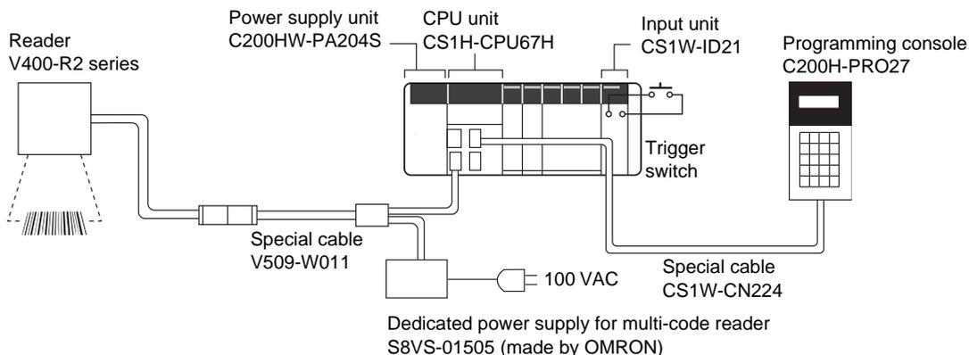
Connect the connection cable of this reader to RS-232C port of the CPU unit.
