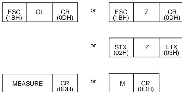
The continuous reading trigger command format is as shown below.
