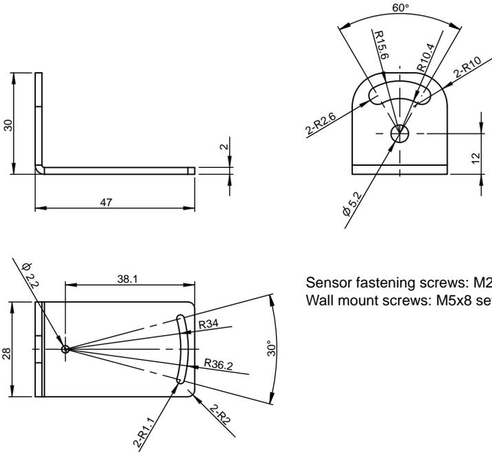
Sensor fastening screws: M2x5 set screws x2
