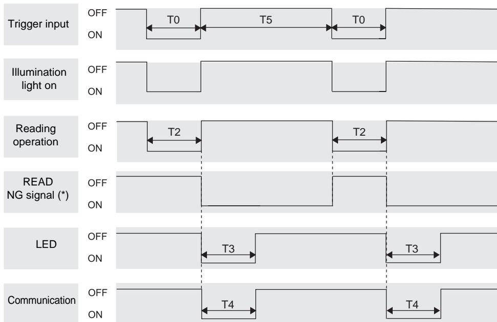
\*The READ NG signal is output when any code other than the labels registered in "Setting for label registration" (p.89) is read.
