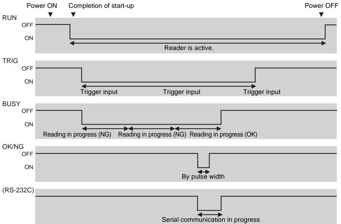
■ When [Continuous] is Selected as Trigger Mode and [OK Pulse] is Selected for [OK/NG Output]
