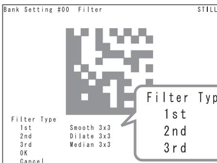
Performing image processing before reading reduces possibility of reading error.
