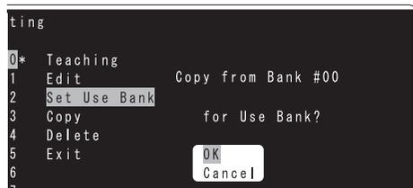
An asterisk (\*) will appear at both right and left ends of the reading condition to be normally used.
