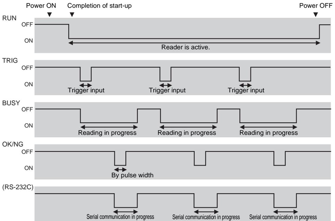
■ When [One Shot] is Selected as Trigger Mode and [Level] is Selected for [OK/NG Output]
