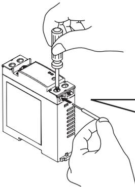
Connect the brown wire to the positive (+) side of the power supply and the blue wire to the negative (-) side.
