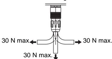
When disconnecting a cable, hold the part of the plug shown below and then pull it out straight.
