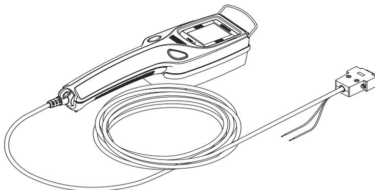
The 2D Code Reader is designed to read two-dimensional code. A built-in monitor and zoom lens are ideal for reading directly marked 2D code.
