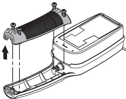
3. Remove the bush from the slot on the case.
