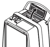
2. Position the Memory Card in the correct direction and insert in the slot until a click is heard.
