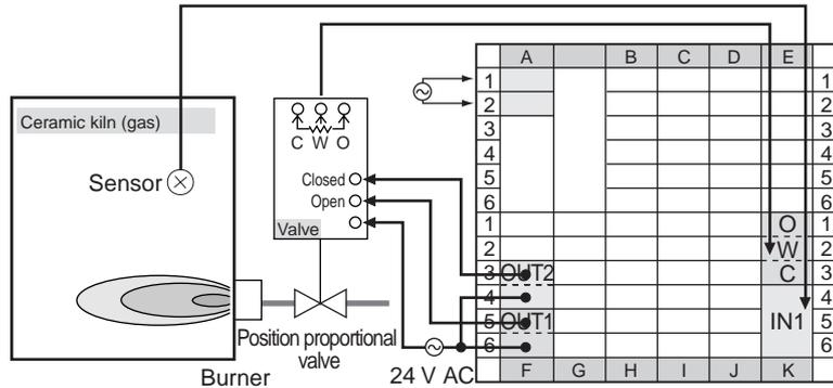
When using floating control, there is no need to connect a potentiometer (C, W, O) unless the amount of valve opening is being monitored.
