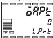
This function restricts key operation in Operation, Adjustment, Adjustment 2, Bank setting, PID setting, Approximation setting and Monitor item levels.
