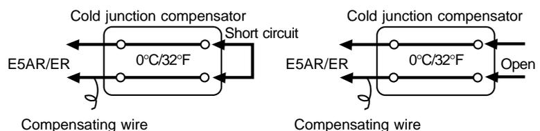
Follow these steps to perform calibration when thermocouple input is selected.
