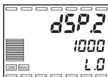
1. Hold the
