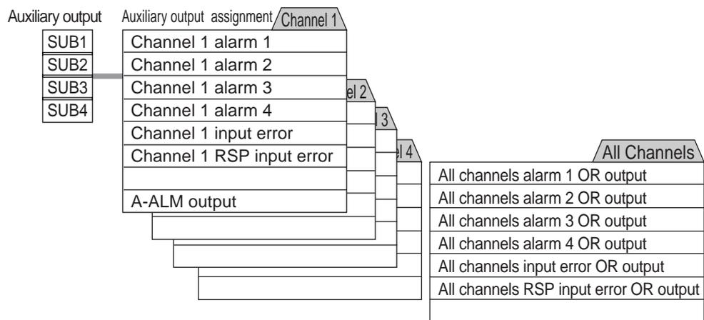
U-ALM output is an OR output (overall alarm) of alarms 1 to 4 of all channels.
