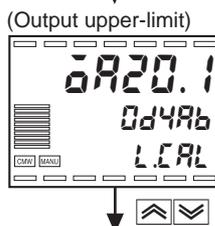
4. While viewing the output on the DMM, use the keys to set the output to 20 mA. In the example at left, "20 mA" appears at a value 2 digits smaller than before calibration.
