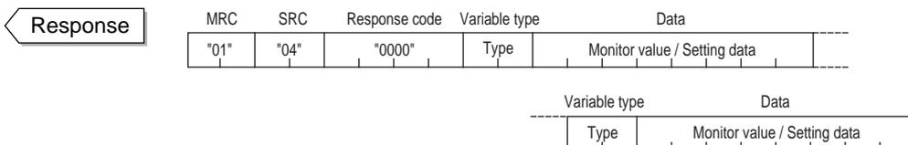
Response codes: The above indicates a normal end. For the response codes, see "6.5 Reading the variable area" (P.6-9).
