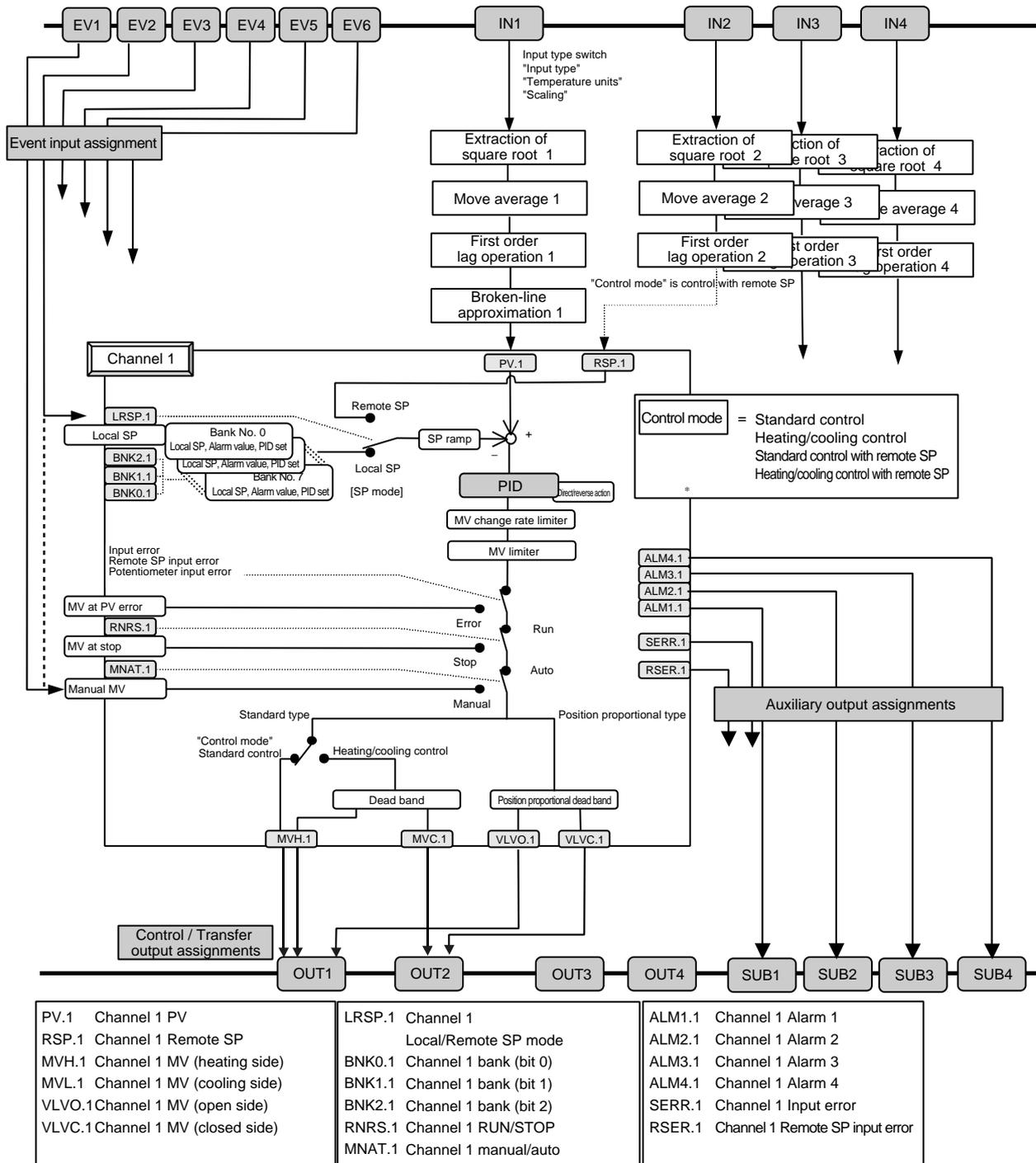
Multi-point input types have the same setting data for channels 2 to 4 depending on the number of input points.
