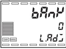
6. Press the  key less than 1 second to move from "RUN level" to "Adjustment level".
