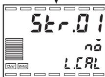
7. Press the key to obtain the display at left. Note that this display will not appear if not all of the required data has been tentatively saved, or if the data has not been changed.
