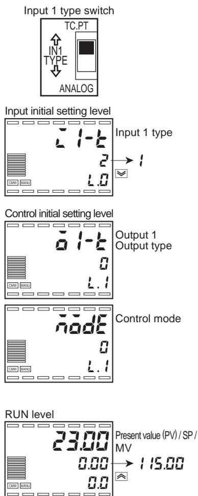
1. Before turning on the power, check that the input 1 type switch is set to TC. PT.
