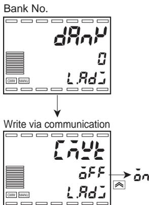
To allow a host computer to write setting data to a controller, set "Write via communication" (Adjustment level) to "on: Enabled".
