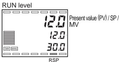
When the ratio setting (AP1) is 0.05 and the measured value of input 2 is 240.0 kg/s, control of the dye takes place using an SP of 12.0 kg/s.
