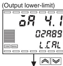
5. Press the key to obtain the display at left and begin 4 mA calibration.
