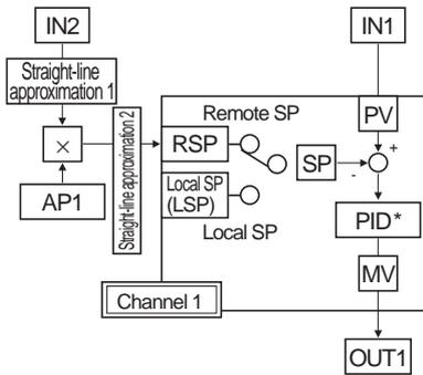
Ratio control is achieved by multiplying input 2 (which serves as a reference) by the proportion and using the result as remote SP.
