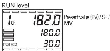
1. After the power is turned on, "PV/SP/MV" of the primary loop appears (ch 1). (Here we assume that cascade control is in progress using near SP of 180.0°C)
