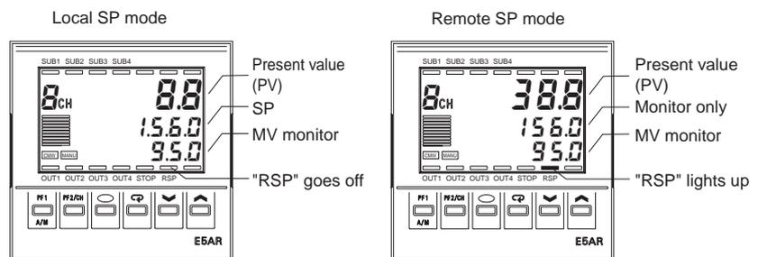
• When using a bank in local SP mode, a link is created to the local SP of the selected bank. For example, if Bank 3 is selected, the local SP of Bank 3 appears in Display 2, and when the value is changed, the value of "Bank 3 local SP" (Bank setting level) also changes.
