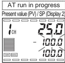
If you attempt to move to "RUN level" and show "PV/SP" while AT is running, Display 2 will blink and indicate that AT is running.
