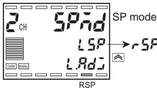
8. Press the  key to select the secondary (ch 2) "SPAd: SP mode". Press the  key to select "rSP: Remote SP". The RSP operation indicator will light up in remote SP mode to indicate cascade control (cascade closed).
