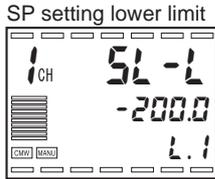
The SP setting upper and lower limits can be set within the input setting range.
