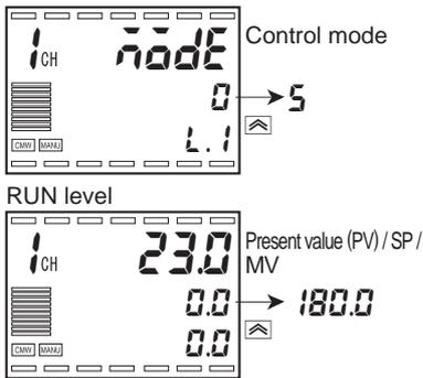
3. Press the key repeatedly to select "mode: Control mode". Press the to select "5: Cascade standard control".
