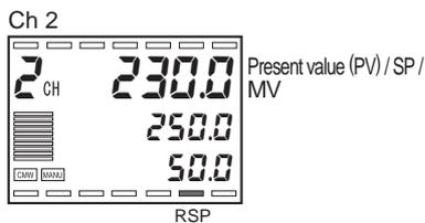
2. Press the key to select the secondary (ch 2) "PV/SP/MV". The RSP operation indicator lights on to indicate that the system is in the cascade control (cascade closed) state. (Here we assume that the secondary PV is 230.0°C. The secondary local SP will be set to 230.0°C in step 5.)
