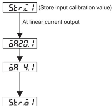
If user calibration was performed on any of inputs 1 to 4 or outputs 1 to 6 following purchase of the controller, user calibration completion information will appear as shown below when you move to Calibration level.
