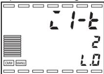
1. Turn on the power and then hold down the  key for at least 3 seconds to move from "RUN level" to "Input initial setting level".
