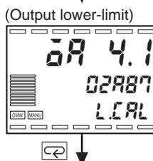
6. While viewing the output on the DMM, use the keys to set the output to 4mA. In the example at left, "4 mA" appears at a value 2 digits smaller than before calibration.
