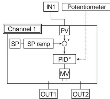
To control a gas kiln using a position proportional control valve, select the control valve control type and configure the instrumentation as shown in the following example.
