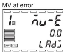
This setting is used to output a fixed MV when an input error PV error or remote SP input error occurs.
