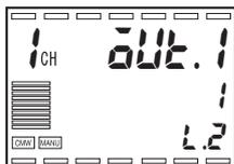
1. Hold down the  key at least 3 seconds to move from "RUN level" to "Input initial setting level".
