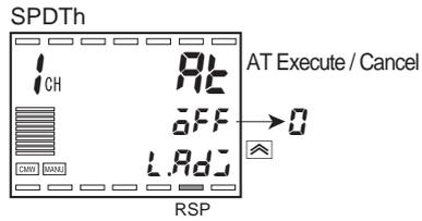
9. Press the **[CH]** key and then press the **[Rt]** repeatedly to select "Rt: AT Execute / Cancel" of the primary loop (ch 1). Press the **[0FF]** key to change the set value to "0" and run primary AT. During AT the automatically selected PID Set No. is displayed and display 1 (**Rt**) blinks. When AT finishes, display 2 changes to "0FF" and display 1 (**Rt**) stops blinking.
