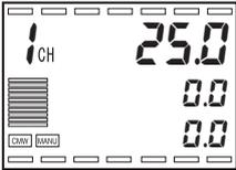
1. Hold down the **[PF]** key for Auto / Manual at least 1 second. The MANU indicator lights up and the mode changes to manual.
