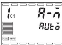
2. Press the **[M]** key to switch to "āMANU: Manual". The MANU indicator lights up and the mode changes to manual.
