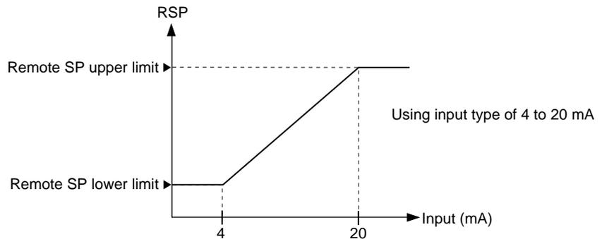
Note that the SP limits are in effect, and therefore if the input remote SP is above or below the SP limits, the SP will be clamped to the upper or lower limit.
