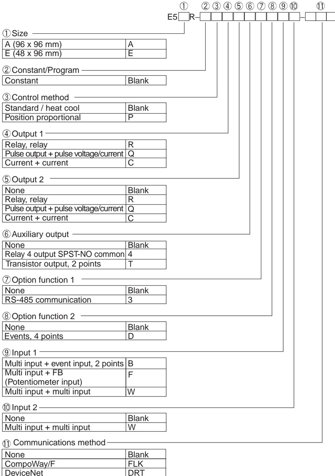
The above is an explanation based on functionality. There may be some differences from the product line depending on the combination of features selected. Please check the catalogue when ordering. For details on using DeviceNet communications functions, refer to the *E5AR/E5ER Digital Controller DeviceNet Communications User's Manual (H124)*.
