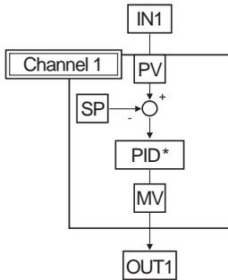
When controlling a heater plate for semiconductor wafers with the E5AR, the control mode is set to standard control and instrumentation is as shown in the following example.
