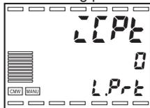
This setting restricts access to Input initial setting, Control initial setting, Control initial setting 2, Alarm setting, Display adjustment, and Communications setting levels.
