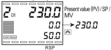
5. Press the  key repeatedly to return to "RUN level". The secondary (ch 2) "PV/SP/MV" will appear. Set the secondary SP to "230.0", which is the PV obtained in step 2.
