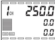
1. The display normally shows "PV/SP". The SP is "0.0" °C.
