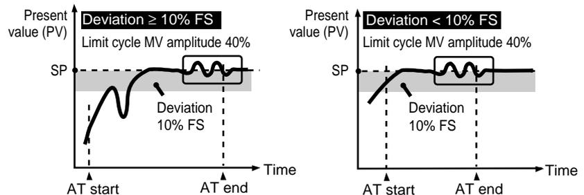
The amplitude of change of the limit cycle MV can be changed in "Limit cycle MV amplitude".
