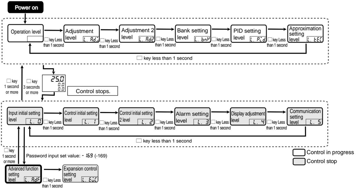
To move to Advanced function setting level, set "Initial setting level protect" in Protect level to "0", and then enter the password (-169) in "Move to Advanced function setting level" (Input initial setting level).
