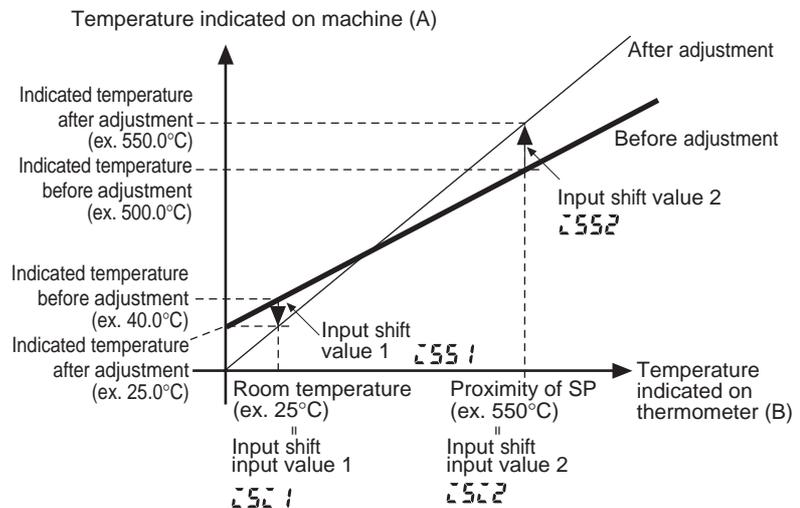
(Image adjustment by point adjustment of Fig. 2.2)
