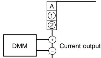
3. Press the key to obtain the display at left and begin 20 mA calibration.
