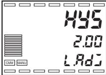
To perform ON/OFF control, the "SP", "Proportional band", and "Hysteresis (heat)" settings must be configured.
