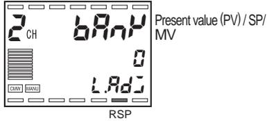
3. Press the  key less than 1 second to move from "RUN level" to "Adjustment level".
