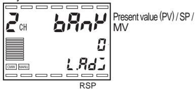
6. Press the  key less than 1 second to move from "RUN level" to "Adjustment level".
