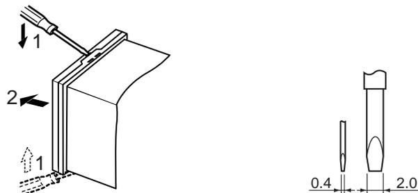
When pulling the unit out, place a cloth over the screwdriver to prevent scratches and other damage.
