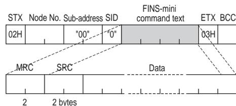
**Response text** FINS-mini response text consists of the MRC and SRC, followed by an MRES (main response code) and SRES (sub response code), and then the required data.
