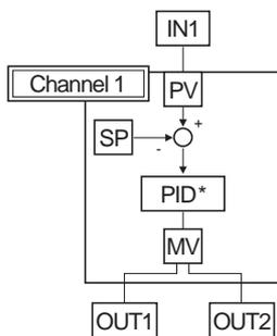
When the E5AR is used to control a chemical reaction device, the control mode is set to heating/cooling control and instrumentation is as shown in the following example.
