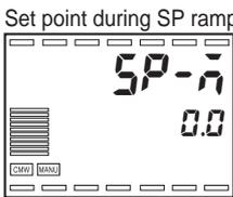
The SP ramp function limits the amount of change of the SP to a set rate. When this function is enabled and the amount of change exceeds the set rate, a space that limits the SP is created as shown in the diagram below
