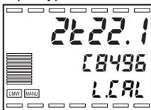
Wait until the count in Display 2 is sufficiently stable and then press the key. This tentatively saves the calibration data at this point.
