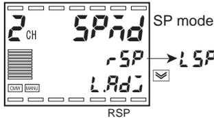
4. Press the  key repeatedly to select the secondary (ch 2) "SPAd: SP mode". Press the  key to set the SP mode to "LSP: Local SP". The RPS operation indicator is off in local SP mode, indicating independent control (cascade open) in the secondary loop.
