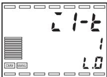
1. Make sure that the input 1 type switch is set to TC.PT and then turn on the power.
