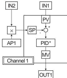
This machine mixes a constant proportion of flowing sand and dye in order to dye the sand a uniform color.
