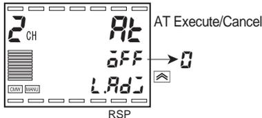
7. Press the  key to select the secondary (ch 2) "At: AT Execute / Cancel". Press the  to change the set value to "0" and run AT. During AT the automatically selected PID Set No. is displayed and display 1 (At) blinks. Display 2 shows "OFF" when AT finishes, and display 1 (At) stops blinking.
