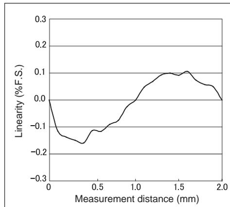
Measuring Sensing Objects of Different Sizes after Adjusting Linearity with Standard Sensing Object
