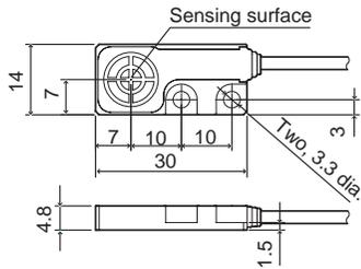
Sensor mounting hole dimensions
