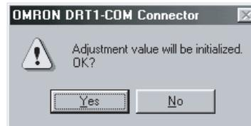
The offset and gain settings stored in the EEPROM in the Analog Output Unit will be reset to the default values. Reset the Unit to enable the default settings.
