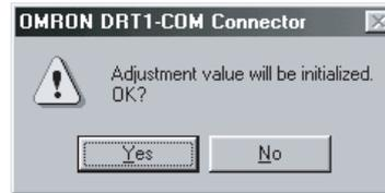
The offset and gain settings stored in the EEPROM in the Analog Input Unit will be reset to the default values. Reset the Unit to enable the default settings.
