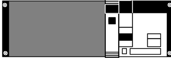
I/O Units are where the control connections are made from the PC to all the various input devices and output devices. As you can see from the figure above, there is still some space available on the left side of the Backplane. This space is for any additional I/O Units that may be required.
