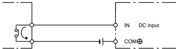
When using the configuration shown below, the sensor and Input Unit should receive their power from the same supply.
