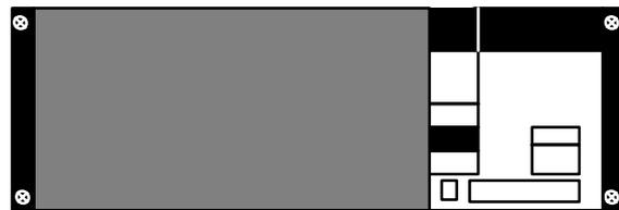
The CPU of the C200H has no I/O points built in. So, in order to complete the PC we need to mount one or more I/O Units to the Backplane. Mount the I/O Unit to the Backplane by locking the top of the I/O Unit into the slot on the Backplane and rotating the I/O Unit downwards as shown in the following diagram. Press down on the yellow tab at the bottom of the slot, press the I/O Unit firmly into position, and then release the yellow tab.
