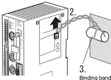
4. Install a new battery in the reverse order of removal.
