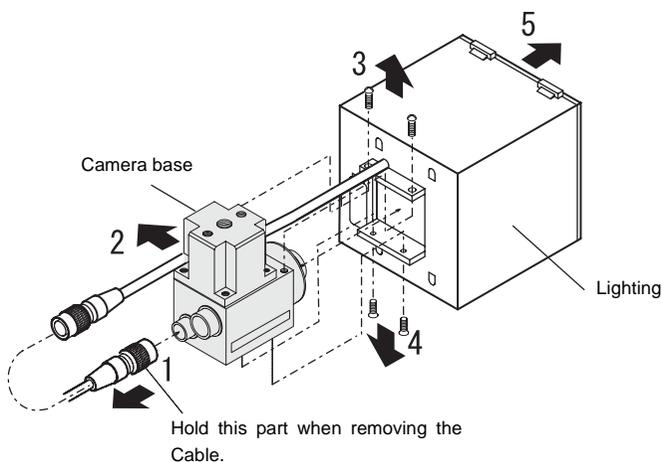
1. Disconnect the light cable from the light connector on the back of the Camera.
