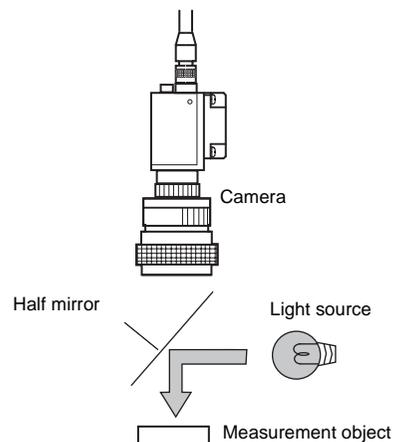
Applications: Surface inspections, positioning, and hole inspections of comparatively small objects
