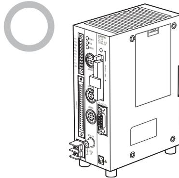
Do not install the Controller upside down as shown in the following diagram.
