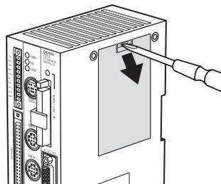
The battery is installed behind this cover.
