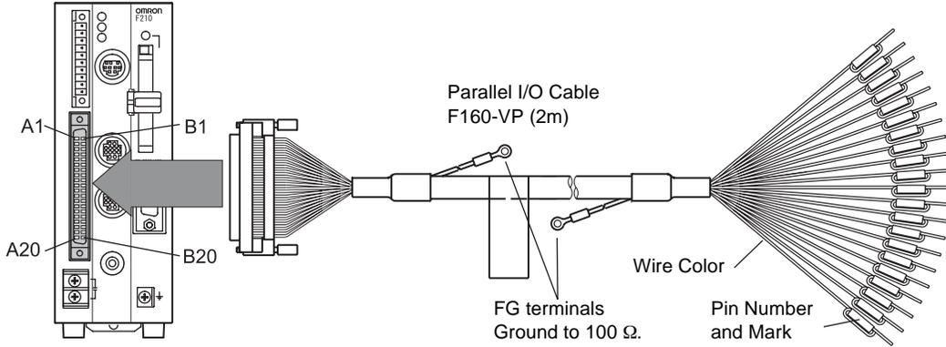
**NOTICE** Turn OFF the power supply before connecting or disconnecting a Parallel I/O Cable. Peripheral devices may be damaged if the cable is connected or disconnected with the power ON. The parallel connectors are capped with screw-on covers when the Controller is shipped. When the connector is not being used, leave the cover in place or replace the cover to protect against dust, dirt, and static electricity.
