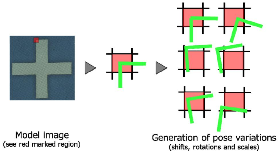
Fig.8. the variation-absorbing templates method
