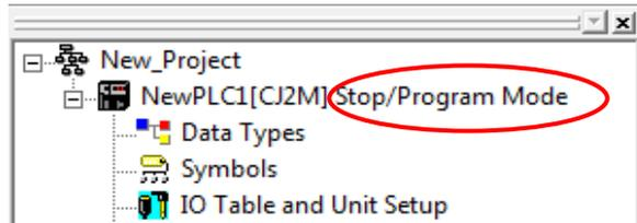
2 Select **Edit - I/O Table and Unit Setup** from the PLC Menu of CX-Programmer.
