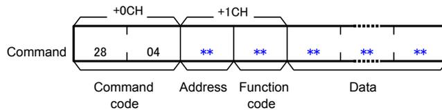
\*Command code #2804 is known as the FINS command for Modbus-RTU communication.
