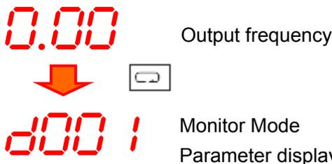
\*If the output frequency is not displayed in Data display, press and hold the **Mode** Key for 3 seconds or more to display the output frequency.
