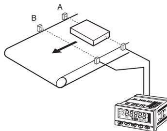
Measuring Differences in Length of Workpiece Steps
