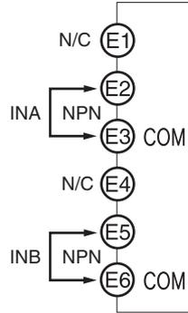
**Note:** E3 and E6, as well as B6 are internally connected.
