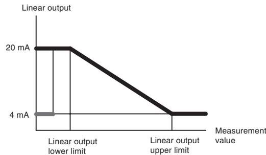
\* If the upper and lower limit are set to the same value, then the upper limit will equal the lower limit plus 1 for linear output.
