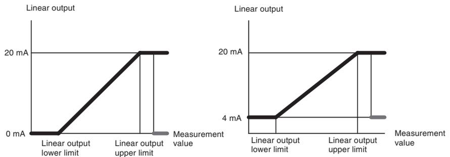
\* If operation stops without performing a measurement, then the minimum value (e.g., 4 mA for the 4 to 20 mA range) is output.
