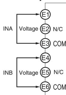
**Note:** E3 and E6, as well as B6 are internally connected.
