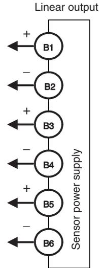
**Note:** Terminals B2 and B4 and terminals B2 and B6 are internally connected. If they are connected to a host device with a shared common, an unwanted current path may be created, preventing the correct signals from being output. If that occurs, provide isolation with a signal converter (an isolator) or other method.
