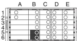
The sensor power can be supplied from terminals B5 and B6. The power supply specifications are outlined below.
