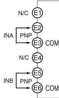
**Note:** E3 and E6, as well as B5 are internally connected.
