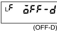
Output OFF delay is set using the following parameter.
