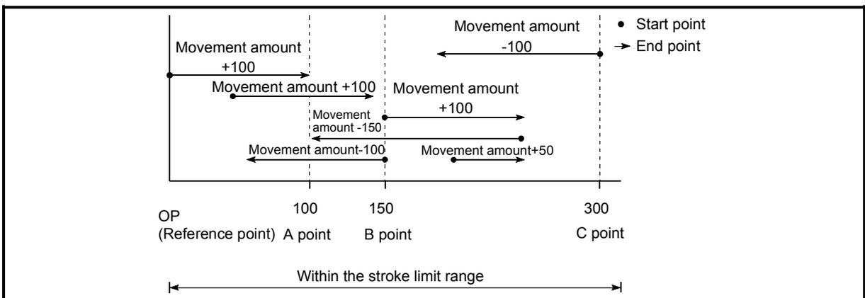
Fig. 9.6 Incremental system positioning control
