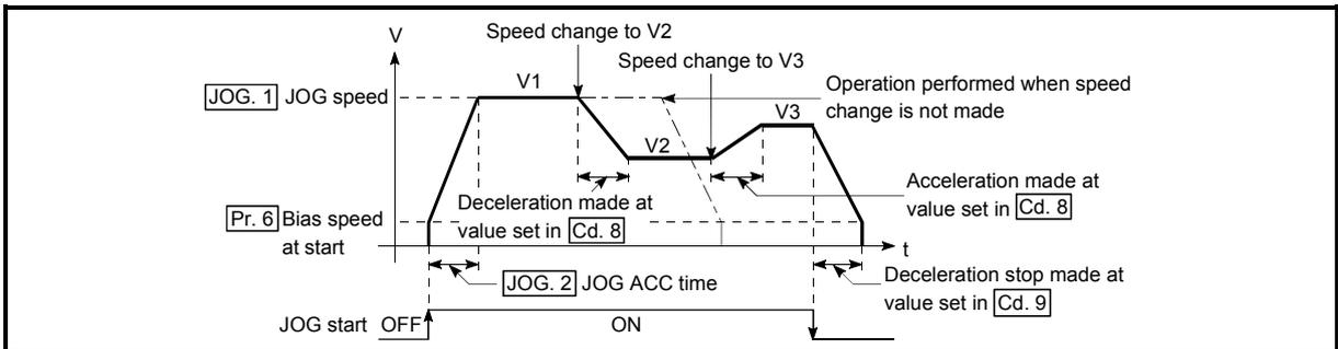
Fig. 11.1 Speed change operation
