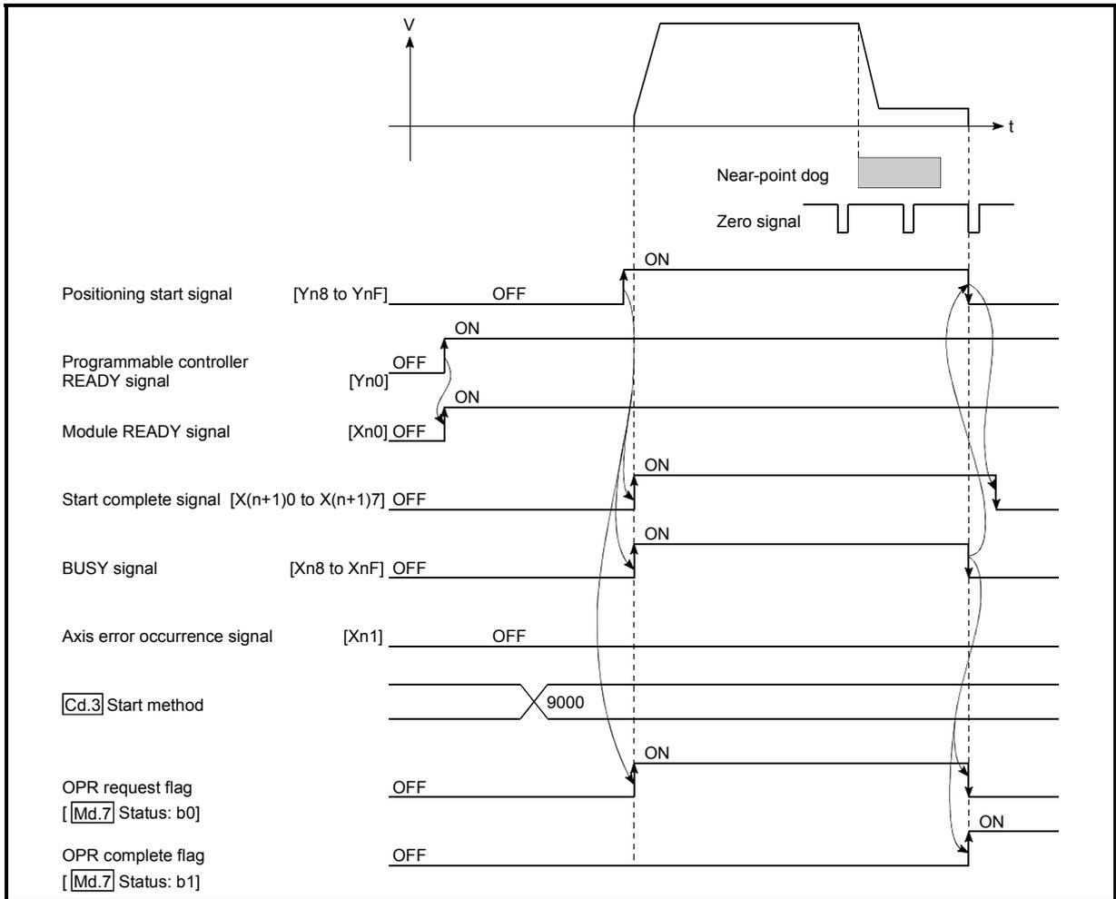
Fig. 7.4 Machine OPR control starting timing chart
