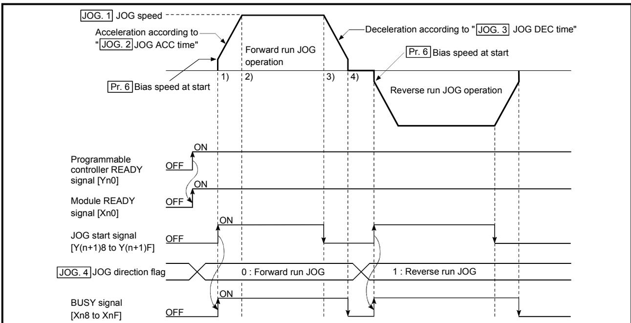
Fig. 10.1 JOG operation starting timing chart
