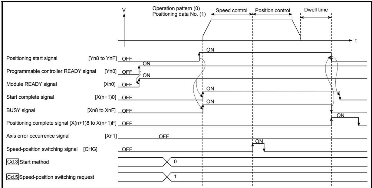
Fig. 7.7 Speed-position switching control starting timing chart
