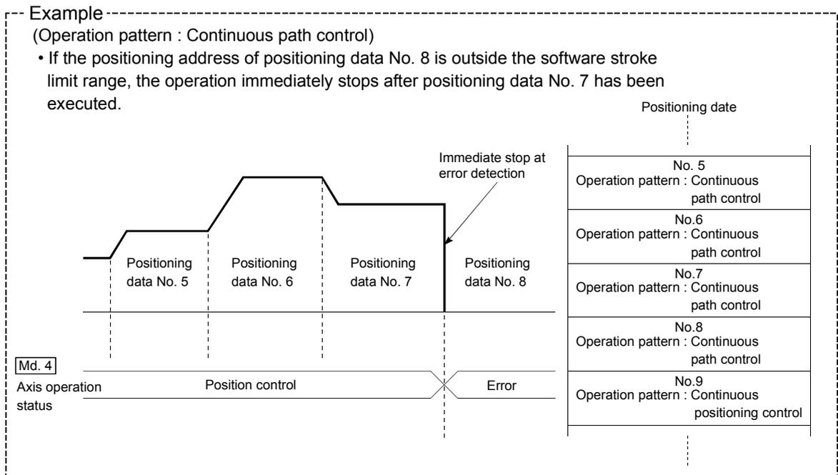
[5] Setting the software stroke limit function
