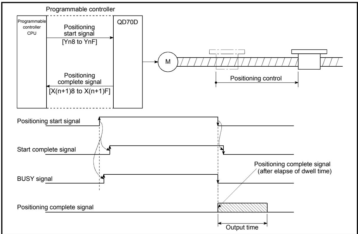
Fig. 4.2 Positioning complete signal output time
