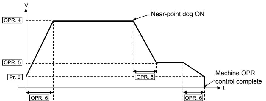
Pr. 6 Bias speed at start, OPR. 4 OPR speed, OPR. 5 Creep speed
