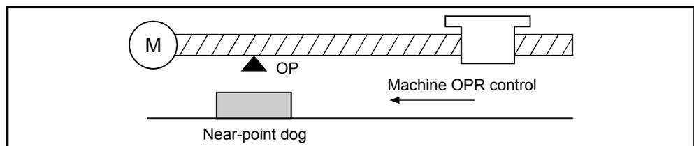
Fig. 8.1 Example of a machine OPR control
