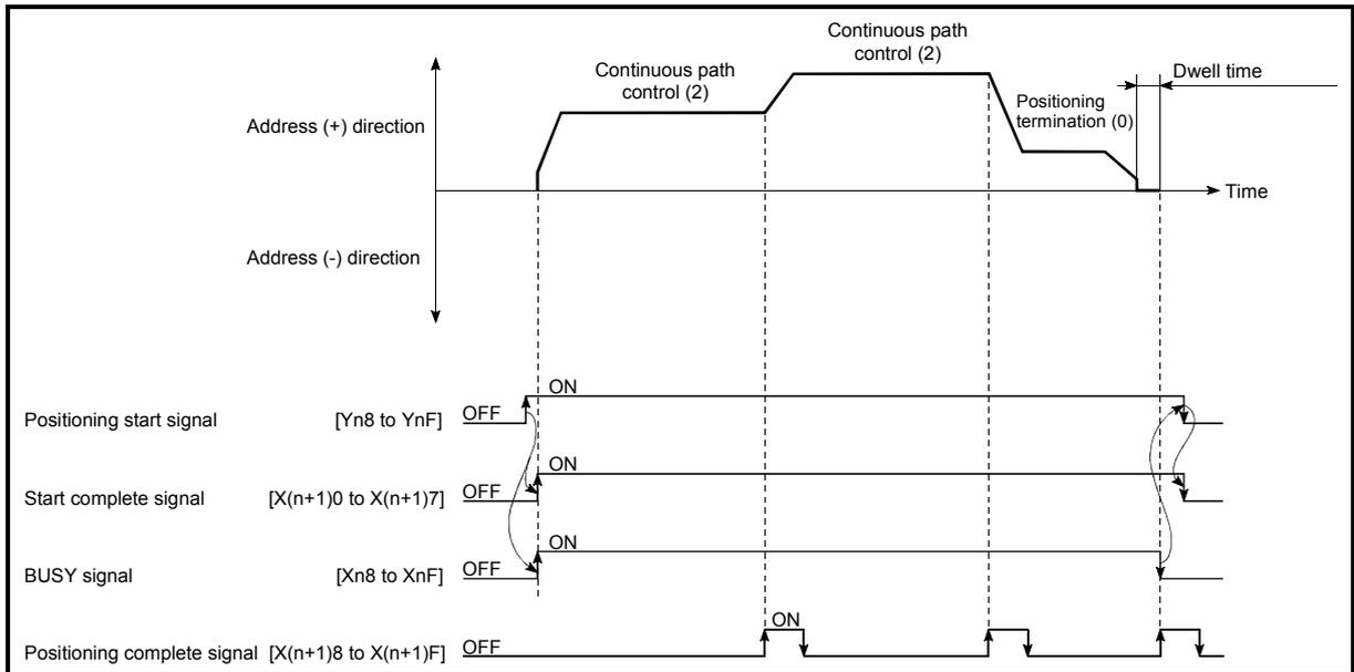
Fig. 9.3 Operation for continuous path control
