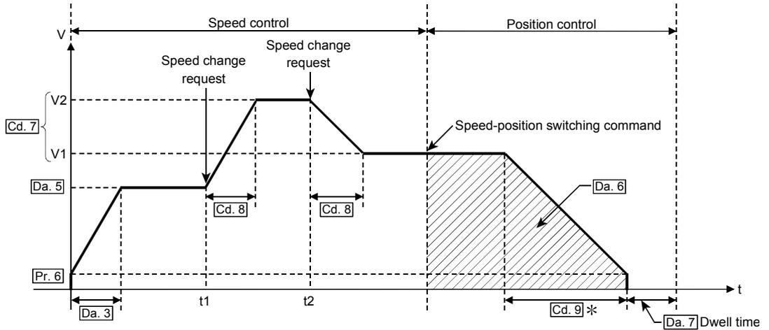
Pr. 6 Bias speed at start, Da. 3 ACC/DEC time, Da. 4 DEC/STOP time
