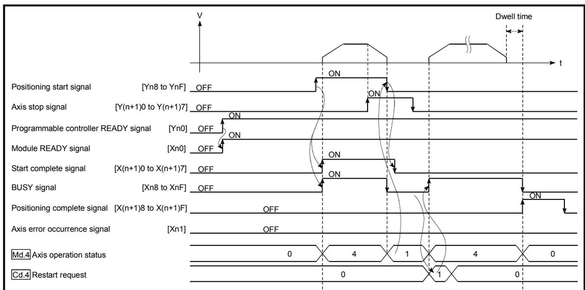
Fig. 7.10 Restarting timing chart (for position control)
