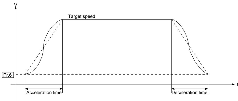
Fig. 11.7 Setting and operation of "Acceleration/Deceleration method"
