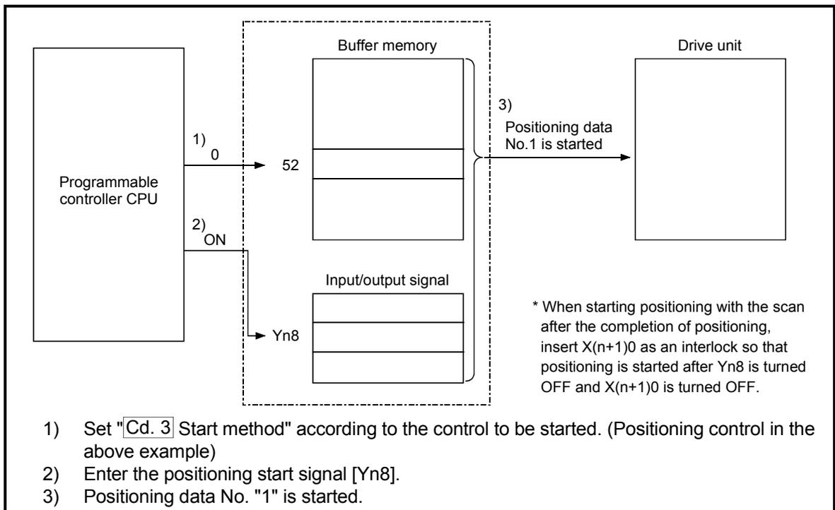
Fig. 7.2 Procedures for starting control (for axis 1)
