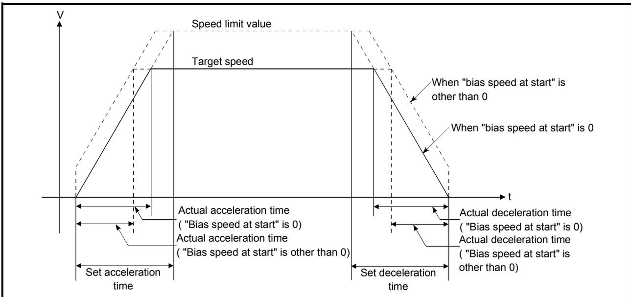
\* The operation of the acceleration/deceleration processing function of the AD75 is the same as that of the QD75.
