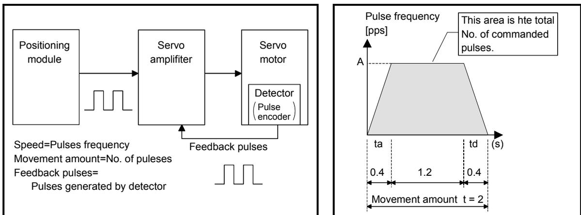
Fig. 1.1 Relationship between position control and speed control
