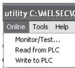
[Monitor/Test] : Activates the Select monitor/test module screen.
