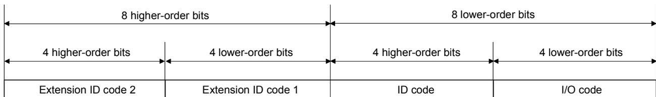
Configuration data structure of AS-i Ver. 2.04-compatible slave
