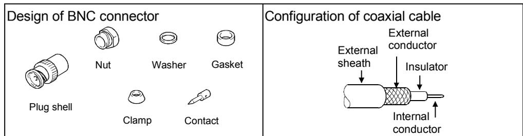
Fig. 5.4 Configuration of BNC connector and coaxial cable
