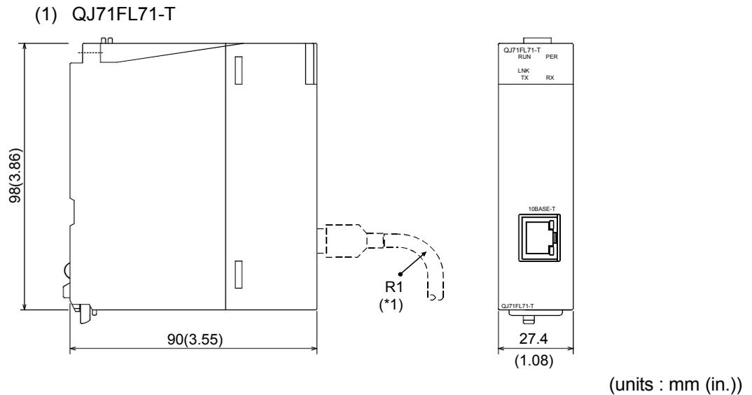
\*1 When connecting the twisted pair cable, set the bending radius near the connector (reference value: R1) as four times the cable's outside diameter or larger.
