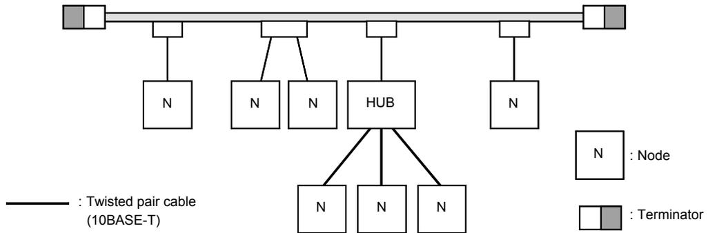
In addition, if the distance between nodes is short, the twisted pair cable can be connected to the HUB without passing through a coaxial cable or transceiver.
