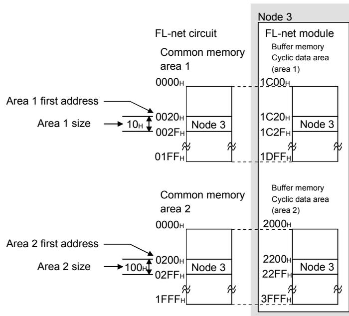
**(4) Common memory assignment****(a) Common memory assignment of the local node**
