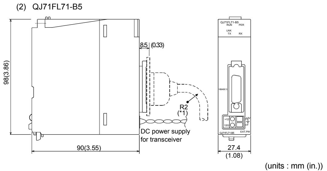
\*1 When connecting the AUI cable, set the bending radius near the connector (reference value: R2) as four times the cable's outside diameter or larger.
