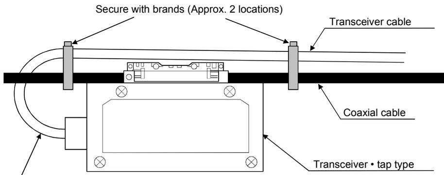
Take the bending radius of the transceiver cable into consideration (the smallest bending radius is 80 mm)
