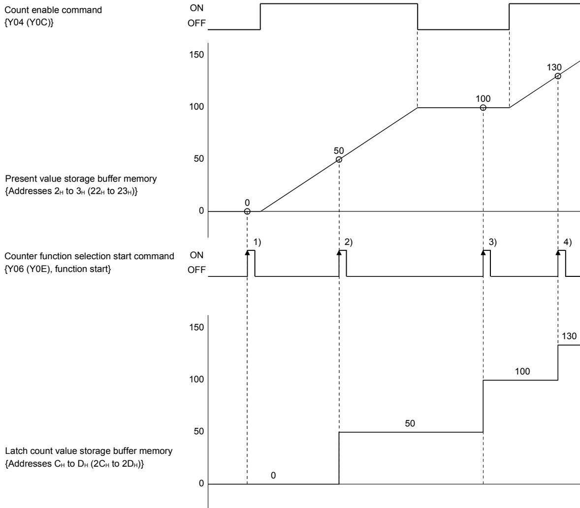
When the counter function selection start command {Y06 (Y0E), function start input} rises at points indicated by 1) to 4) in the figure above, the present counter value is stored in the latch count value storage buffer memory {addresses C<sub>H</sub> to D<sub>H</sub> (2C<sub>H</sub> to 2D<sub>H</sub>)}. The latch counter function is executed regardless of whether the count enable command {Y04 (Y0C)} turns ON/OFF.
