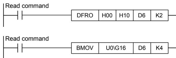
Depending on the relation between the update timings of the previous and present periodic pulse count values inside the module and the read timing in the sequence program, the previous value may be the same as the present value. If this has occurred, execute the reading again. (See Section 8.2.)
