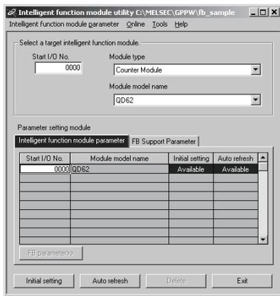
Enter "Start I/O No.", then select "Module type" and "Module model name".
