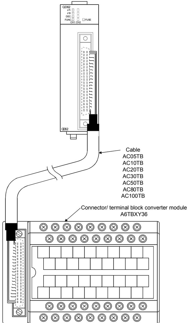
(2) The following table lists the signal names and the corresponding connector side terminal numbers and terminal block side terminal symbols, when a connector/terminal block converter module is used in the QD62(E/D) .
