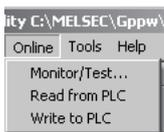
[Monitor/Test] : Activates the Select monitor/test module screen.
