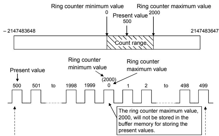
(a) The ring counter will operate as follows when the "present value < ring counter minimum value" or "ring counter maximum value < present value".
