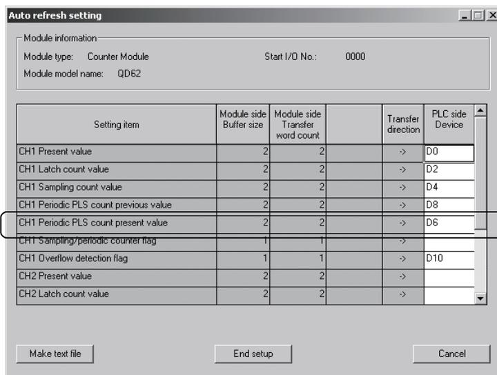
The number of settings in this one line is counted as one setting. The number of settings is not counted by columns. Add up all the setting items in this setting screen, then add them to the total for the other intelligent function modules to get a grand total.
