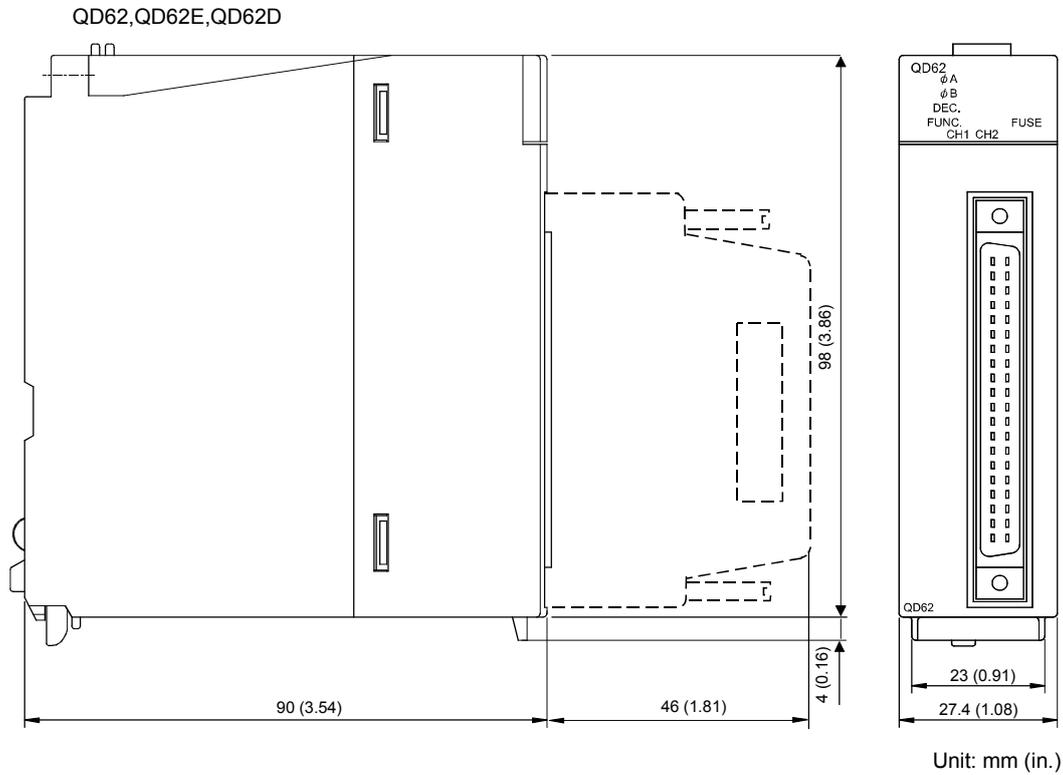
A value in parentheses shows the reference measurement when the A6CON1 is installed.
