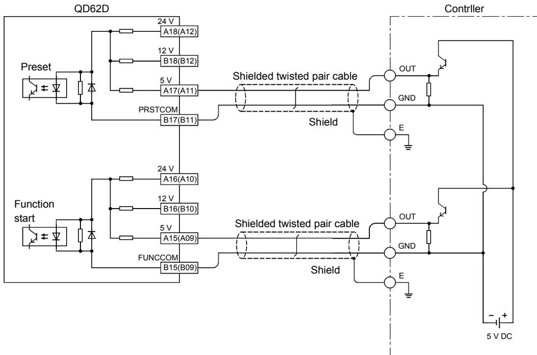
The number inside the ( ) indicates the terminal number for channel 2.
