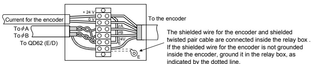
4.4.2 Wiring example of a module and an encoder
