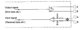
The following type of the RS-422 connector is used. The counter connector must match this connector
