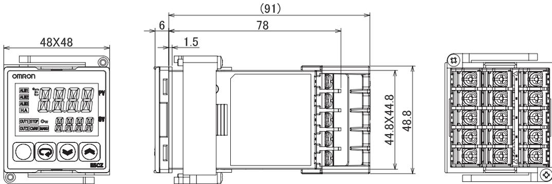
**Note:** Do not remove the terminal block. Doing so may result in failure or malfunction.
