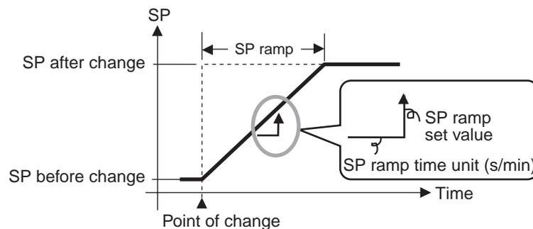
The rate of change during SP ramp is specified using the "SP ramp set value" and "SP ramp time unit" parameters. The "SP ramp set value" parameter is set to OFF by default, i.e., the SP ramp function is disabled.
