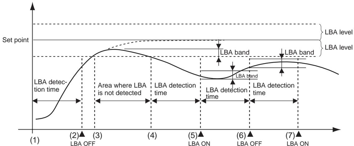
If the control deviation is reduced in the area between 1 and 2 (i.e., the set point is approached) and the amount the control deviation is reduced is at least equal to the LBA band, the loop break alarm will remain OFF.
