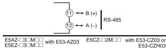
Specify both ends of the transmission path including the host computer as end nodes (that is, connect terminators to both ends).
