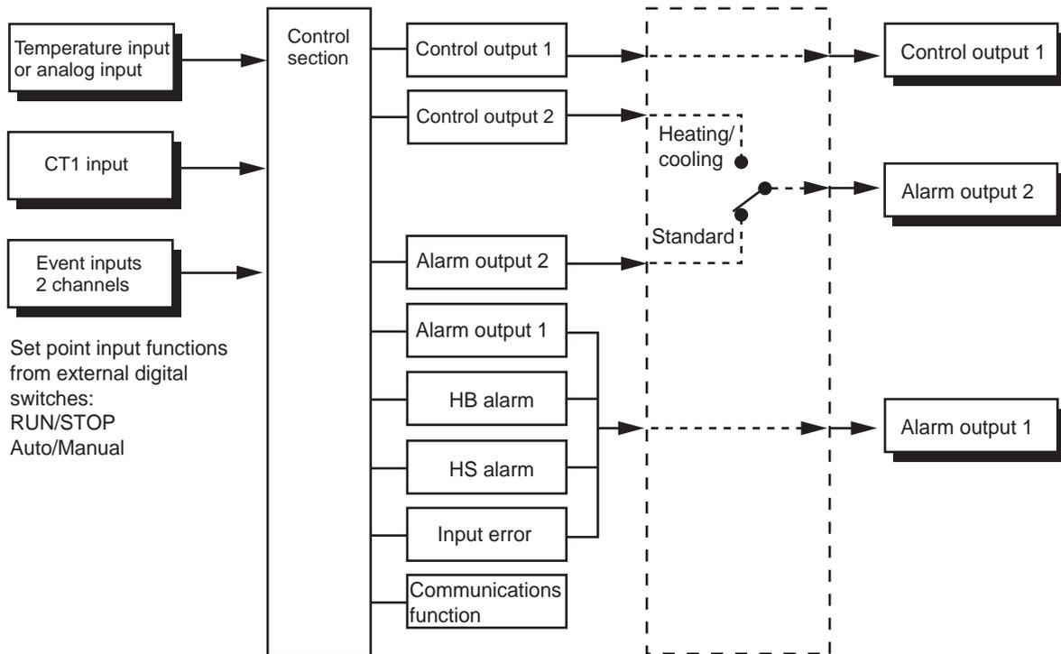
**Note** Functions can be assigned individually for each output by changing the set values for the control output 1 assignment, the alarm output 1 assignment, and the alarm output 2 assignment in the advanced function setting level.
