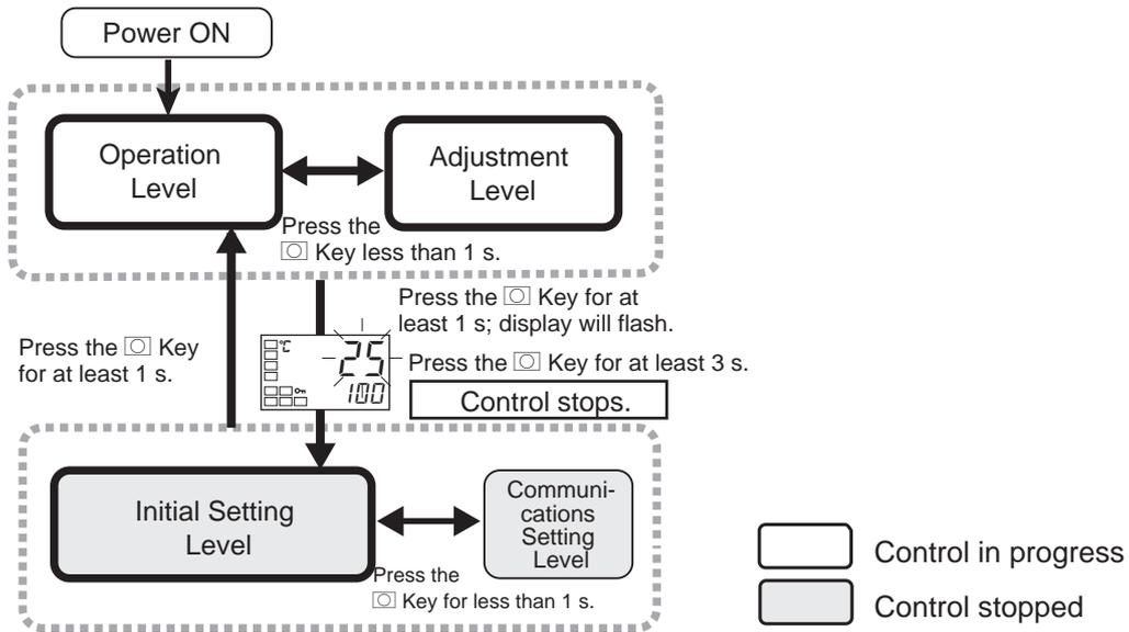
This level is displayed immediately after the power is turned ON. To move to other levels, press the  $\square$  key or the  $\square$  and M keys.
