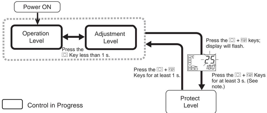
To move from the operation level to the protect level, press O and M keys for three seconds (See note.) or more.
