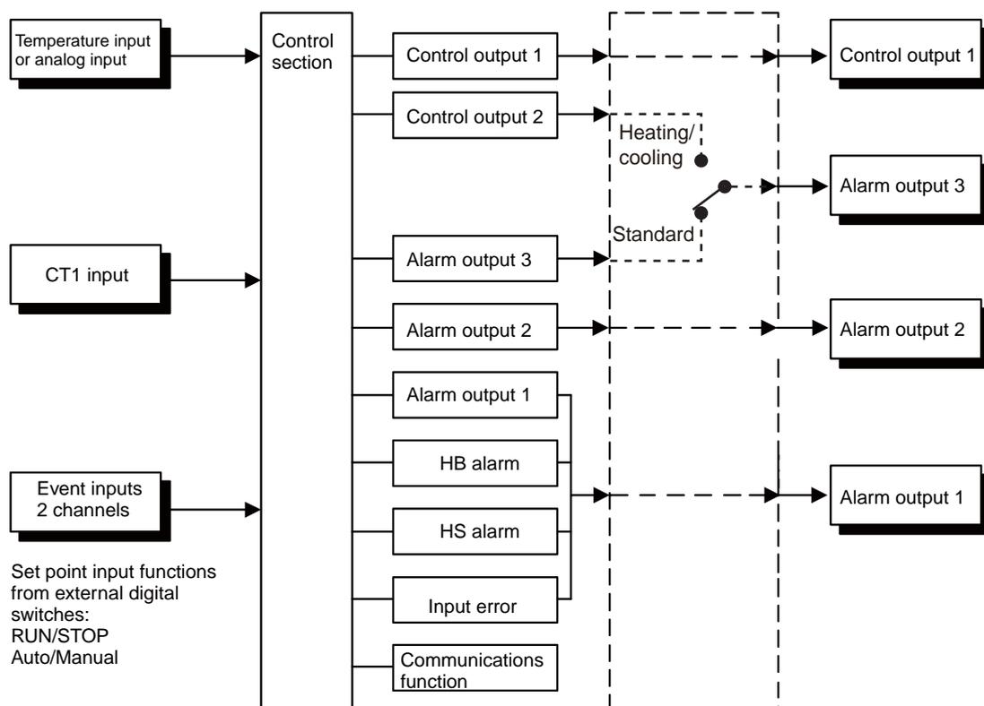
**Note** Functions can be assigned individually for each output by changing the set values for the control output 1 assignment, the alarm output 1 assignment, the
