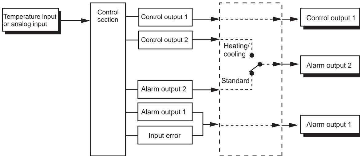
**Note** Functions can be assigned individually for each output by changing the set values for the control output 1 assignment, the alarm output 1 assignment, and the alarm output 2 assignment in the advanced function setting level
