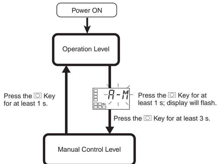
To move from the operation level to the manual control level, press the  $\bigcirc$  key for at least three seconds with the “auto/manual switch” parameter displayed.
