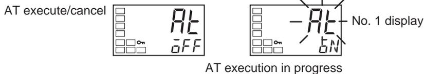
If you move to the operation level during AT execution, the No. 2 display flashes to indicate that AT is being executed.
