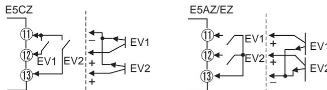
When you are setting two externally input set points, set in the “number of multi-SP uses” parameter.
