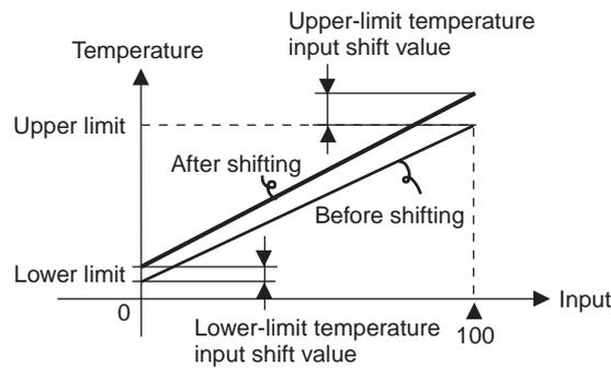
**4-1-2 How to Calculate Input Shift Values for a 2-point Shift**
