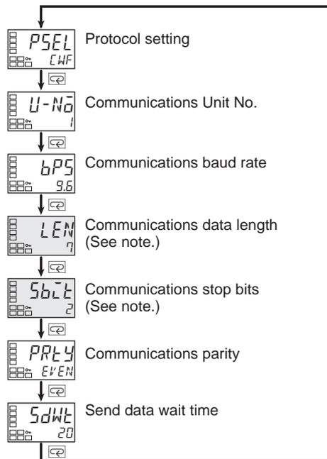
**Note** The “protocol setting” parameter is displayed only when CompoWay/F communications are being used.
