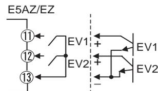
Event input assignments 1 and 2 are as follows according to the setting of the “number of multi-SP uses” parameter:
