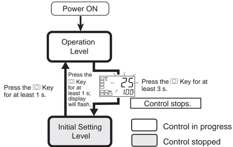
To move from the operation level to the initial setting level, press the  $\square$  key for at least 3 seconds with any parameter displayed except for the “auto/manual switch” parameter.
