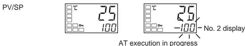
Only the “communications writing,” “RUN/STOP,” and “AT execution/cancel” parameters can be changed during AT execution. Other parameters cannot be changed.
