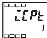
This protect level restricts movement to the initial setting level, communications setting level and advanced function setting level.
