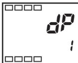
1. Press the key for at least three seconds to move from the “operation level” to the “initial setting level”.
