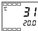
4. To return to the “operation level,” press the key. The process value is 1°C larger than before shift is applied.
