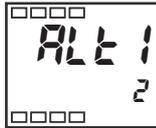
2. Select the “alarm 1 type” parameter by pressing the key. Confirm that the set value is 2. The default value is 2 (Upper-limit alarm).
