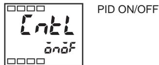
3. Select the “PID ON/OFF” parameter by pressing the key.
