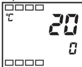
The “operation level” is displayed when the E5AZ/E5EZ is turned ON. The upper display (No.1 display) displays the process value, and the lower display (No.2 display) displays the set point.
