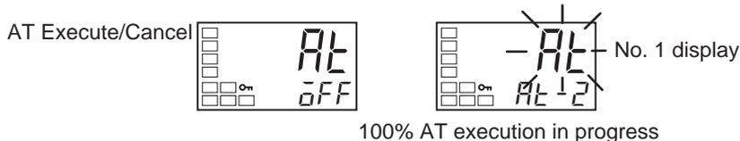
If you move to the operation level during AT execution, the No. 2 display flashes to indicate that AT is being executed.
