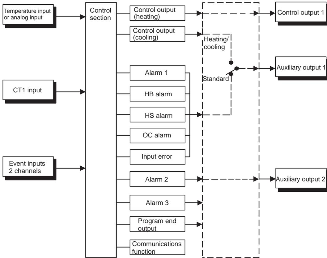
**Note** Functions can be assigned individually for each output by changing the set values for the Control Output 1 Assignment, the Auxiliary Output 1 Assignment, and the Auxiliary Output 2 Assignment parameters in the advanced function setting level.
