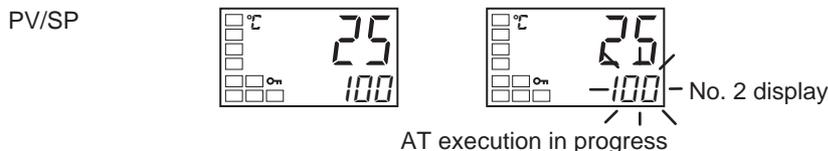
Only the Communications Writing, RUN/STOP, AT Execution/Cancel, and Program Start parameters can be changed during AT execution. Other parameters cannot be changed.
