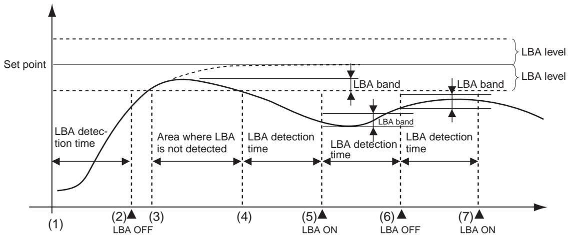
If the control deviation is reduced in the area between 1 and 2 (i.e., the set point is approached) and the amount the control deviation is reduced is at least equal to the LBA band, the loop burnout alarm will remain OFF.
