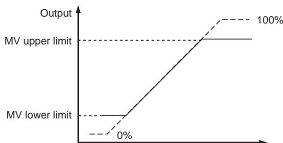
**Note** When the manual MV limit is enabled, the manual MV will be restricted by the MV limit.
