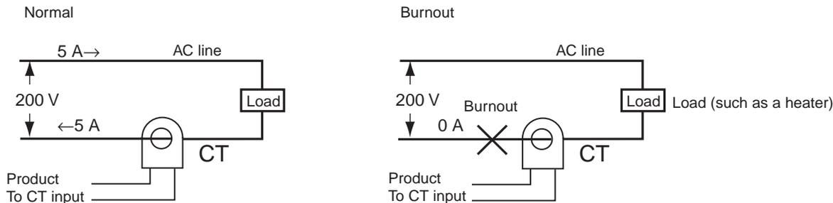
The heater power supply provides 5 A when the current is normal, and 0 A when there is a burnout, so the heater burnout detection current is calculated as follows:
