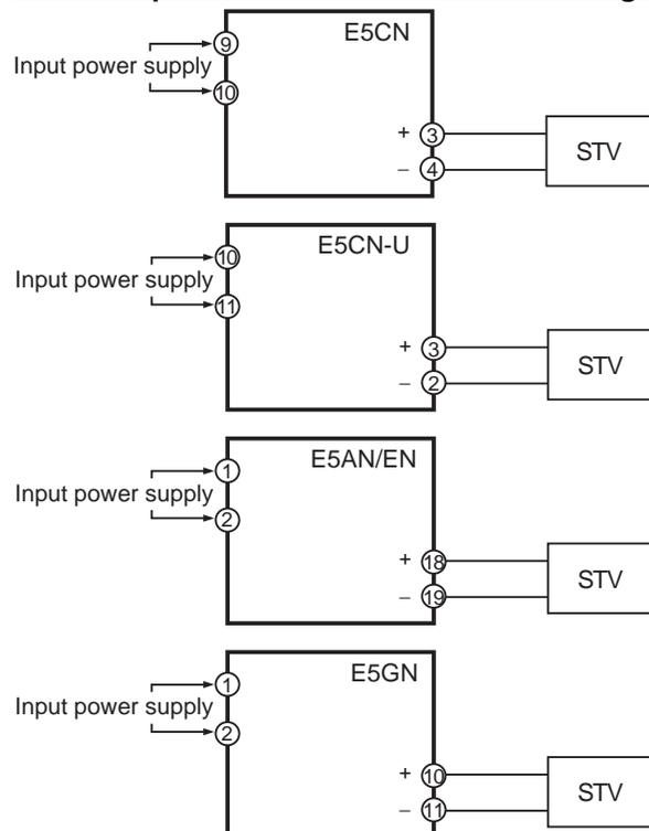
**Voltage Input for a Controller with an Analog Input**
