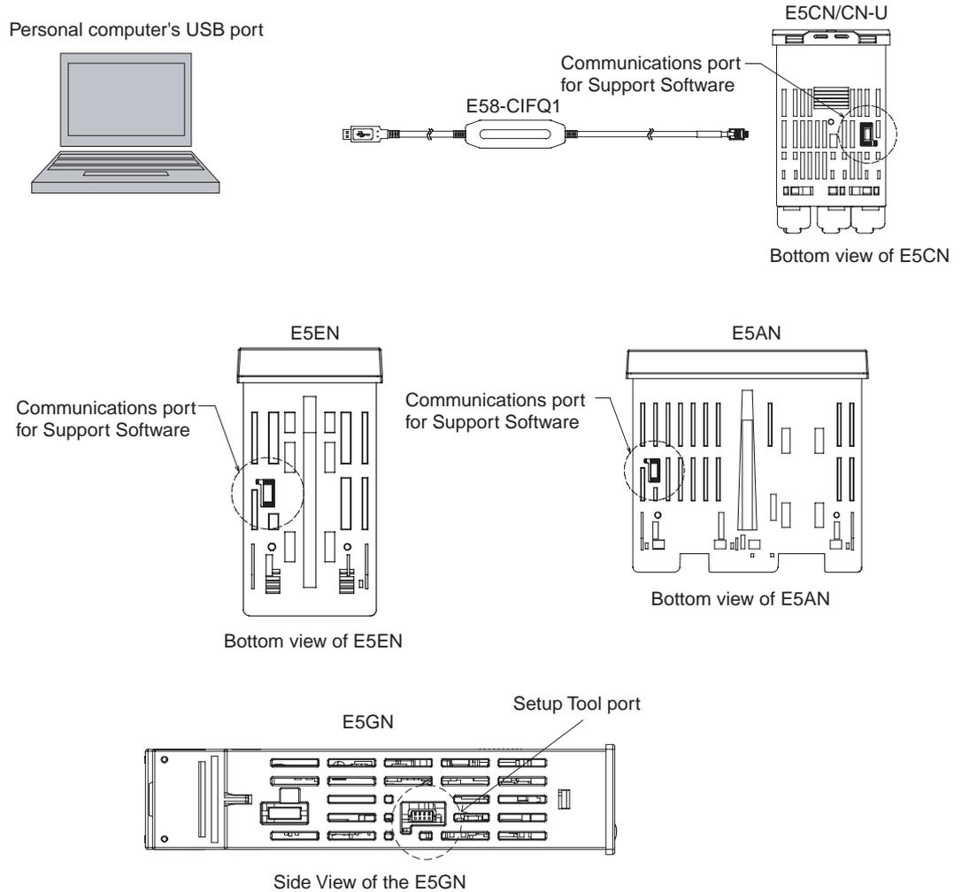
**Note** Hold the connector when inserting or disconnecting the Cable.
