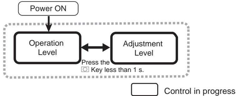
To move to the adjustment level from the operation level, press the  Key once.
