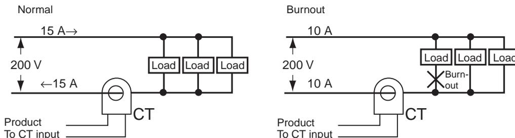
The heater power supply provides 15 A when the current is normal, and 10 A when there is a burnout, so the heater burnout detection current is calculated as follows:
