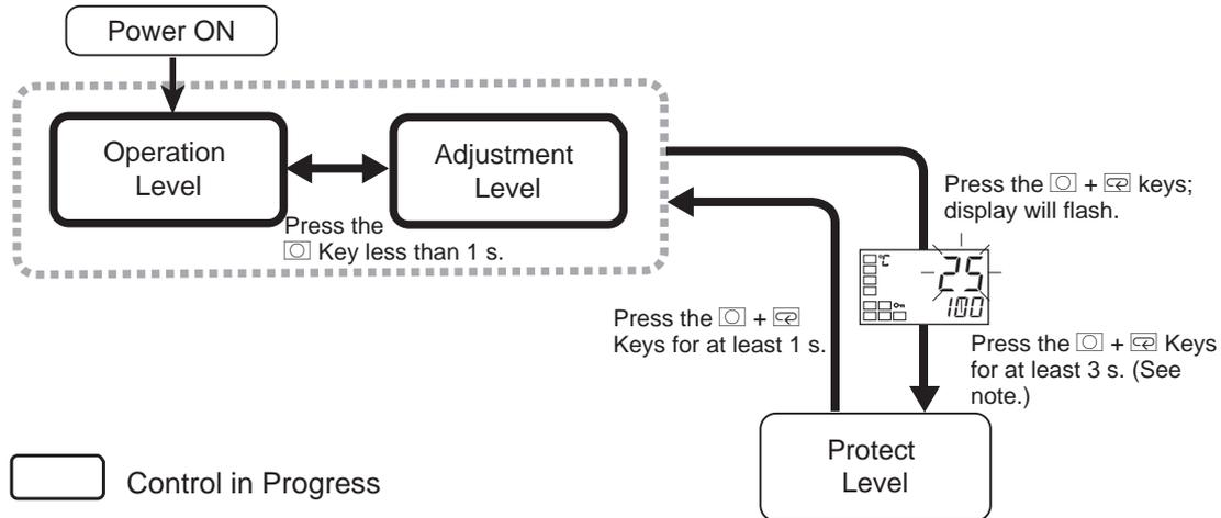
To move from the operation level to the protect level, press  $\square$  and  $\square$  Keys for three seconds (see note) or more.
