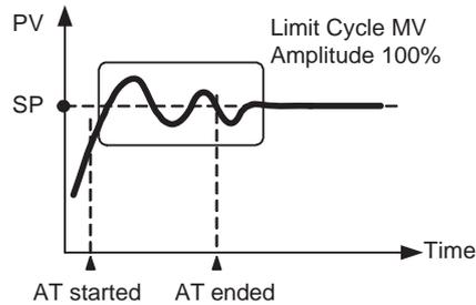
**Note** The Limit Cycle MV Amplitude parameter is disabled.
