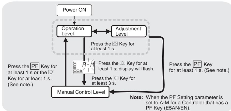
To move from the operation level to the manual control level, press the **□** Key for at least three seconds with the Auto/Manual Switch parameter displayed. In addition, this operation can be performed using the PF Key by setting the PF Key parameter (advanced function setting level) to A-M (Auto/Manual). For details on the setting method, refer to 4-13 Performing Manual Control.
