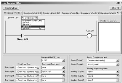
2. The Logic Operation Editor will be displayed. Confirm that the screen for work bit 1 is displayed, and select *Operation 3* from the *Operation Type* Field.
