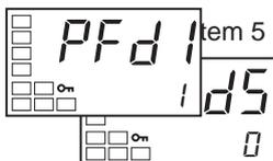
Setting the PF Setting parameter to the Monitor/Setting Item makes it possible to display monitor/setting items using the function key. The following table shows the details of the settings. For setting (monitor) ranges, refer to the applicable parameter.
