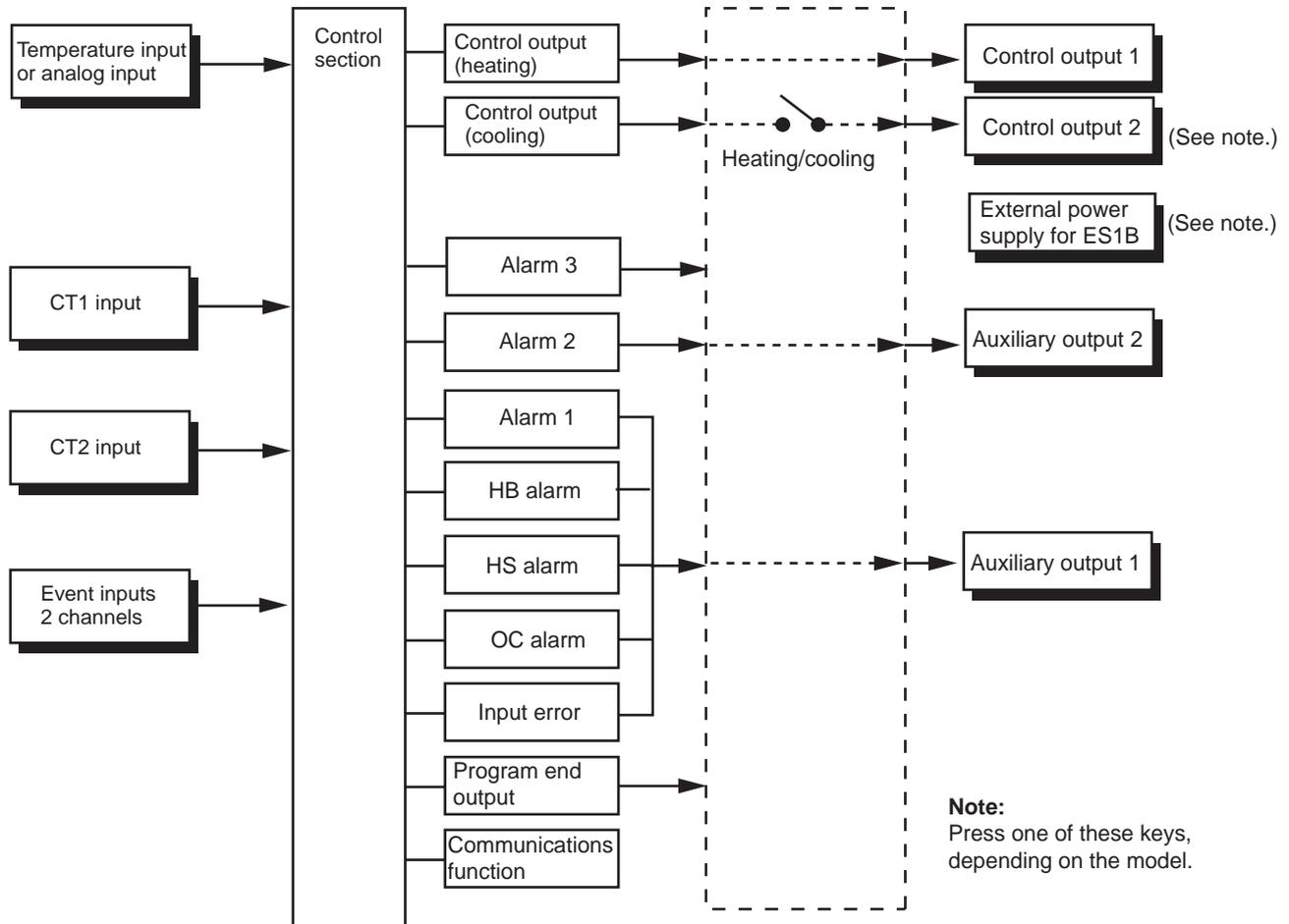
**Note** Functions can be assigned individually for each output by changing the set values for the Control Output 1 Assignment, the Control Output 2 Assignment, the Auxiliary Output 1 Assignment, and the Auxiliary Output 2 Assignment parameters in the advanced function setting level.
