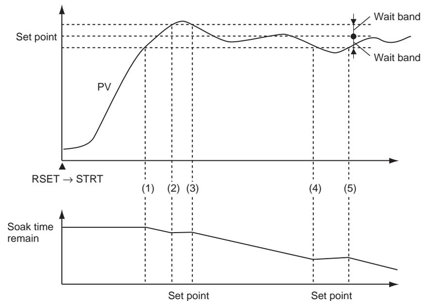
The wait band is the band within which the process value is stable in respect to the set point. The soak time is measured within the wait band. The timer that measures the soak time operates only when the process value is within the wait band around the set point (i.e.,  $SP \pm \text{wait band}$ ). In the following diagram, the timer will be stopped between the start and (1), (2) and (3), and (4) and (5) and will measure the time only between (1) and (2), (3) and (4), and (5) and the end.
