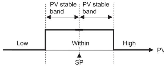
The default is 5.0 (°C/°F) for Controllers with Thermocouple/Resistance Thermometer Universal Inputs and 5.00% FS for Controllers with Analog Inputs.
