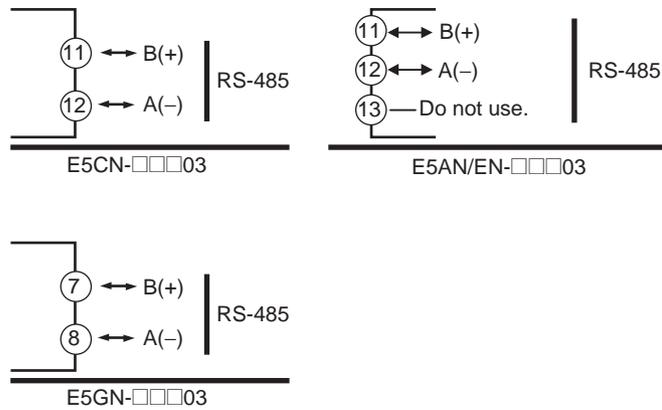
Specify both ends of the transmission path including the host computer as end nodes (that is, connect terminators to both ends).
