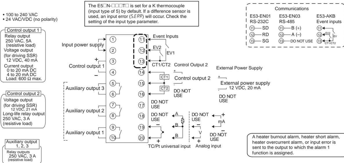
Since the voltage output (control output) is not electrically insulated from the internal wiring, one or other of the control output terminals must be left unearthed when using an earthed thermocouple thermometer. (Connection makes measurements unreliable due to sneak currents.)
