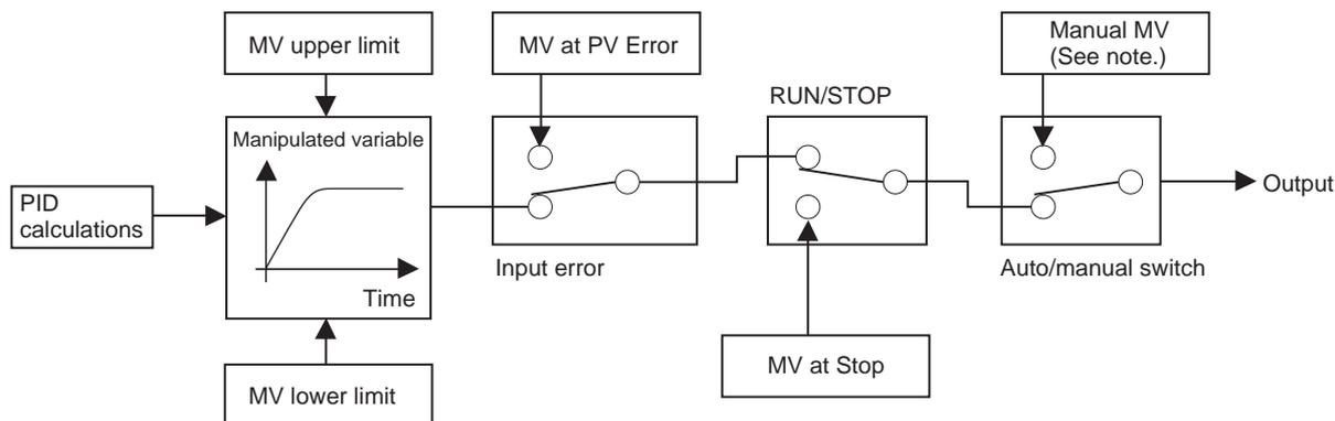
**Note** When the Manual MV Limit Enable parameter is set to ON, the setting range will be the MV lower limit to the MV upper limit.
