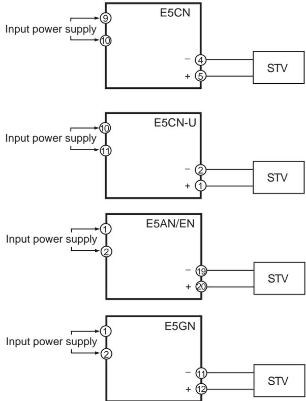
**Current Input for a Controller with an Analog Input**
