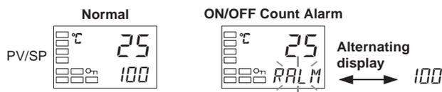
**Control Output ON/OFF Count Alarm Function**
