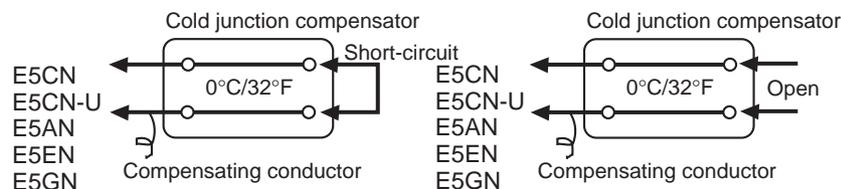
In this example, calibration is shown for a Controller with a Thermocouple/Resistance Thermometer Universal Input, with thermocouple/infrared temperature sensor set as the input type.
