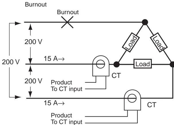
Current when there is a burnout =  $10 \text{ A} \times \sqrt{3} \times (\sqrt{3}/2) = 15 \text{ A}$
