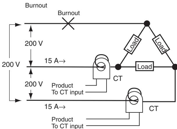
Current when there is a burnout =  $10 \text{ A} \times \sqrt{3} \times (\sqrt{3}/2) = 15 \text{ A}$
