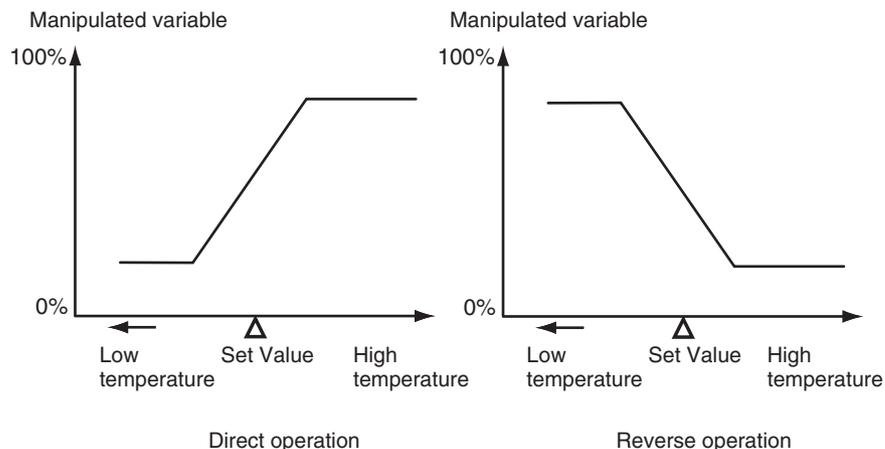
For example, when the process value (PV) is lower than the set point (SP) in a heating control system, the manipulated variable increases according to the difference between the PV and SP. Accordingly, reverse operation is used in a heating control system. Direct operation is used in a cooling control system, in which the operation is the opposite of a heating control system.
