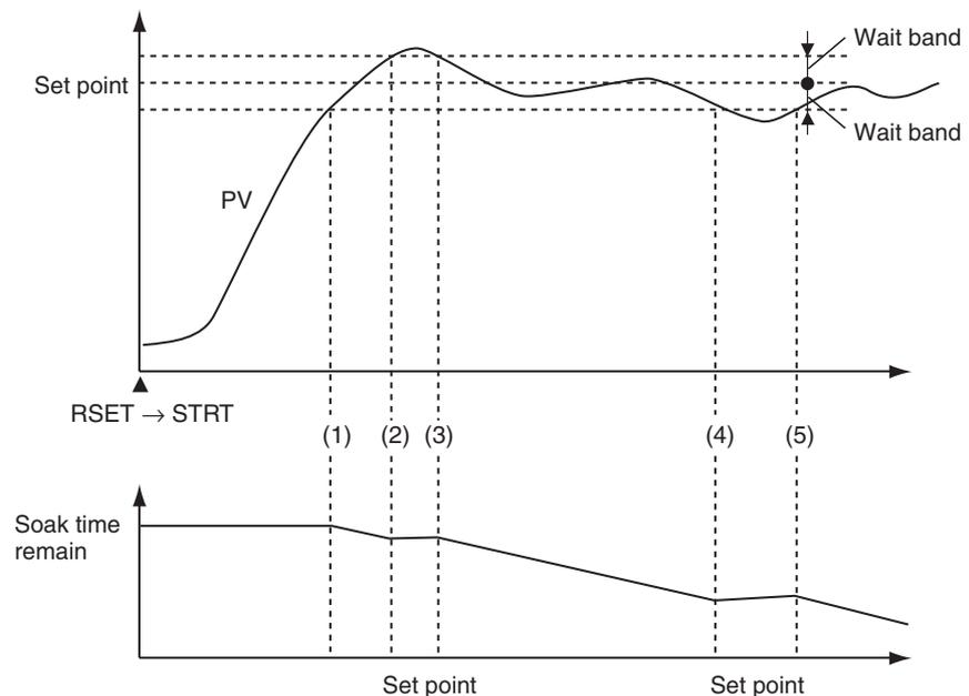
The wait band is the fixed band within which the process value is stable in respect to the set point. The soak time is measured within the wait band. The timer that measures the soak time operates only when the process value is within the wait band around the set point (i.e.,  $SP \pm \text{wait band}$ ). In the following diagram, the timer will be stopped between the start and (1), (2) and (3), and (4) and (5) and will measure the time only between (1) and (2), (3) and (4), and (5) and the end.
