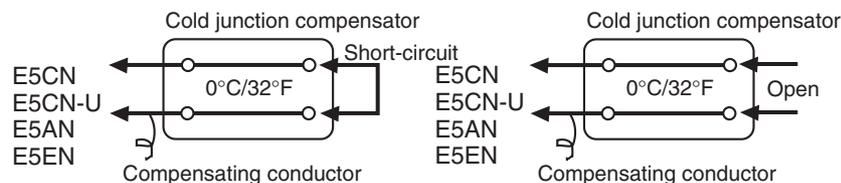
In this example, calibration is shown for a Controller with a Thermocouple/Resistance Thermometer Multi-input, with thermocouple/infrared temperature sensor set as the input type.
