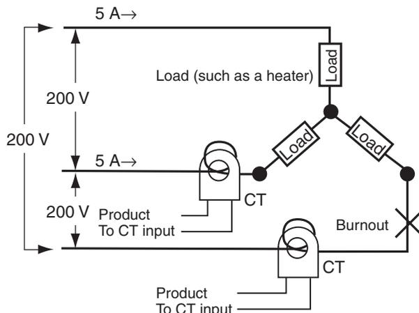
$$\text{Current when there is a burnout} = 10 \text{ A} \times (1/\sqrt{3}) \times (\sqrt{3}/2) = 5 \text{ A}$$
