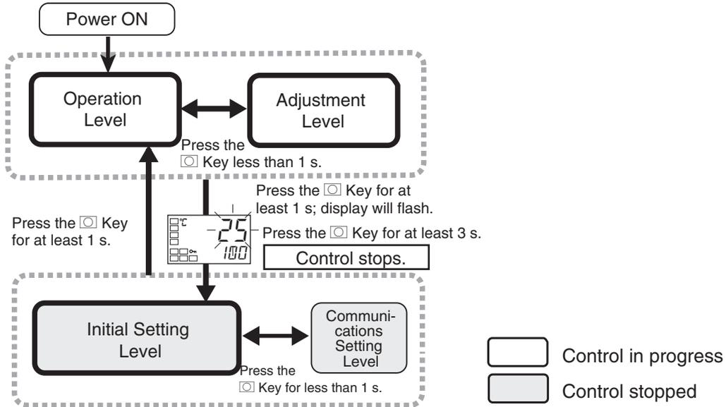
This level is displayed immediately after the power is turned ON.
