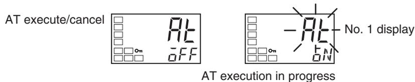
If you move to the operation level during AT execution, the No. 2 display flashes to indicate that AT is being executed.
