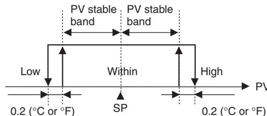
When analog inputs are used: 0.02 (%FS)
