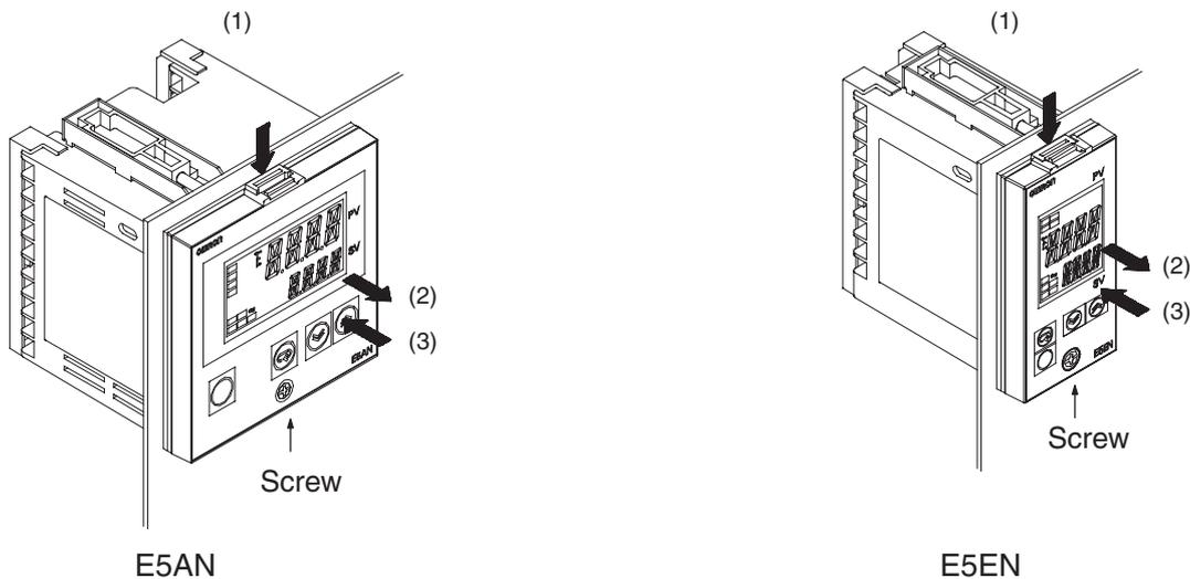
Prepare a Phillips screwdriver suitable for the screw on the front panel to remove the Temperature Controller.
