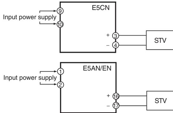
**Voltage Input for a Controller with an Analog Input**
