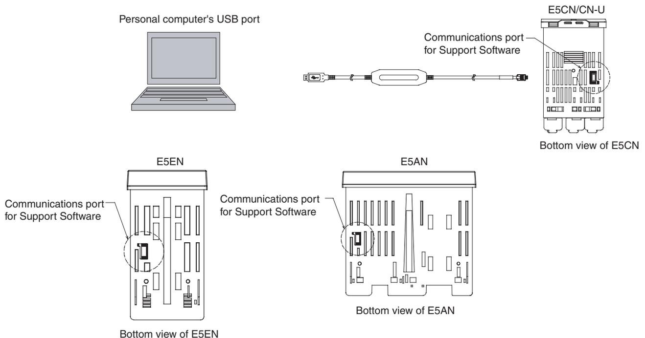
**Note** Hold the connector when inserting or disconnecting the Cable.
