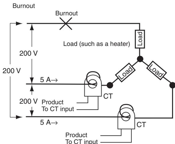
$$\text{Current when there is a burnout} = 10 \text{ A} \times (1/\sqrt{3}) \times (\sqrt{3}/2) = 5 \text{ A}$$
