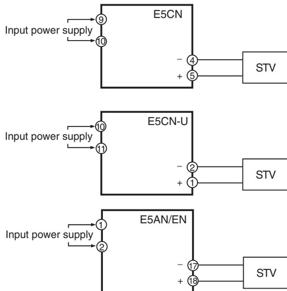
**Current Input for a Controller with an Analog Input**
