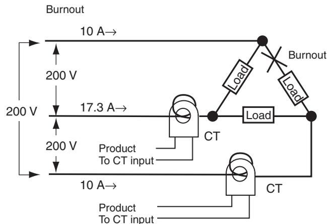
Current when there is a burnout =  $10 \text{ A} \times \sqrt{3} \times (1/\sqrt{3}) = 10 \text{ A}$
