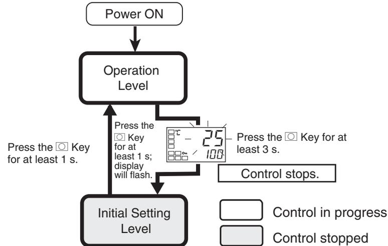
To move from the operation level to the initial setting level, press the  key for at least three seconds with any parameter displayed except for the “auto/manual switch” parameter.
