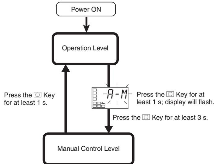
To move from the operation level to the manual control level, press the [Key] key for at least three seconds with the “auto/manual switch” parameter displayed.
