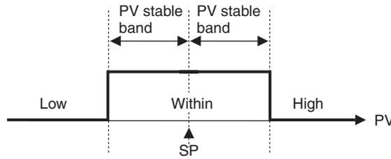
The default is 5.0 (°C/°F) for Controllers with Thermocouple/Resistance Thermometer Multi-Inputs and 5.0% FS for Controllers with Analog Inputs.
