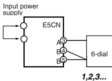
This example describes how to calibrate the E5CN when it is connected to a platinum resistance thermometer.
