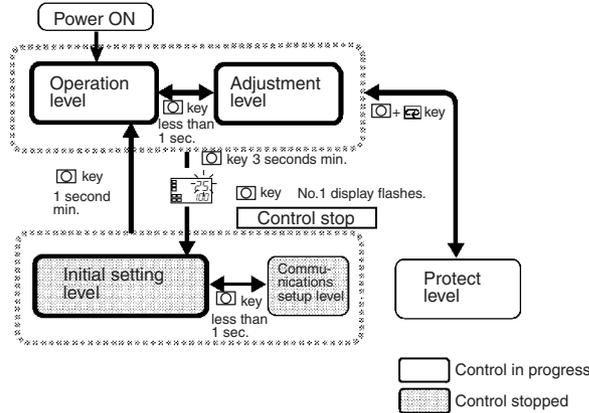
To move to the adjustment level from the operation level, press the key for less than one second.
