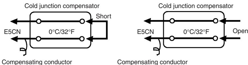
This example describes how to calibrate the E5CN when thermocouple input is currently selected on an E5CN supporting thermocouple input.
