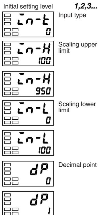
1. Press the key for at least three seconds to move from the “operation level” to the “initial setting level”.
