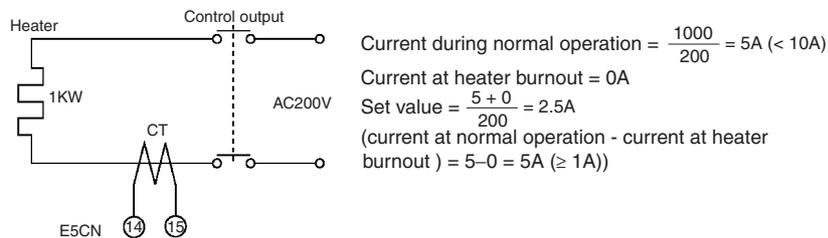
Example 2 When using three 200 VAC, 1 kW heaters
