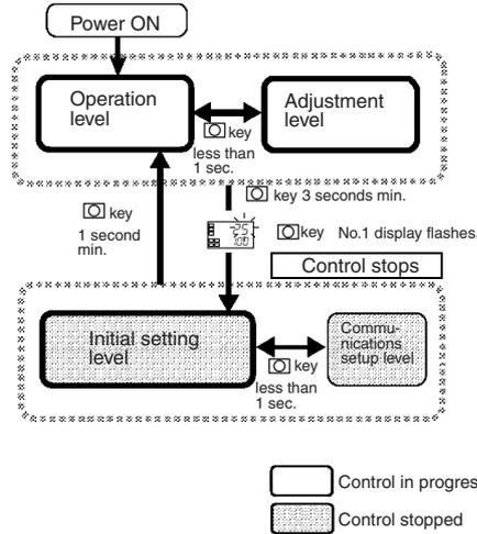
To move from the operation level to the initial setting level, press ○ key for three seconds or more.
