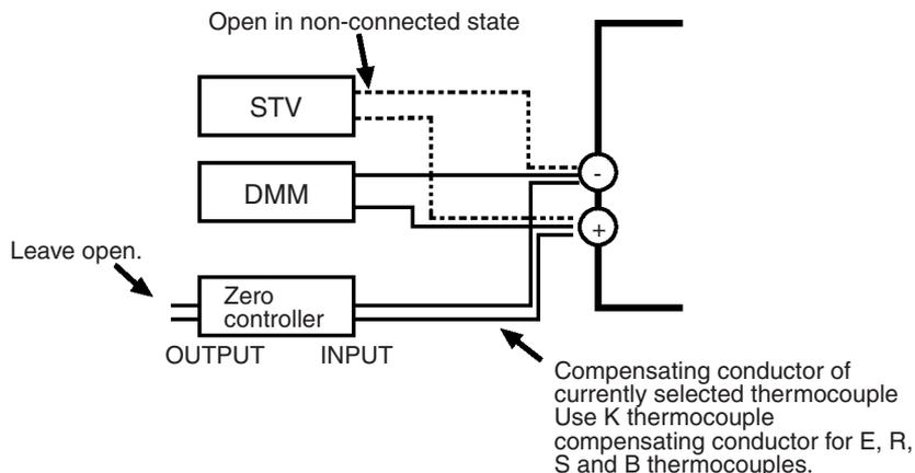
Disconnect the STV to enable the thermocouple of the cold junction compensator. When doing this, be sure to disconnect the wiring on the STV side.
