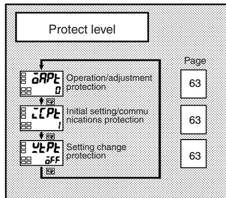
The settings of protected parameters are not displayed and so cannot be modified.
