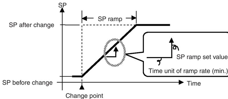
The change rate during SP ramp is specified by the “SP ramp set value” parameter. The “SP ramp set value” default is “OFF”, and the SP ramp function is disabled.
