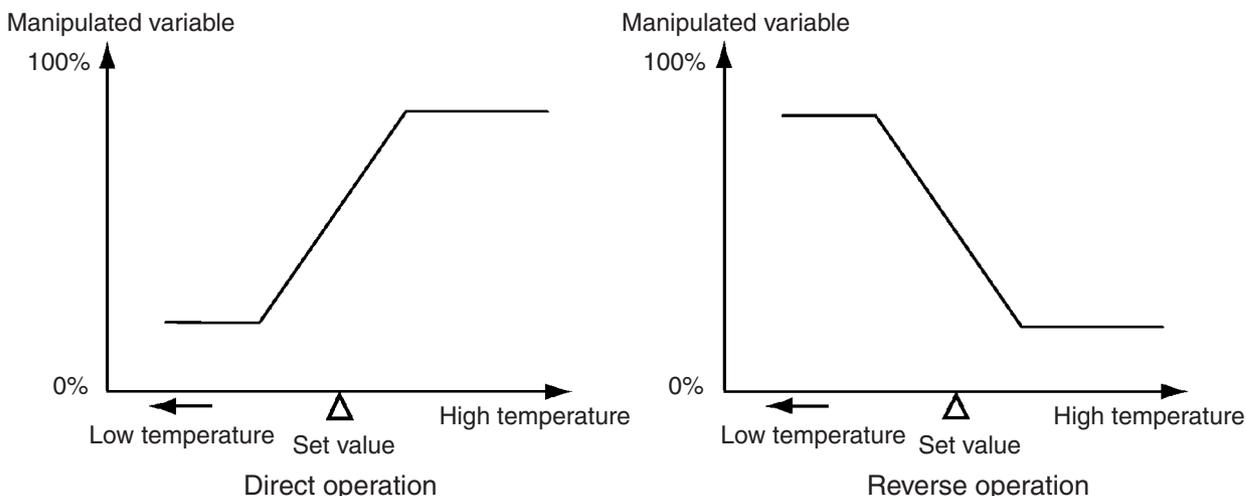
For example, when the process value (PV) (temperature) is lower than the set point (SP) (temperature) in a heating control system, the manipulated variable increases by the difference between the PV and SP values. Accordingly, this becomes “reverse operation” in a heating control system, or alternatively, “direct operation” in a cooling control system.
