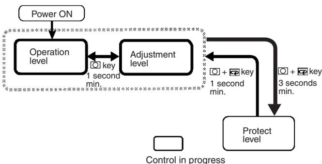
To move from the operation Level to the protect level, press the and keys for at least three seconds.
