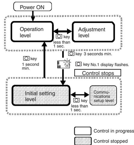
This level is automatically displayed immediately after the E5CN is turned ON. To move to other levels, press the key or the and keys.
