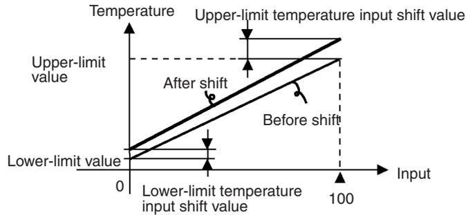
4-1-2 How to calculate input shift values (2-point shift)
