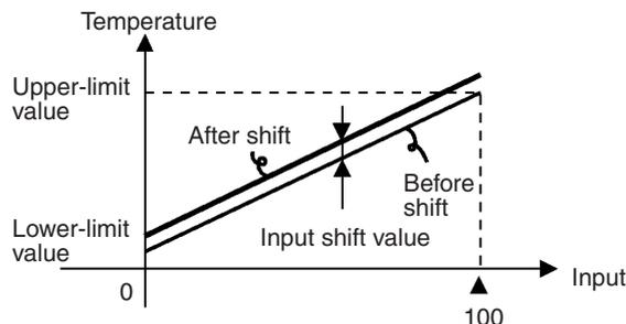
In this example, let's shift the input of the K sensor by “1°C” by 1-point input shift.
