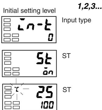
1. Press the key for at least three seconds to move from the “operation level” to the “initial setting level”.
