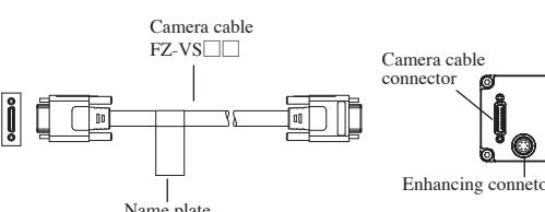
\* The camera cable FZ-VS□□ has polarity. Be sure to connect the side with the name plate on it to the controller.
