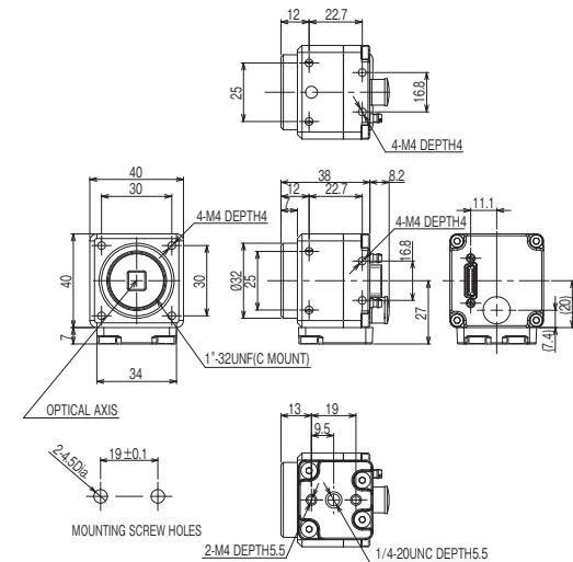
\* The base at the bottom of the camera can be mounted to the bottom, top, and both sides. Remove the base mounting screw (M4x8) and correct the mounting position. (Recommended mounting screw torque: 1.2 N·m)
