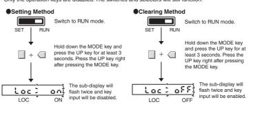
If a key is pressed while key operations are locked. "LOC" will flash E Loci twice on the display to indicate that key operations have been disabled.
