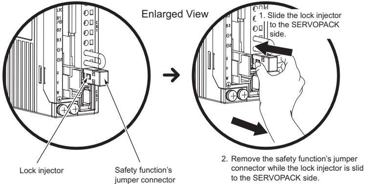
Note: The safety function's jumper connector may be damaged if removed while the lock is still on.
