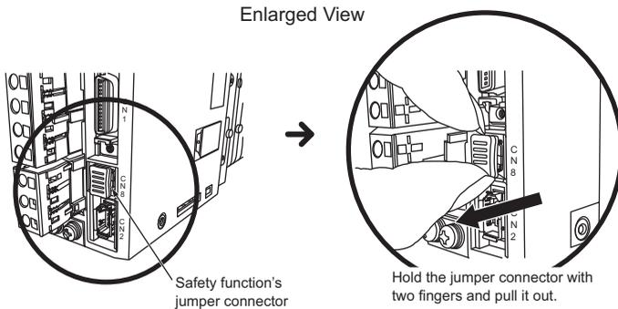
**3. Connect a safety function device to CN8.**
