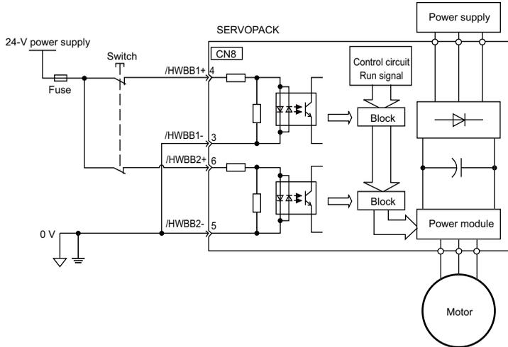
Note: For safety function signal connections, the input signal is the 0V common and the output signal is the source output. This is opposite to other signals described in this manual. To avoid confusion, the ON and OFF status of signals for safety functions are defined as follows:
