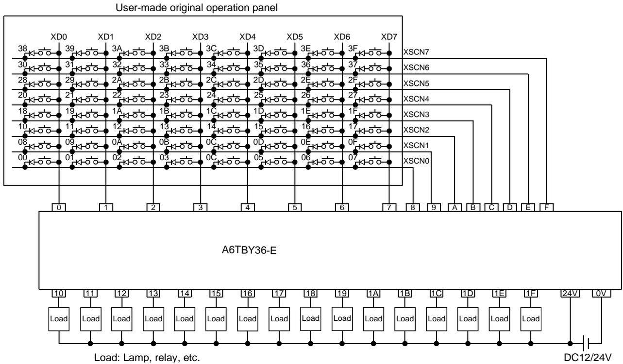
(b) For use of A6TB54-E type connector terminal block conversion unit
