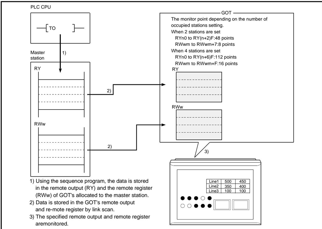
Monitor (write from GOT) for remote input and remote register (read area)
