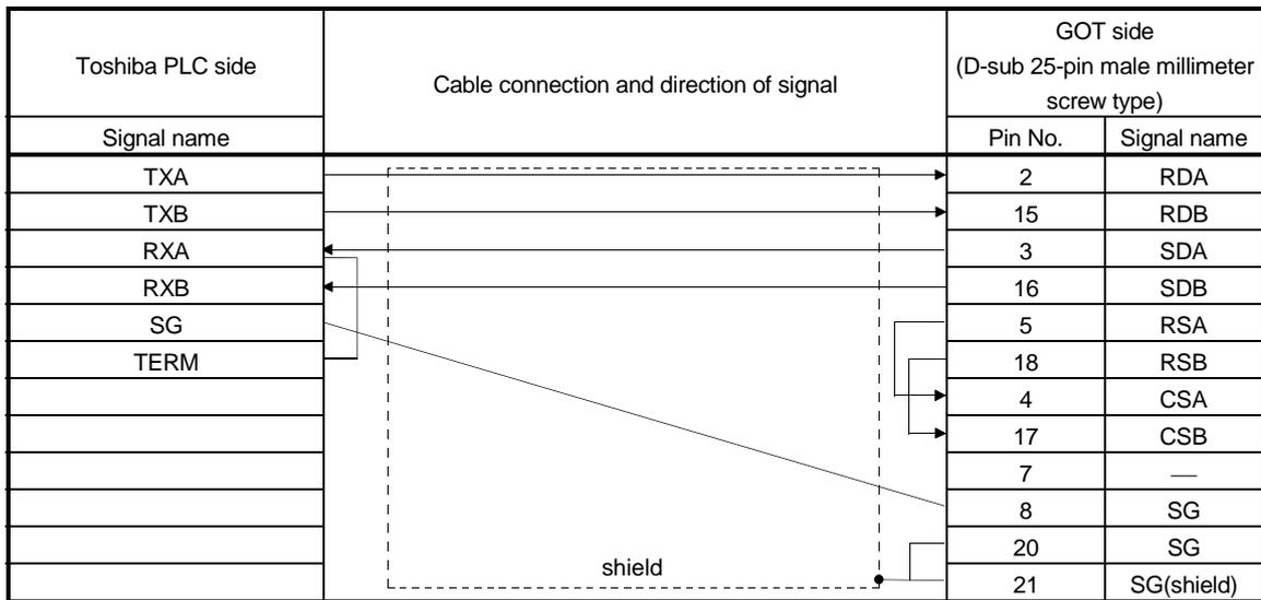
\*1.RXA and TERM on the Toshiba PLC side must be shorted. (Connect to the terminator resistor.)
