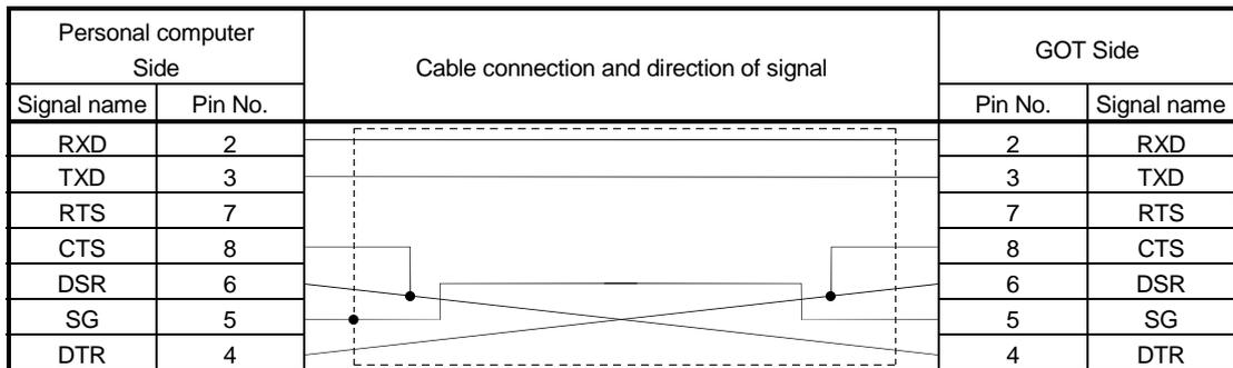
(c) Connection diagram of AC30N2A
