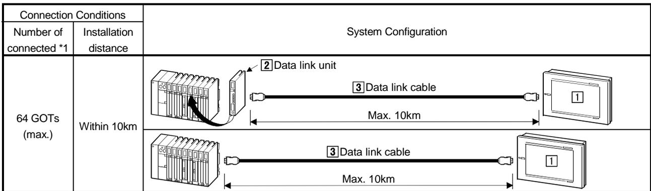
\*1 The number of GOTs connectable is up to the number of connectable stations in the corresponding data link system.
