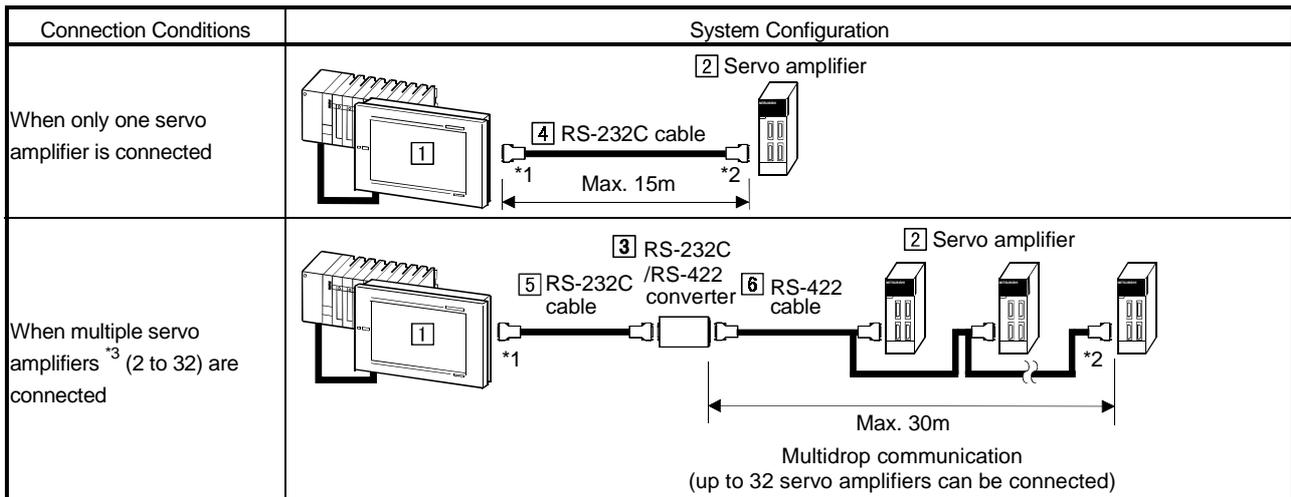
\*1 Connect the GOT side connector of the cable to the RS-232C interface at the bottom of the GOT used for downloading the monitor screen data.
