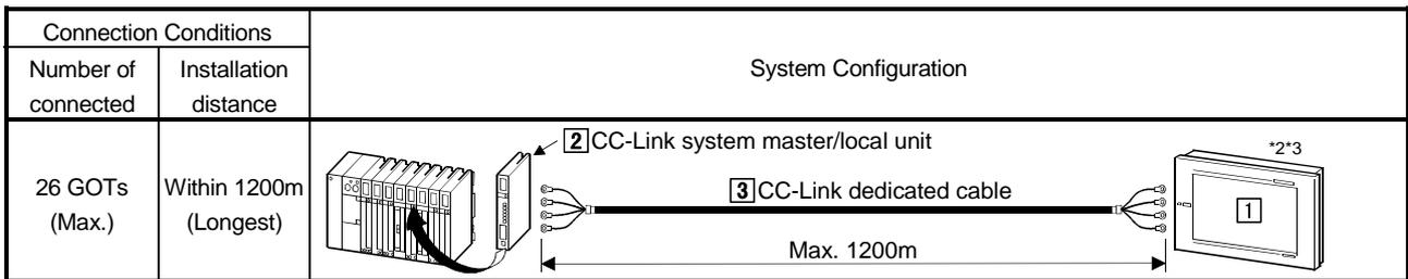
\*1 The number of connected GOTs varies with the configuration of the CC-Link system, and the installation distance (maximum transmission distance) varies with the transmission speed of the CC-Link system.
