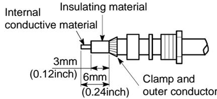
4) Solder the contact to the tip of the internal conductive material.
