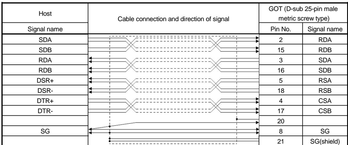
DSR signal ... If this signal is OFF, data is not transmitted from the GOT to the host.
