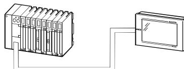
The network module (remote I/O module) on the remote I/O station of the MELSECNET/H network system and GOT can also be connected by the RS-232C cable. (Refer to Section 2.3.6 for connection to the remote I/O station of the MELSECNET/H network system.)
