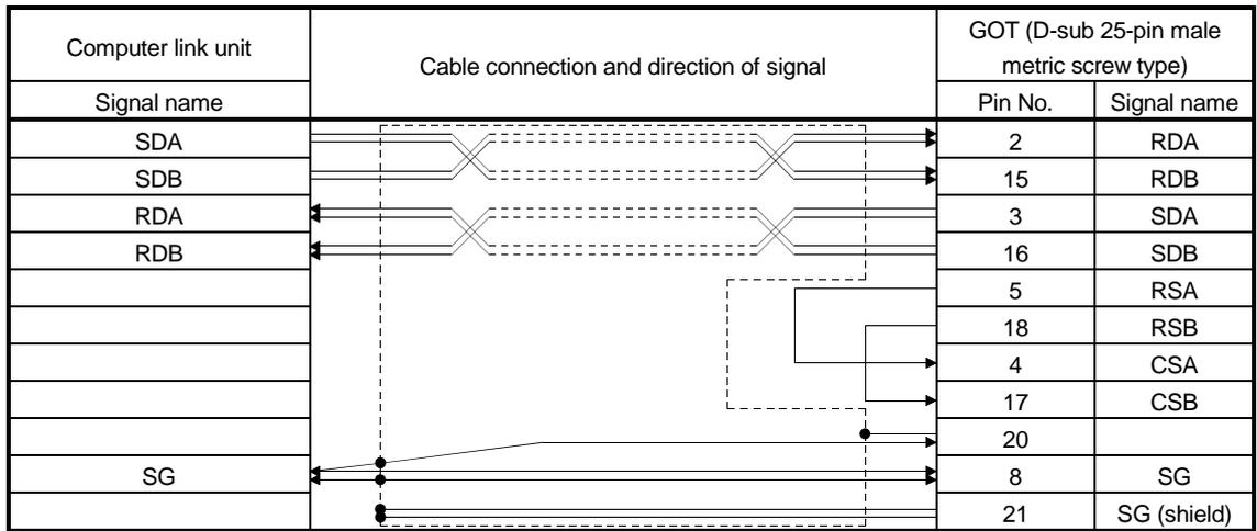
(b) Connector, crimp terminal and cable
