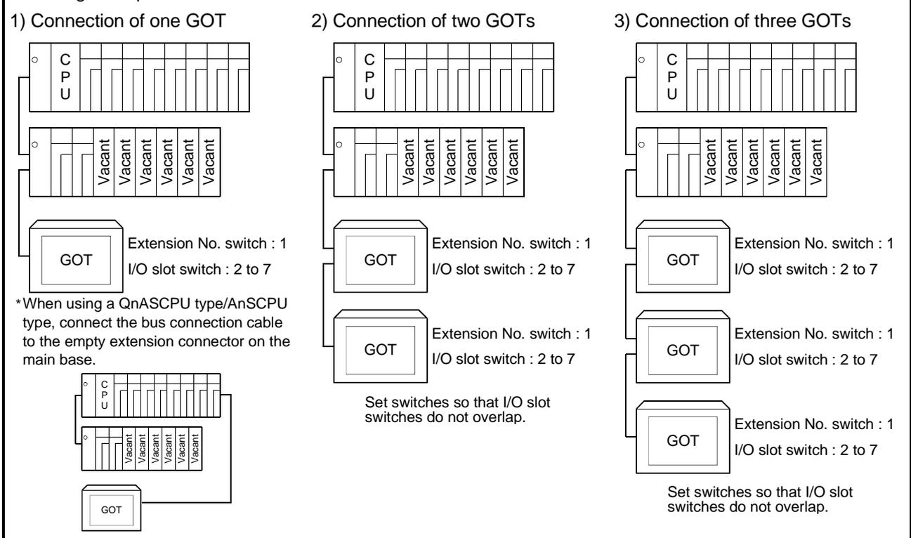
(3) Setting method used when there are no empty slots on the extension base unit connected
