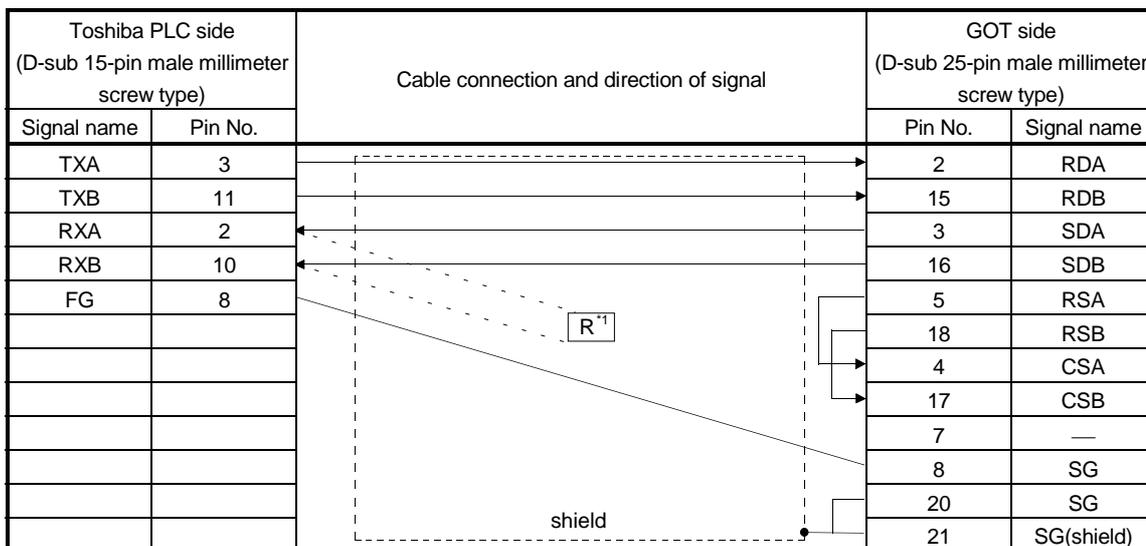
\*1 A 1/2W-120Ω resistor must be connected between RXA and RXB on the Toshiba PLC side.
