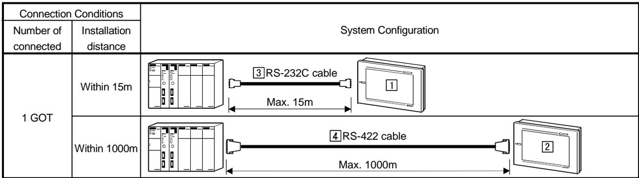
\*1 RS232C communication can be made with the T2E and T2N only.
