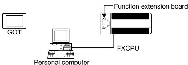
\*7 The function extended board used depends on the type of the FXCPU connected. Use the compatible function extended board given in the following table.
