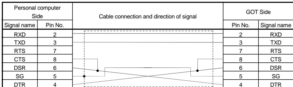
(c) Connection diagram of AC30N2A
