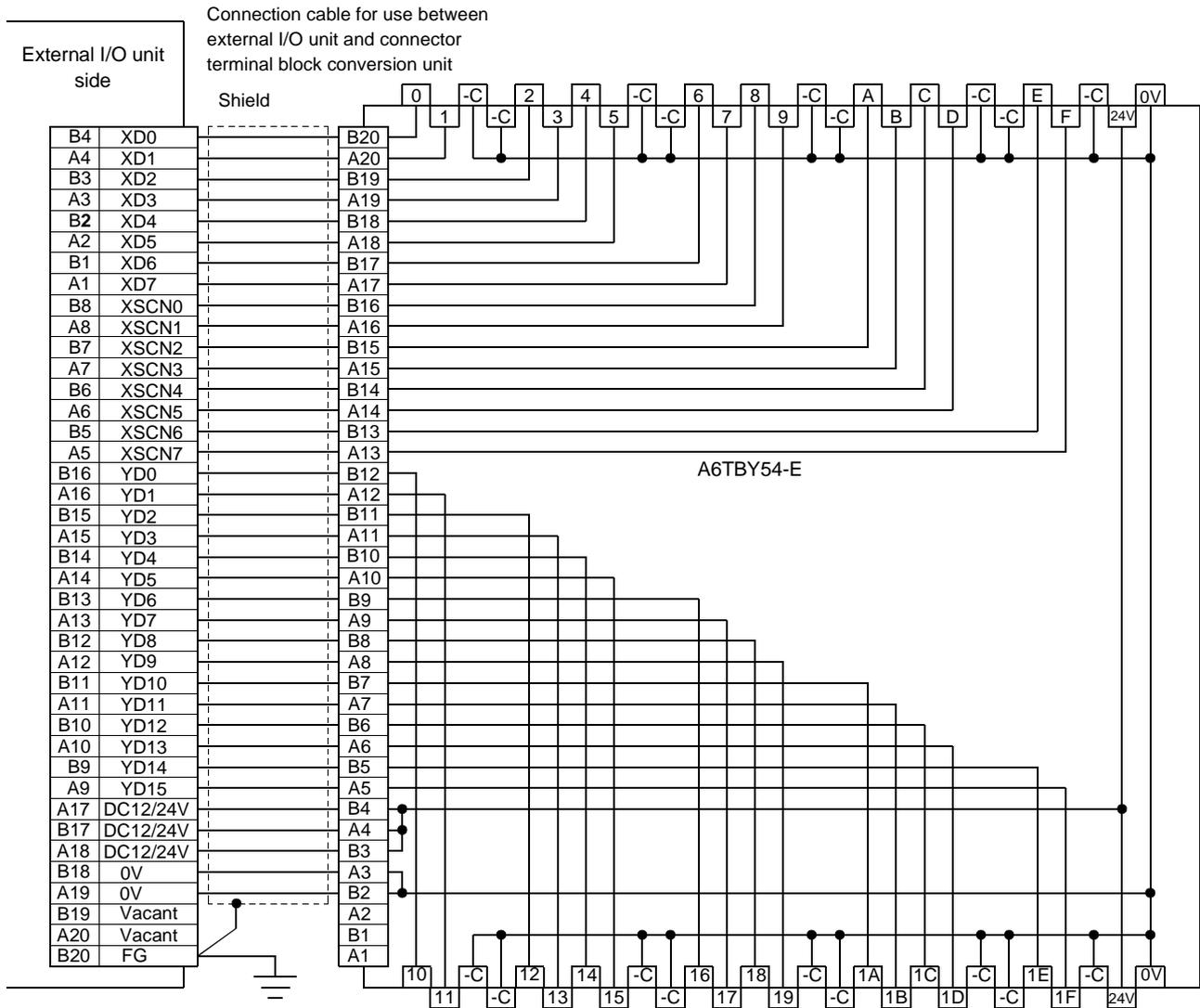
(2) Wiring diagram for use between connector terminal block conversion unit and user-made original operation panel
