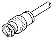
\*1 Soldered part must not have excess solder mound.
