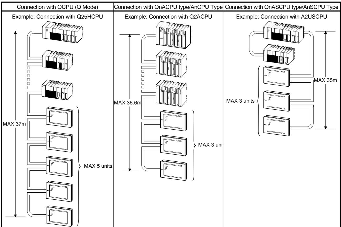
\*There are various precautions for bus connection according to the system selected. For details, refer to Chapter 3.
