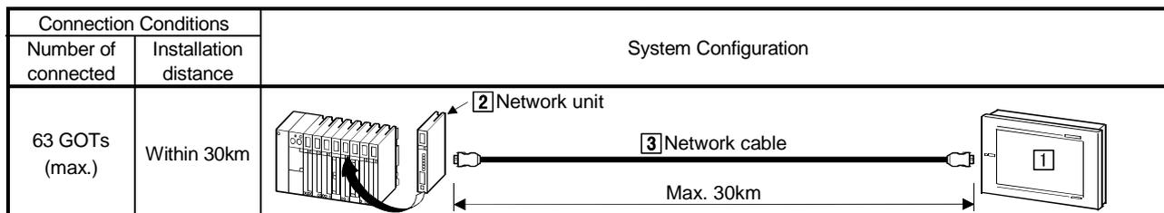
\*1 The number of GOTs connectable is up to the number of connectable stations in the corresponding network system.
