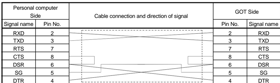
(d) When using the software (DOS version) for motion controller CPU (A series)
