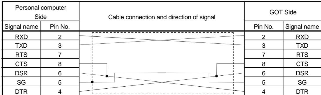
(b) Connection diagram of AC30R2-9P, F2-232CAB-1
