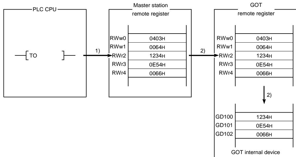
1) Store the continuous write command data in the master station's remote register (RWw).
