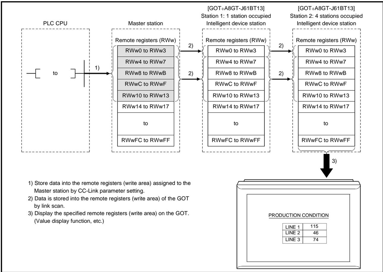
8.2.2 I/O signals transfered to/from the master module
