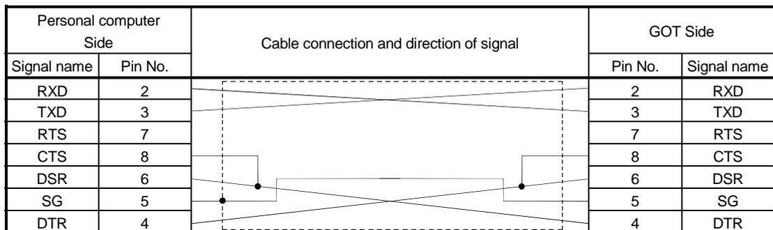
(b) Connection diagram of AC30R2-9P, F2-232CAB-1
