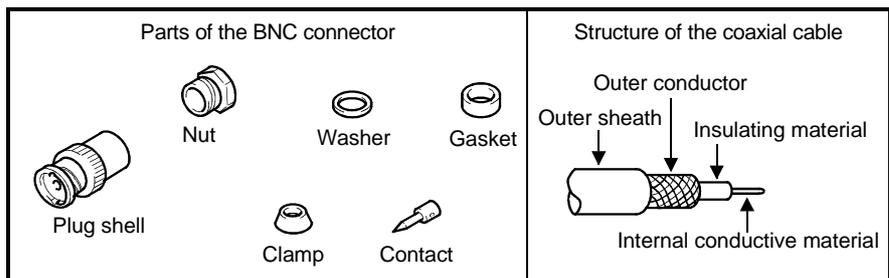
(b) Connecting the BNC connector with the coaxial cable
