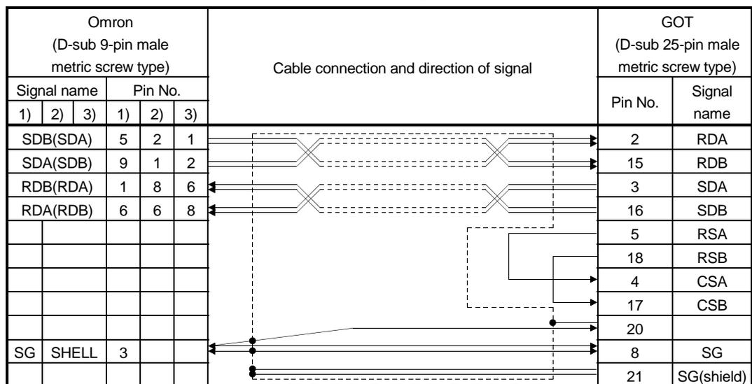
3) CPU (CV500, CV1000, CV2000, CVM1-CPU01, CVM1-CPU11, CVM1-CPU21)
