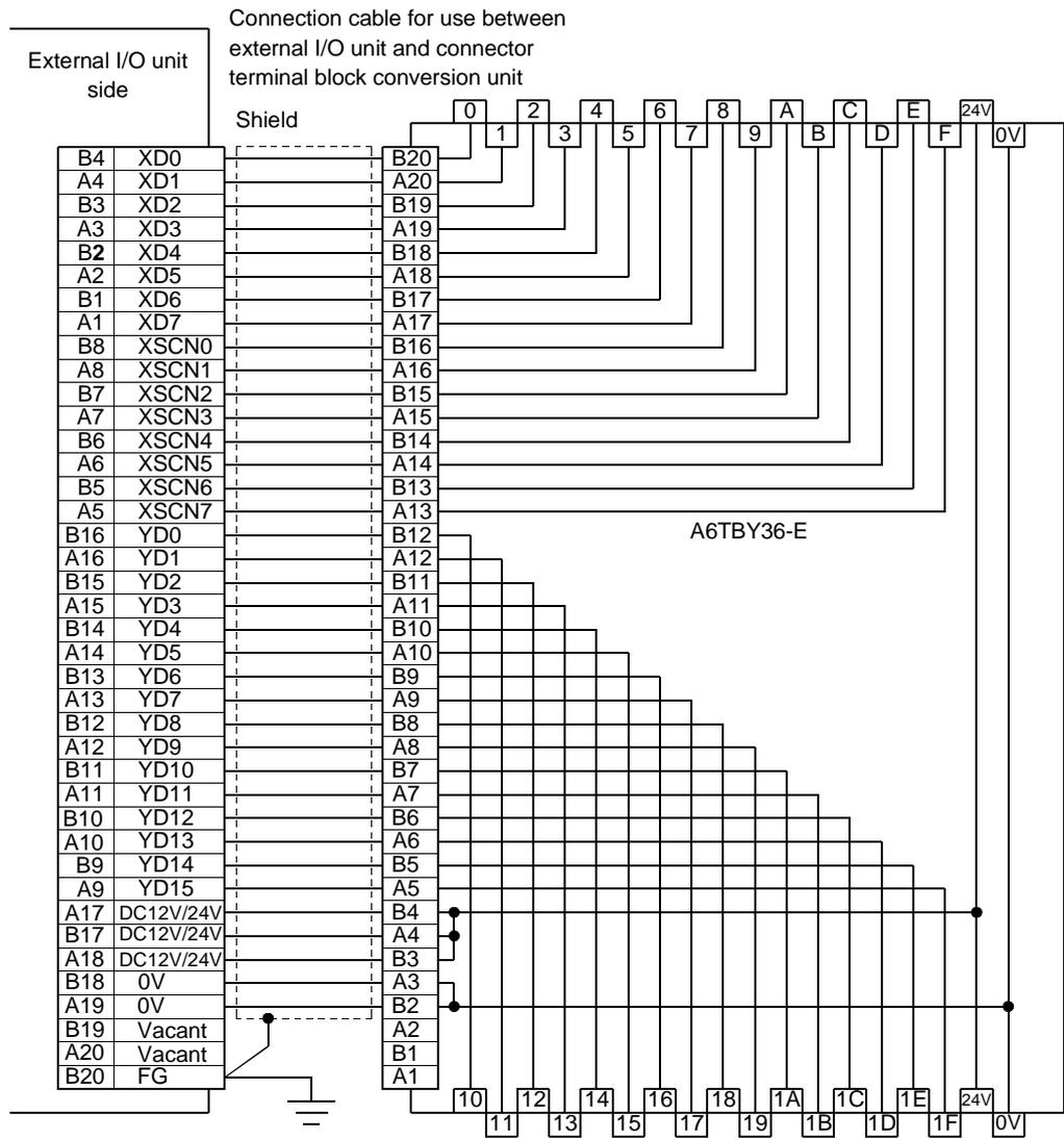
(b) For use of A6TBY54-E type connector terminal block conversion unit
