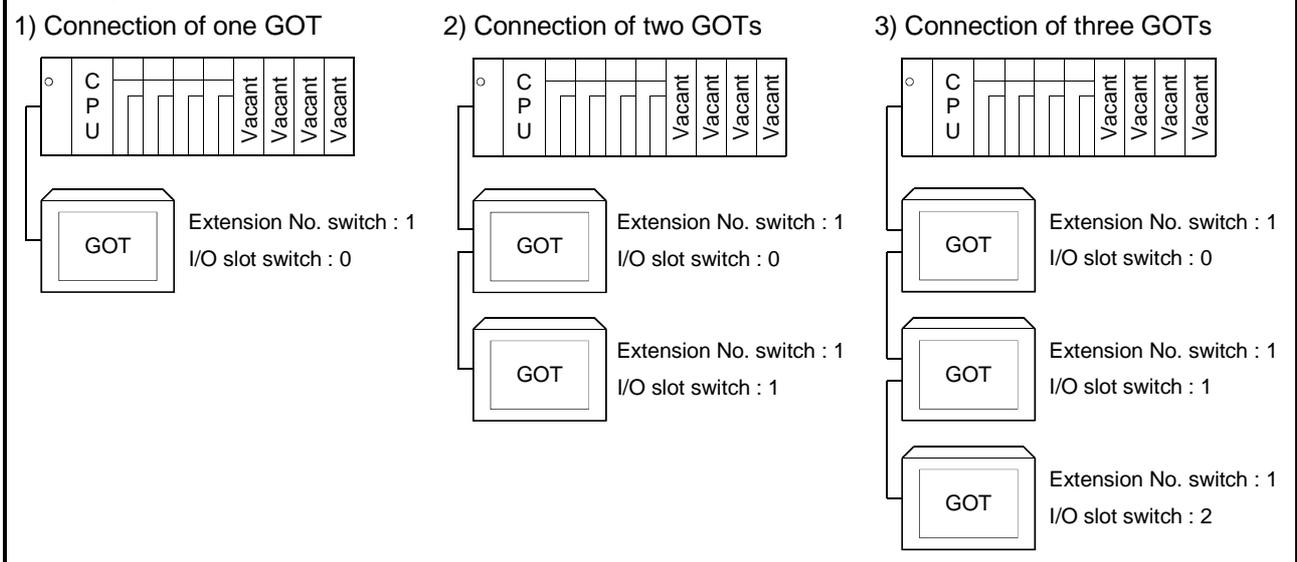
(2) Setting method used for assignment of GOT(s) to empty slot(s) of extension base unit
