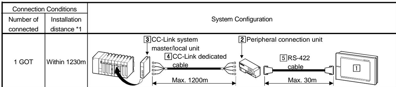
\*1 The installation distance (maximum transmission distance) varies with the transmission speed of the CC-Link system. For details, refer to the CC-Link System Master/Local Unit User's Manual (Details).
