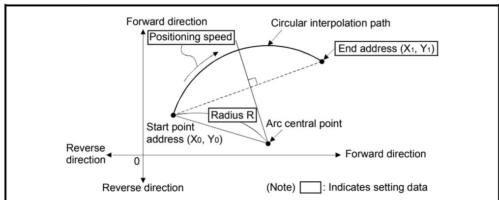
Fig.6.13 Circular interpolation control using absolute data method
