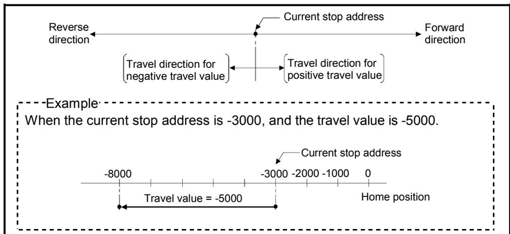
Fig.6.2 Positioning using incremental data method
