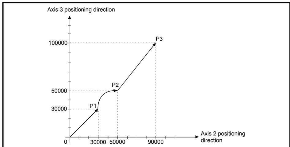
Fig.6.30 Positioning for Axis 2 and Axis 3
