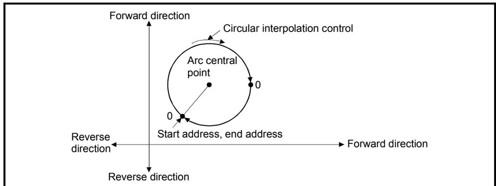
Fig.6.21 Positioning control of a complete round
