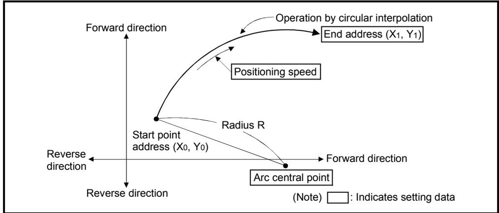
Fig.6.17 Circular interpolation control using absolute date method
