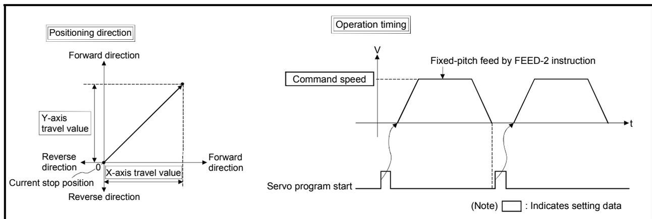
Fig.6.24 Fixed-pitch feed control using 2 axes linear interpolation
