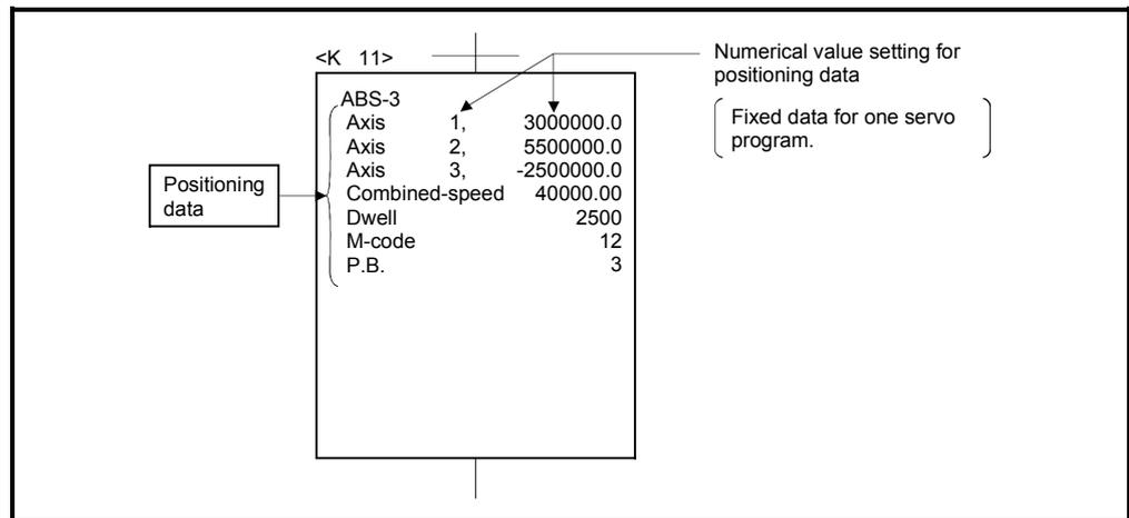
Fig. 5.3 Setting example of positioning data by specifying numerical value
