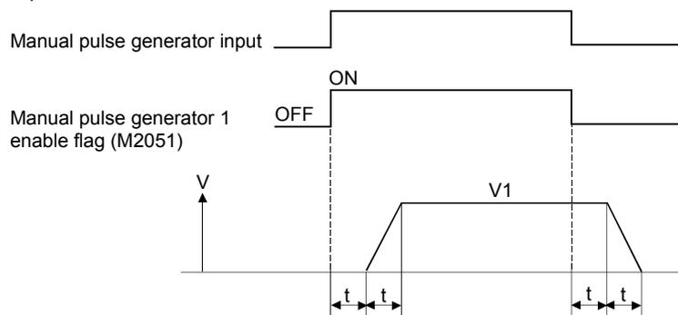
$$\text{Output speed (V1)} = [\text{Number of input pulses/ms}] \times [\text{Manual pulse generator 1- pulse input magnification setting}]$$
