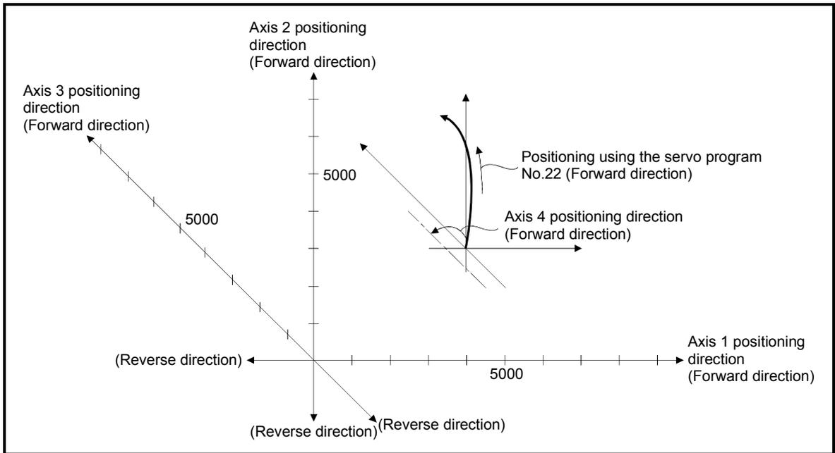
Fig.6.8 Positioning for 4 axes linear interpolation control
