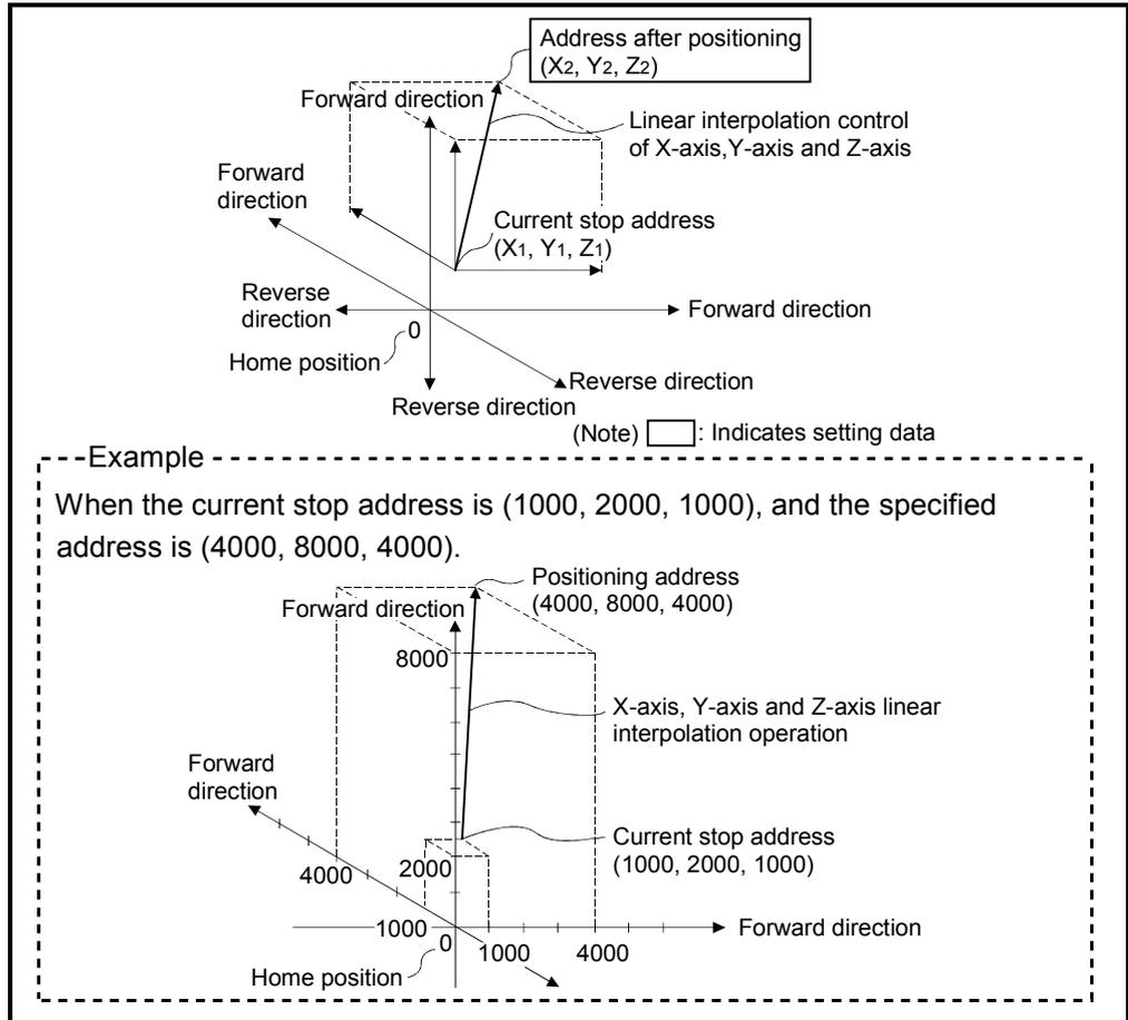
Fig.6.5 Positioning using absolute data method
