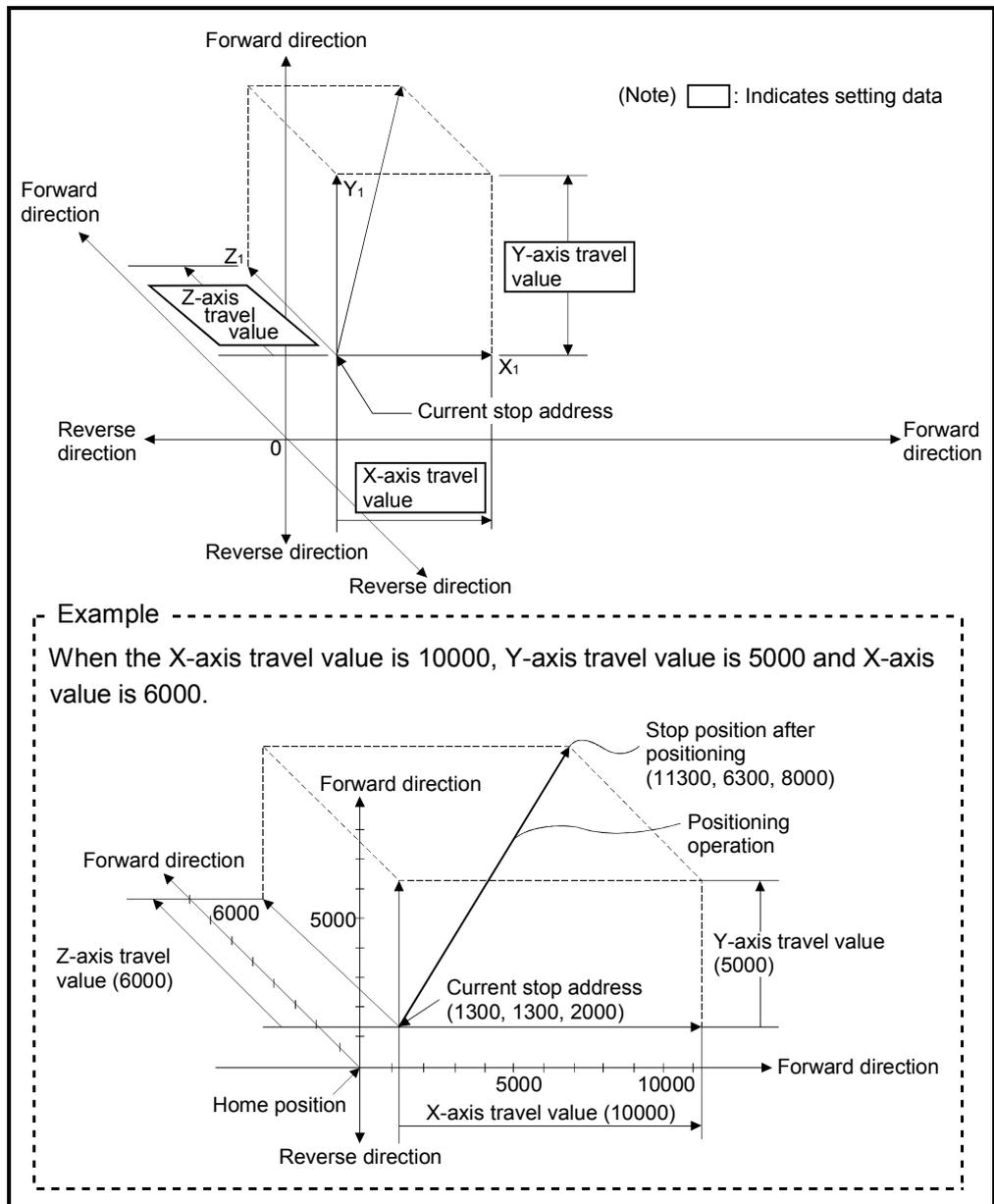
Fig.6.6 Positioning using incremental data method
