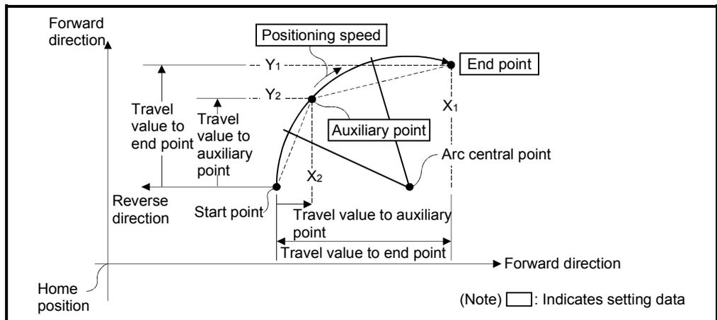
Fig.6.11 Circular interpolation control using incremental data method
