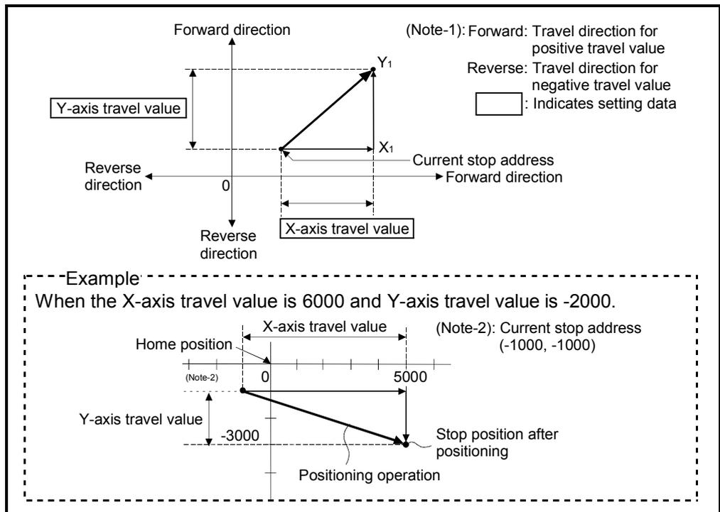
Fig.6.4 Positioning using incremental data method
