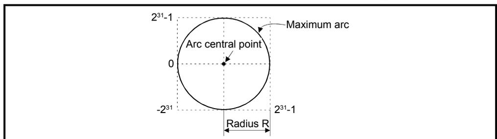
Fig.6.22 Maximum arc radius
