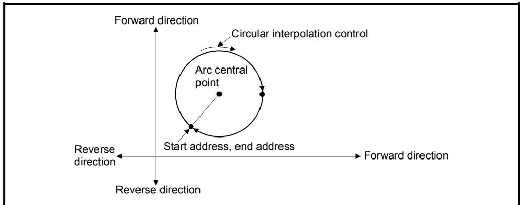
Fig.6.18 Positioning control of a complete round
