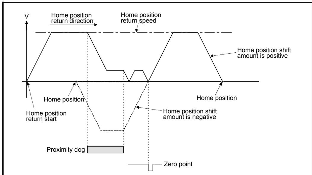
Fig. 6.48 Home position shift operation with the home position return speed
