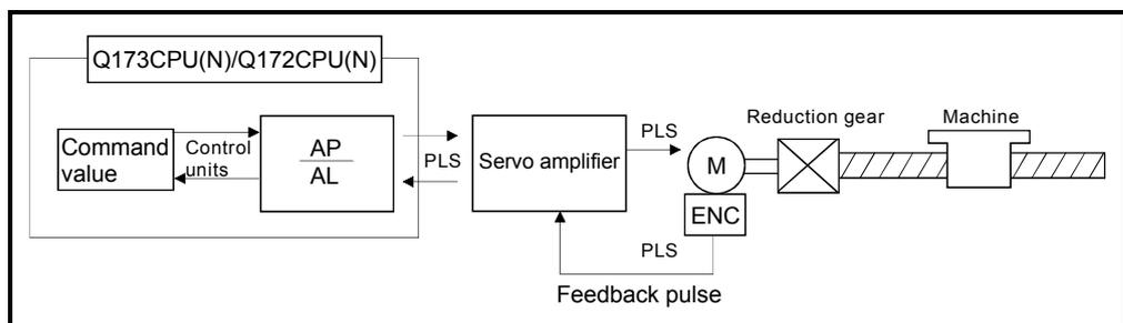
Fig. 4.1 Control content of the Motion CPU
