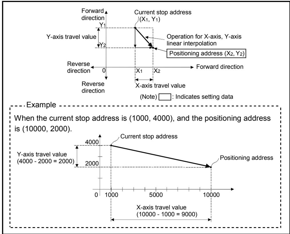
Fig.6.3 Positioning using absolute data method
