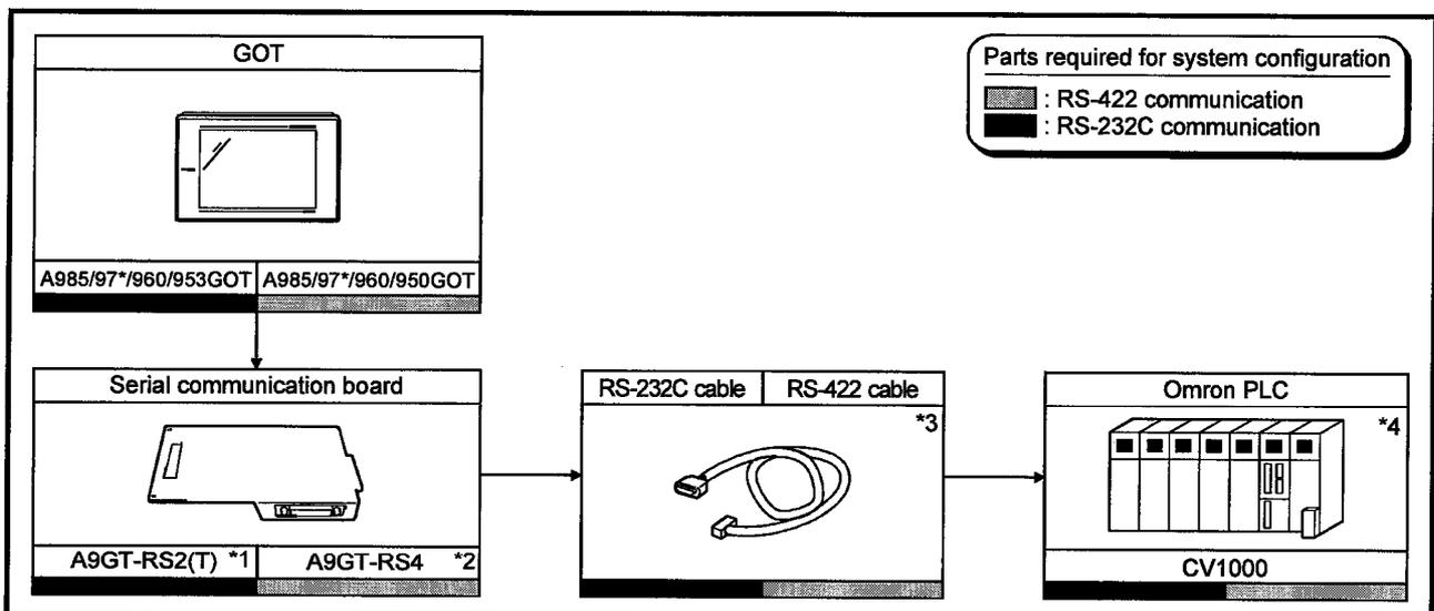
\*1 This is not required when the A953GOT (with built-in serial communication interface) is used.
