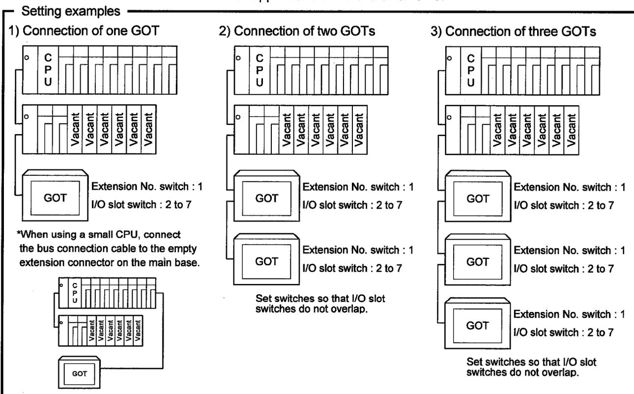
(3) Setting method used when there are no empty slots on the extension base unit connected
