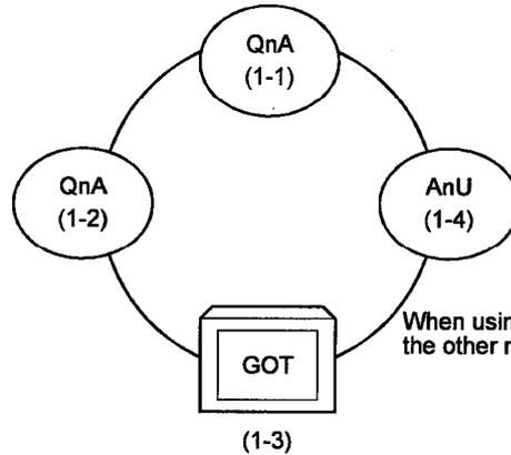
When using MELSECNET/10 connection, the other network cannot be monitored.
