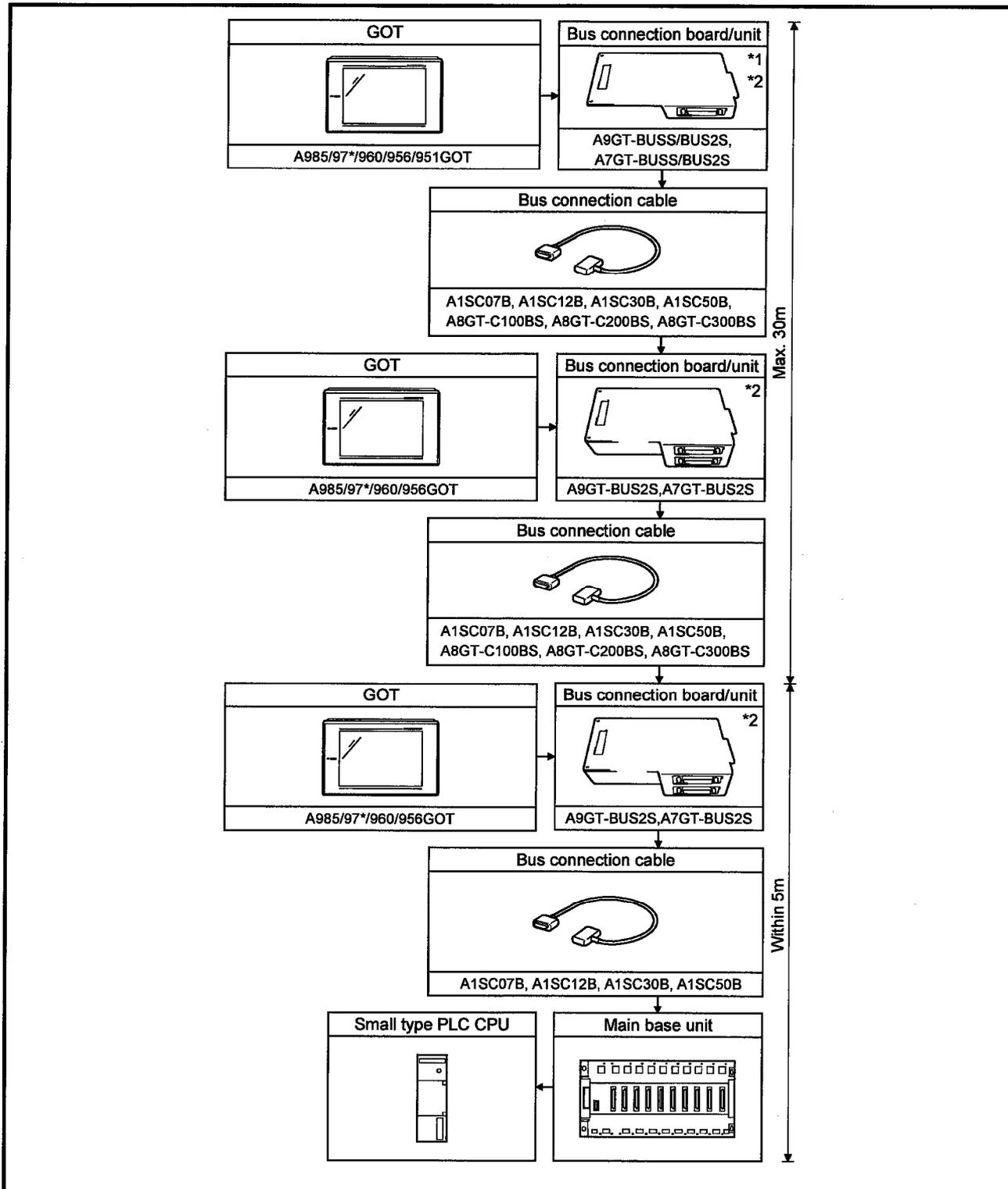
\*1 This is not required when the A951GOT (with built-in bus connection interface) is used.
