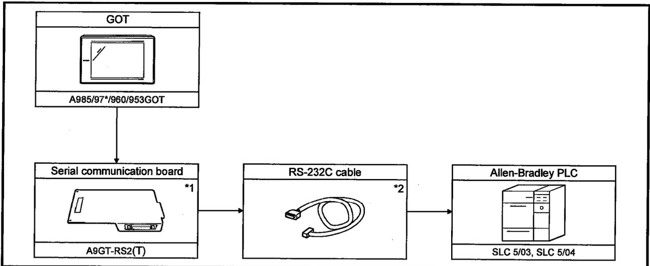
\*1 This is not required when the A953GOT (with built-in serial communication interface) is used.
