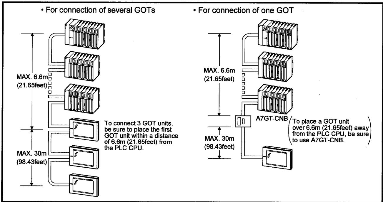
• Connection with small type PLC CPU
