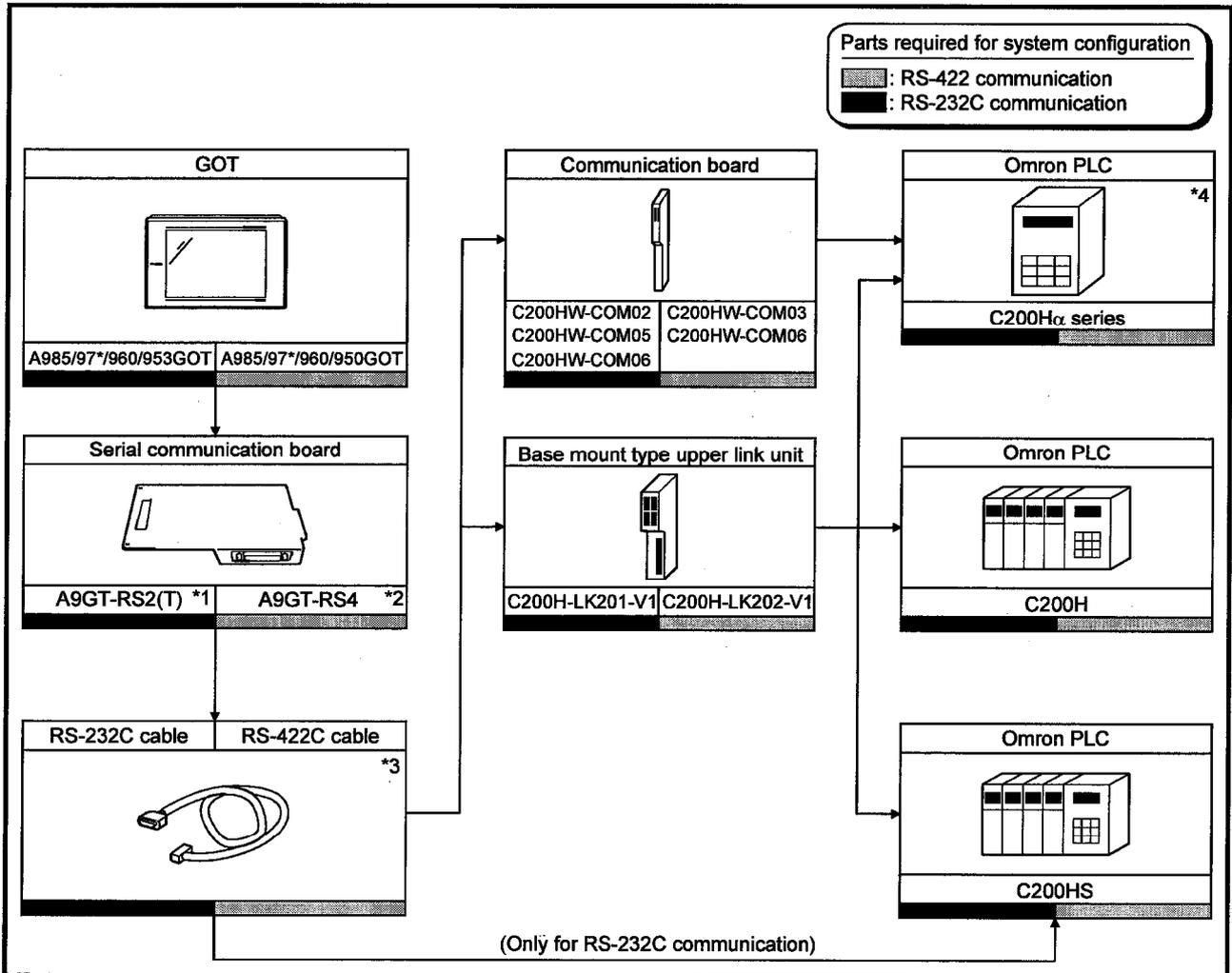
\*1 This is not required when the A953GOT (with built-in serial communication interface) is used.
