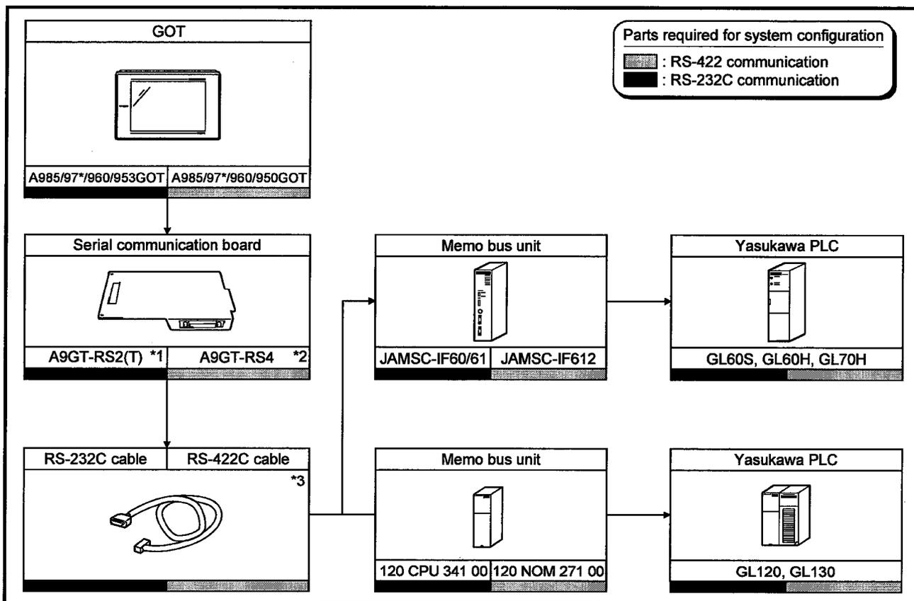
\*1 This is not required when the A953GOT (with built-in serial communication interface) is used.
