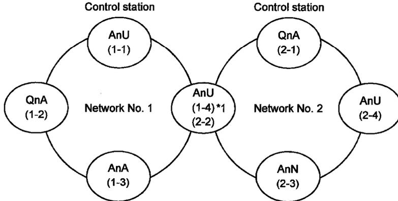
\*1 Data link parameter "Effective unit number for accessing other stations" is designated to the unit number that is connected to the network No. 1.
