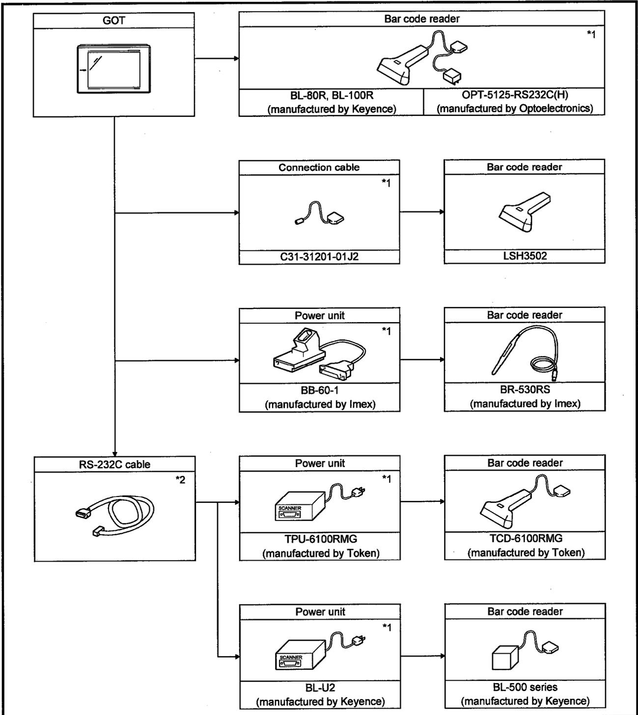
\*1 The bar code reader requires power (DC5V) from the AC-DC adapter and the corresponding power unit.
