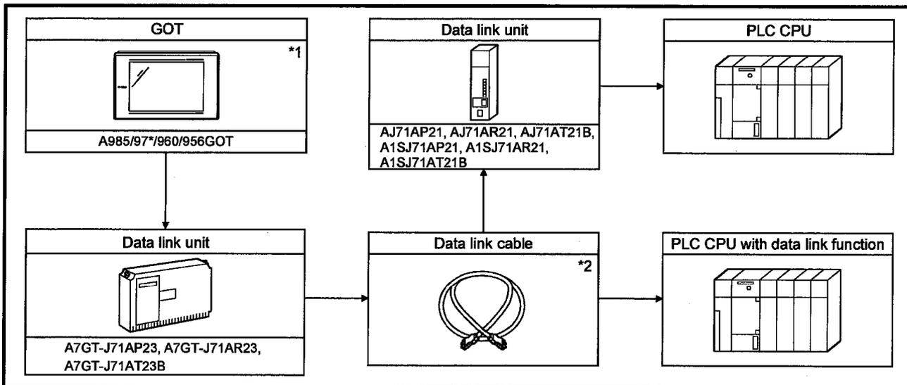
\*1 The maximum number of GOT units that allow connection is the number of stations in each data link system that allow connection.
