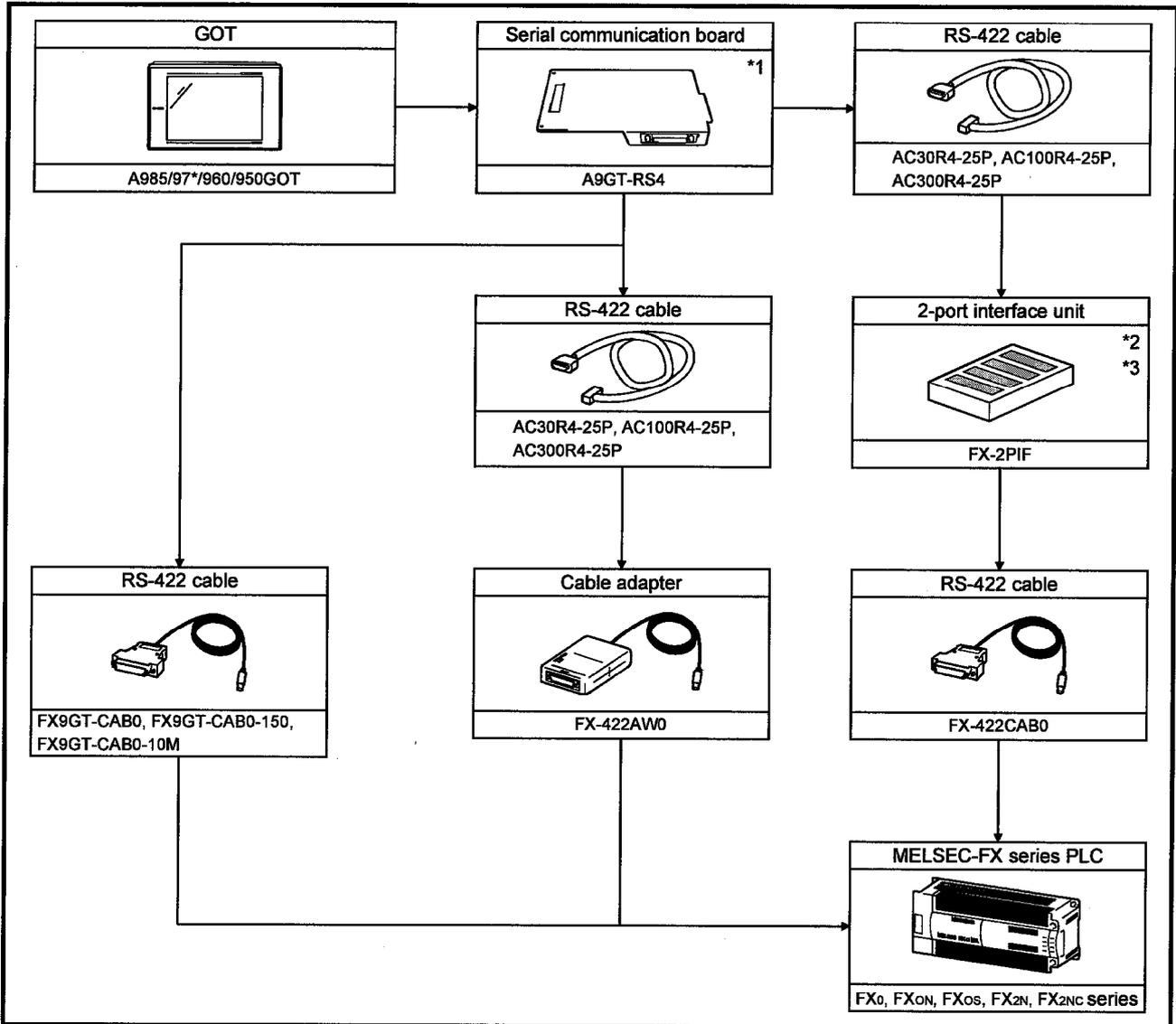
\*1 This is not required when the A950GOT (with built-in serial communication interface) is used.
