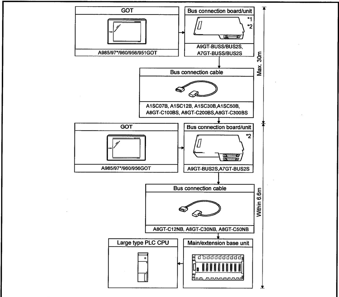
\*1 This is not required when the A951GOT (with built-in bus connection interface) is used.
