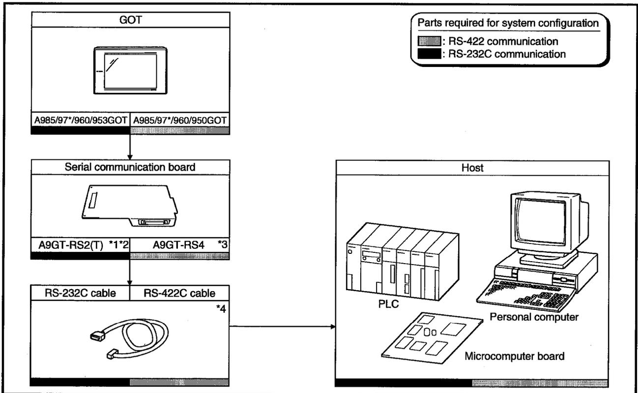
\*1 This is not required when the A953GOT (with built-in serial communication interface) is used.
