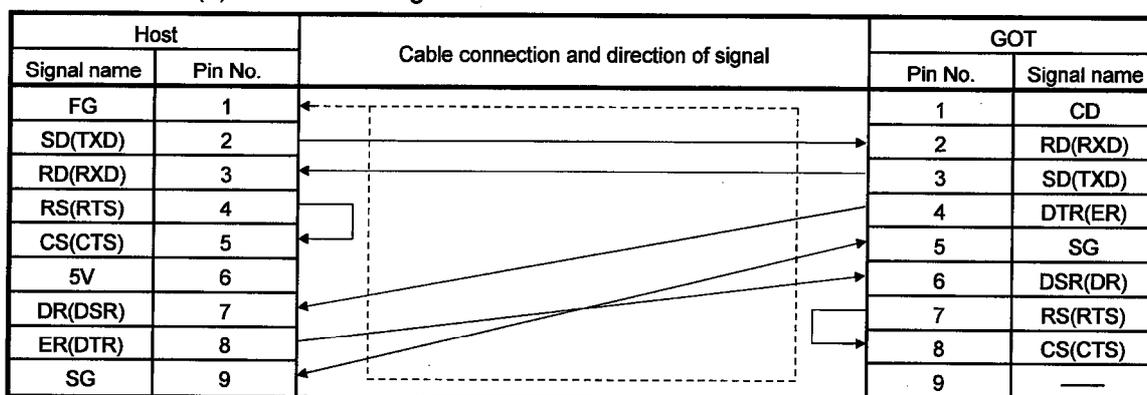
Note) The pin numbers for the host in the above diagram are for reference.
