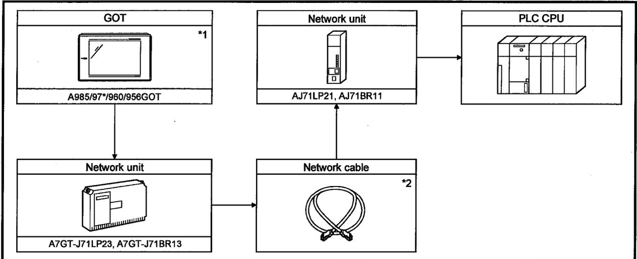
\*1 The maximum number of GOT units that allow connection is the number of stations in each data link system that allow connection.
