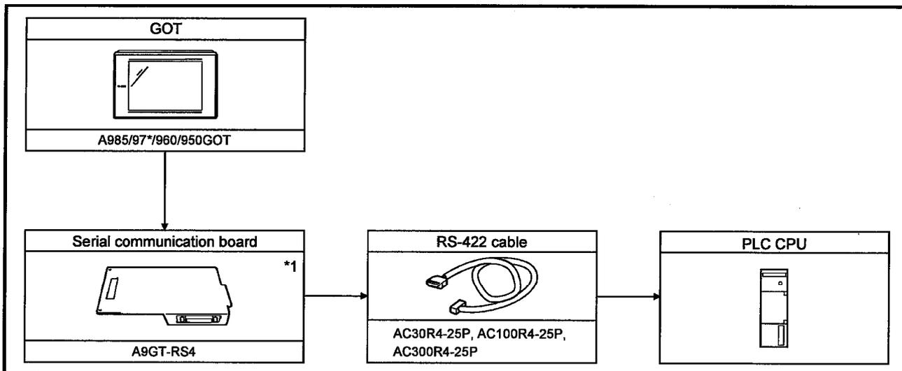
\*1 This is not required when the A950GOT (with built-in serial communication interface) is used.
