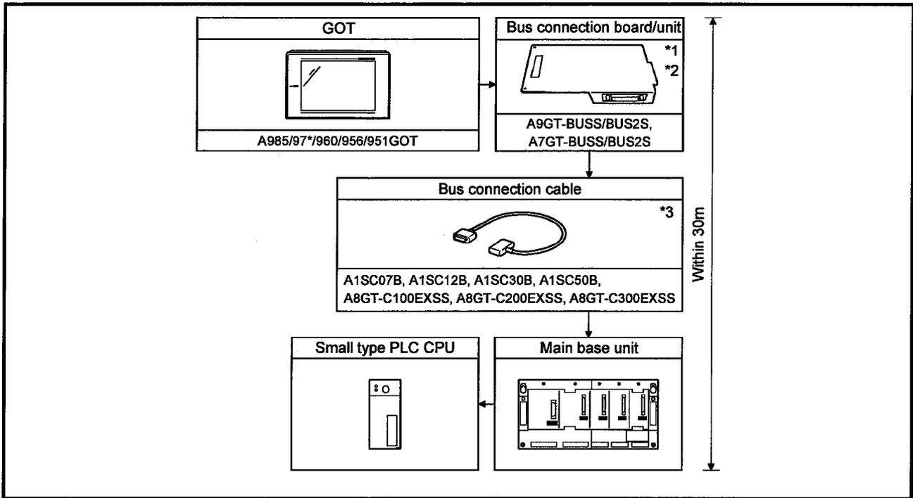
\*1 This is not required when the A951GOT (with built-in bus connection interface) is used.
