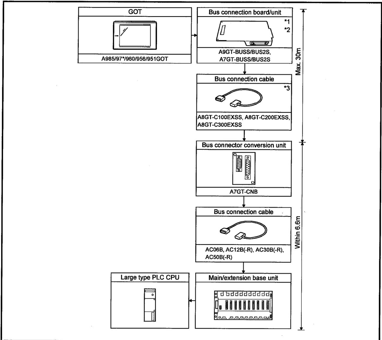
\*1 This is not required when the A951GOT (with built-in bus connection interface) is used.
