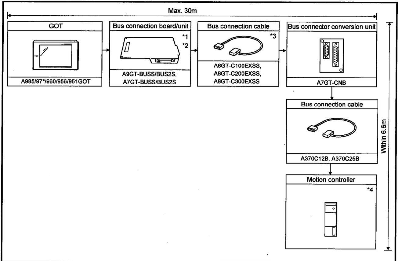
\*1 This is not required when the A951GOT (with built-in bus connection interface) is used.
