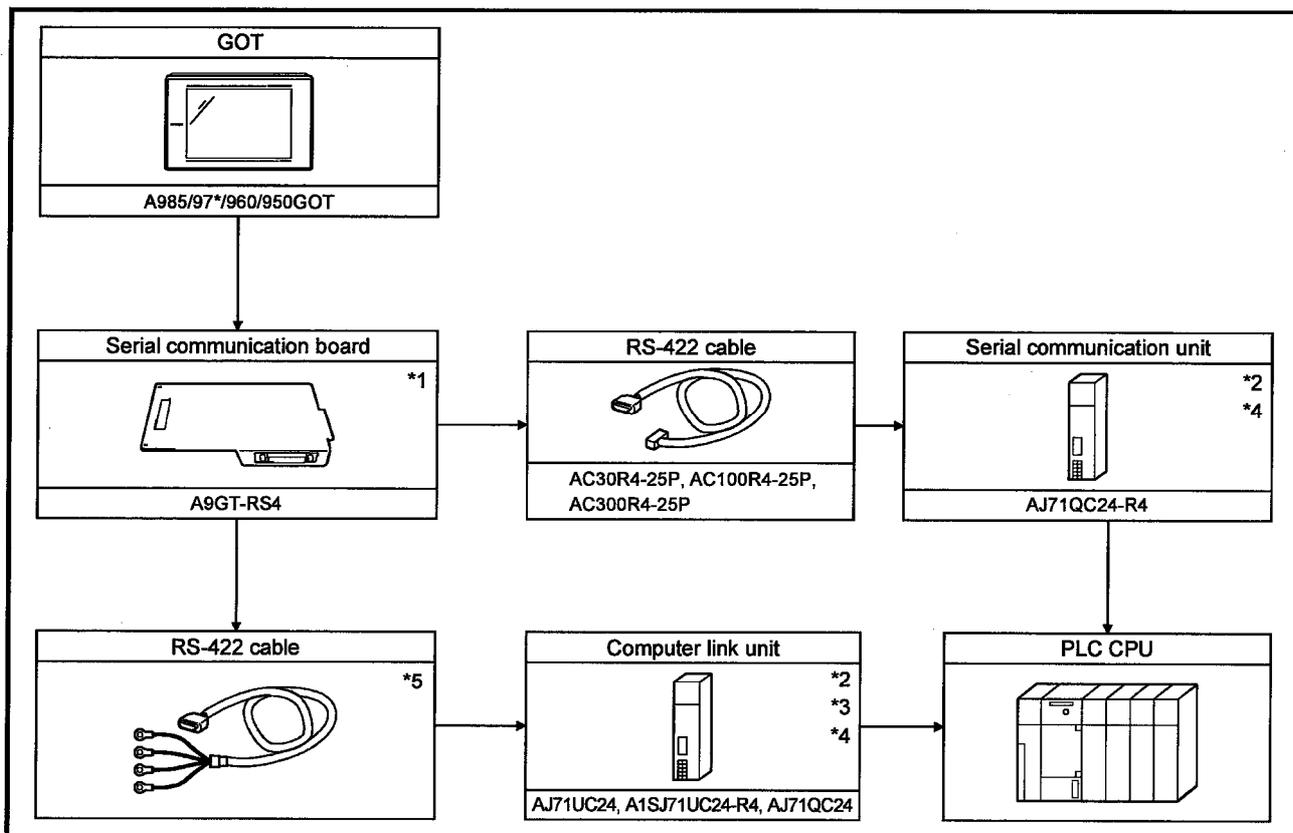
\*1 This is not required when the A950GOT (with built-in serial communication interface) is used.
